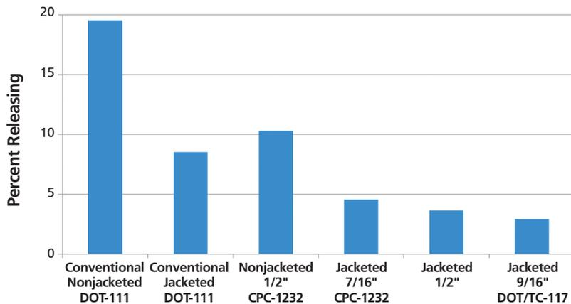
**FIGURE 2** Percentage of tank cars of various designs expected to release 100 or more gallons (CPR<sub>100</sub>) from physical impacts in FRA-reportable accidents (4).
