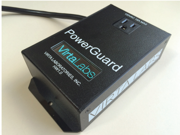
FIGURE 2 My former students and I cofounded Virta Labs, Inc. to detect malware and anomalies on medical devices using a smart power outlet rather than installed software. Machine learning and side channels in reactive AC power enable detection in a manner that does not cause alarm fatigue (Clark et al. 2013).
