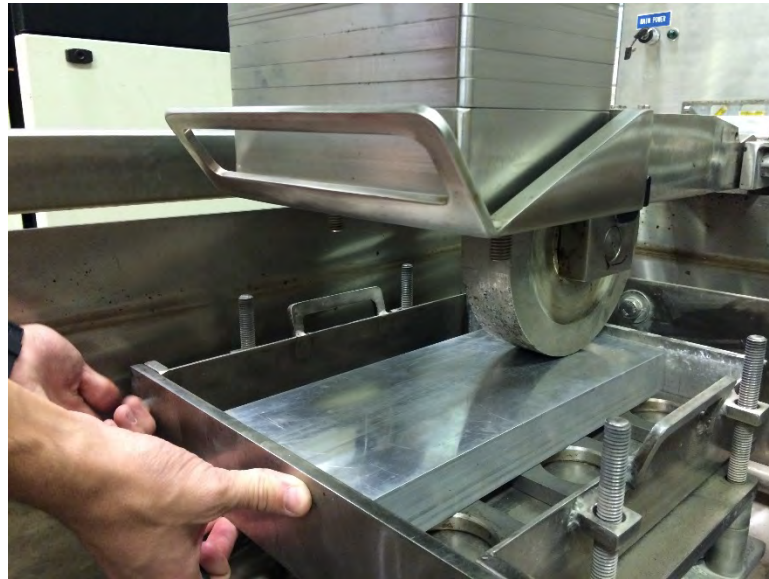
(a) Flat surface for obtaining zero readings
