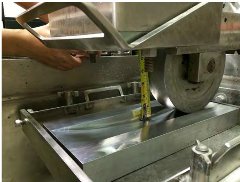
Figure 34 Metal specimen for verifying locations of deformation readings
