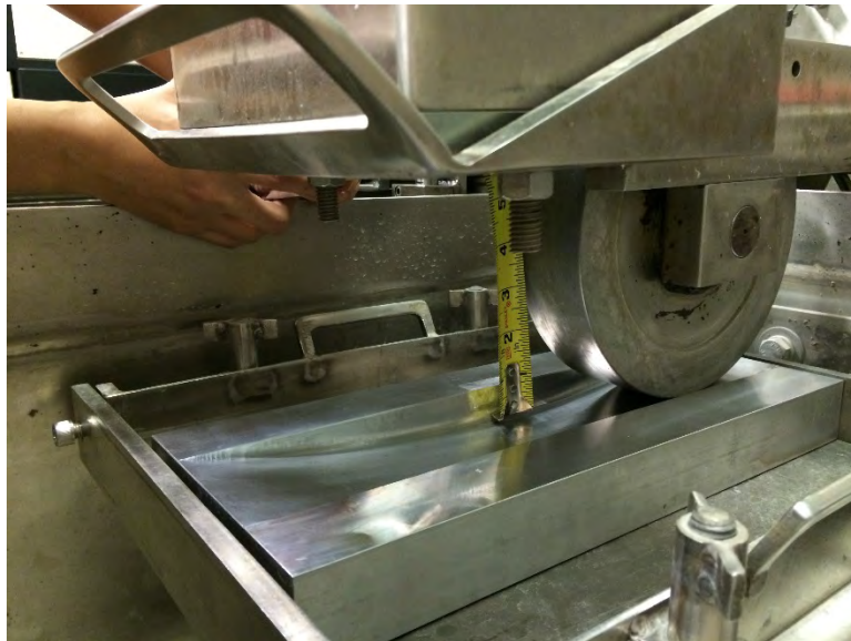
(b) Recording deformation readings along the curvature (ruler shown for scale)
