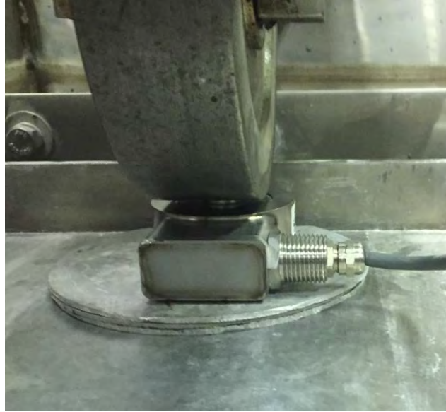
Figure 10 Measuring details: The process of using load cell (Vendor A)
