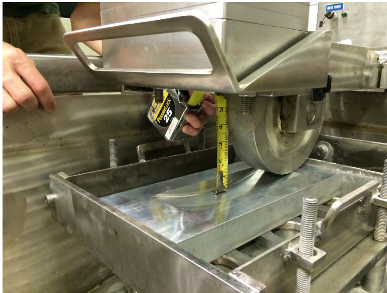
Figure 4 Metal specimen for verifying locations of deformation readings
