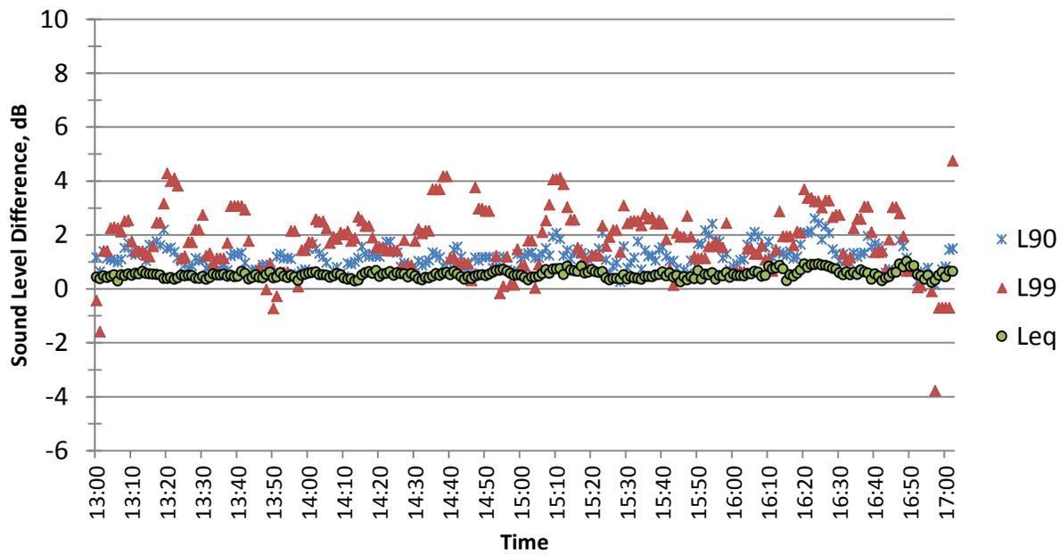
Figure 58. Differences in A-weighted 5-min  $L_{90}$ ,  $L_{99}$  and  $L_{eq}$ , I-90, BarCom04 and NoBarCom06.
