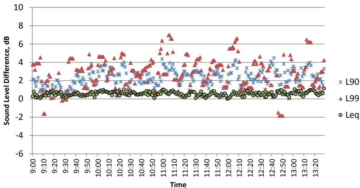
**Figure 37. Differences in broadband A-weighted 5-min  $L_{90}$ ,  $L_{99}$  and  $L_{eq}$ , SR-71, BarRef01 and NoBarRef02.**
