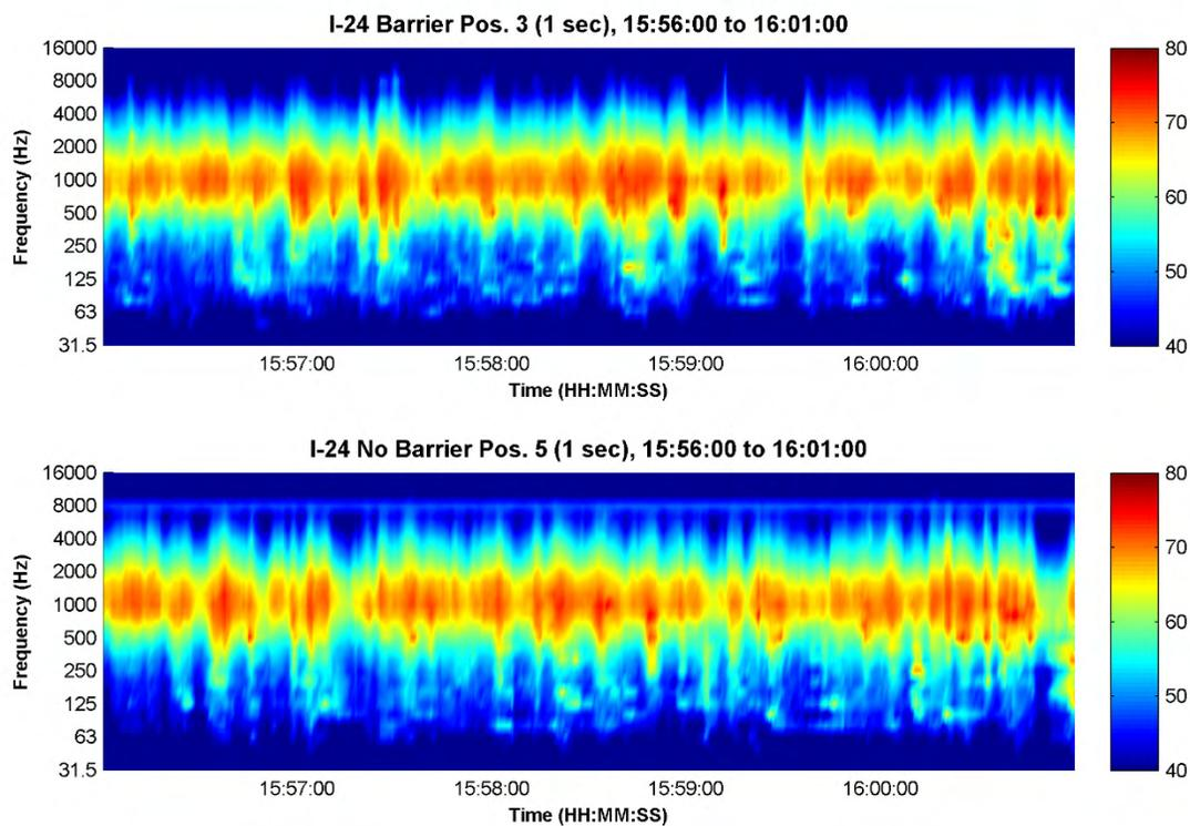
**Figure 41. I-24 5-minute spectrograms; top to bottom: lows mics BarCom03 and NoBarCom05; for Calm Lapse group CLG-6-1, start time 15:56.**
