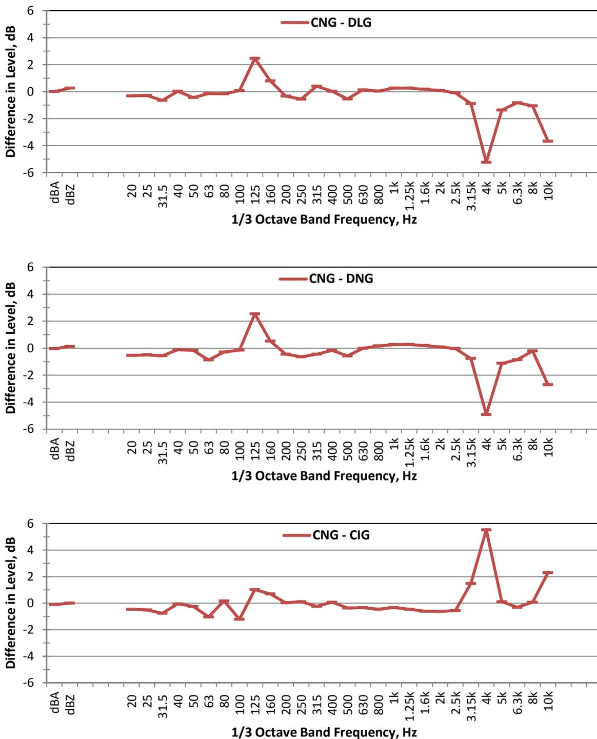
Figure 71. Differences in the Calm Neutral average differences and Downwind Lapse, Downwind Neutral and Calm Inversion average differences ( $L_{eq}(5min)$ , BarCom04 minus NoBarCom06, MD-5.
