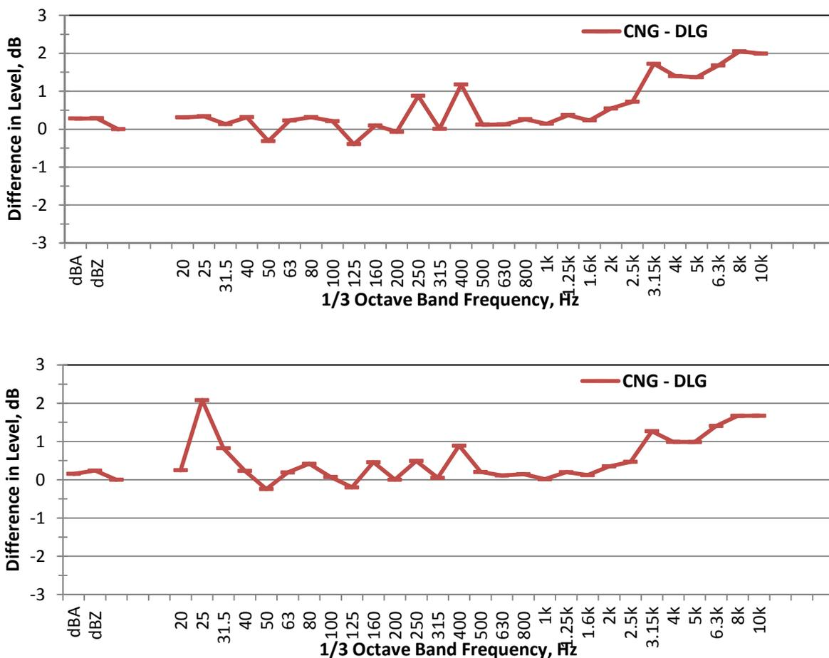
**Figure 68. Calm Neutral minus the Downwind Lapse average differences ( $L_{eq}(5min)$ , BarCom03 minus NoBarCom05 (top) and BarCom04 minus NoBarCom06 (bottom), I-90.**
