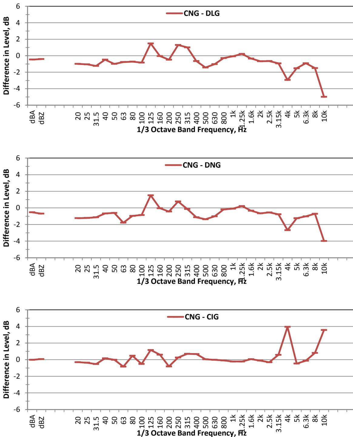
Figure 70. Calm Neutral average differences minus Downwind Lapse, Downwind Neutral and Calm Inversion average differences ( $L_{eq}(5min)$ , NoBarCom05 minus NoBarCom05, MD-5).
