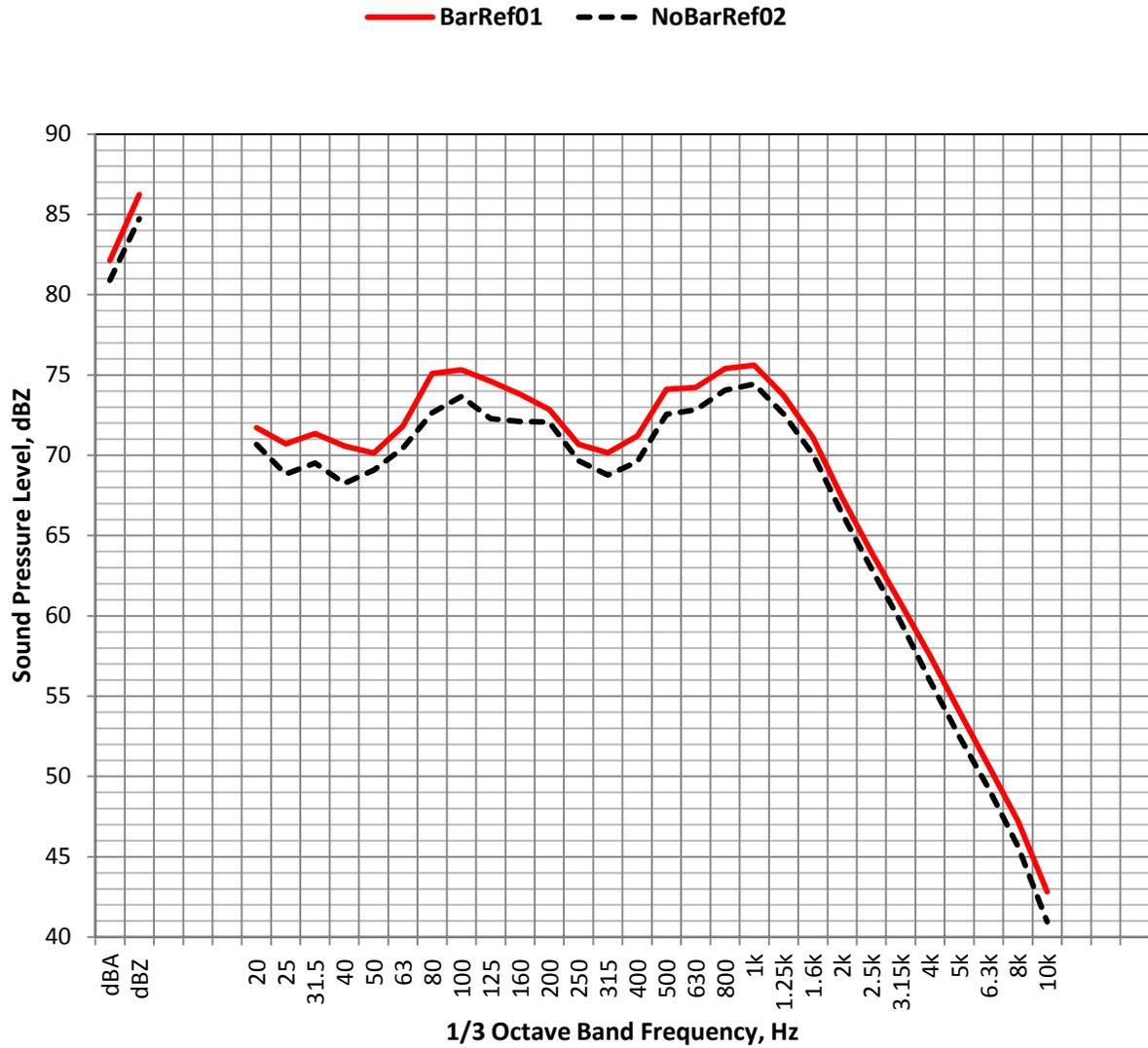
**Figure 31. Sample sound pressure level spectra for BarRef01 and NoBarRef02, I-24, Upwind Lapse group ULG-3-2, 13:26-13:31 ( $L_{eq}(5min)$ , dBZ).**
