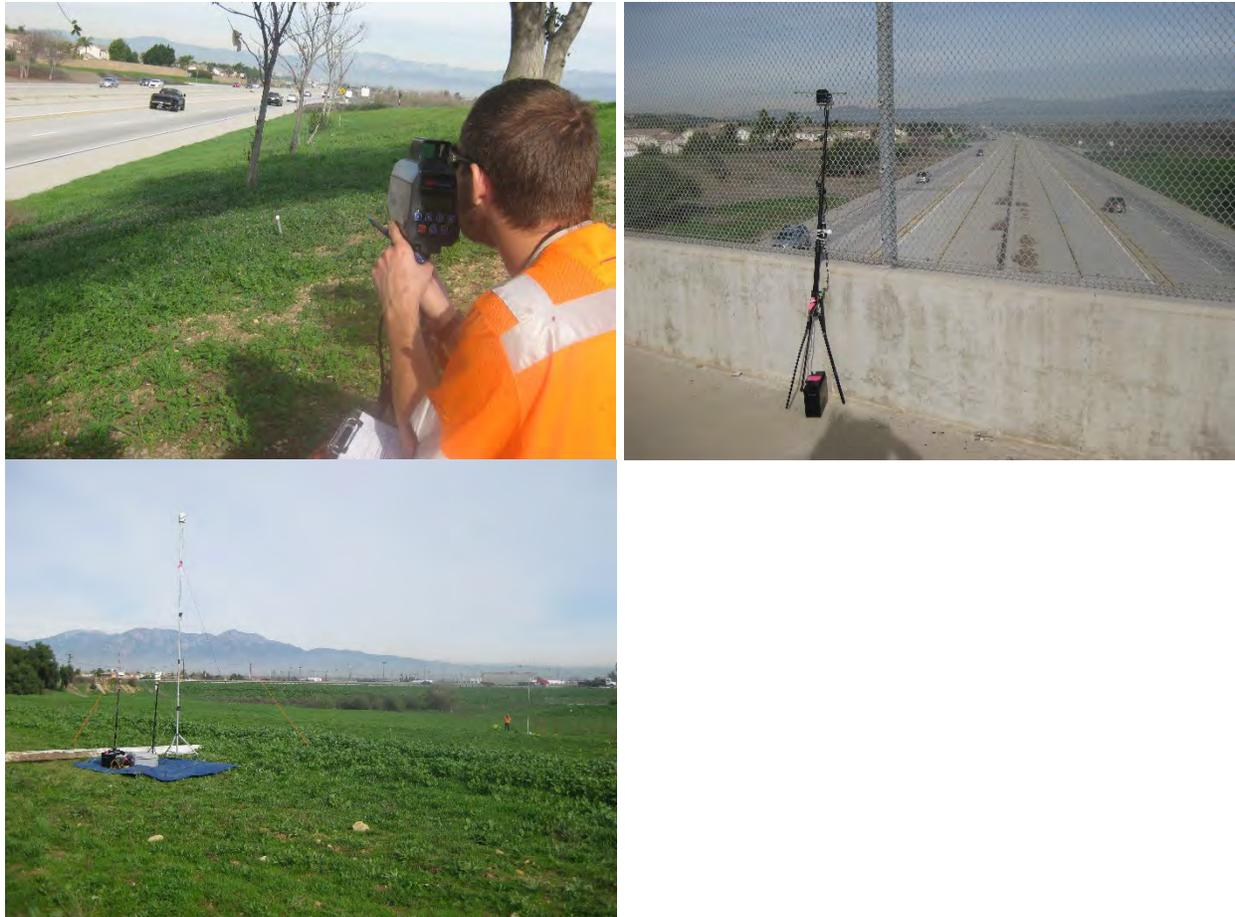
**Figure 19. SR-71 BarRef01 Traffic speed (top left), traffic count video (top right), meteorological station (bottom left). (Source: research team members.)**
