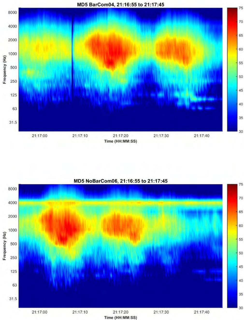
**Figure 185. MD-5 spectrograms for heavy truck on northbound (community) side (approximate event times: Barrier site 21:17:20, No Barrier site 21:17:05.) Additional vehicle follows the heavy truck: top is BarCom04; bottom is NoBarCom06.**
