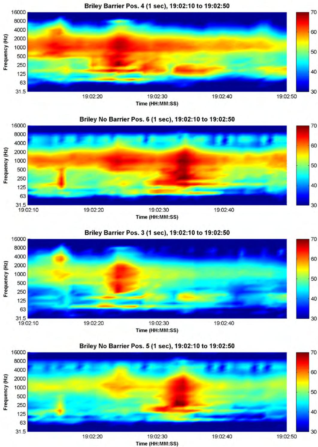
Figure 70. Spectrogram for a heavy truck eastbound (example 2); top to bottom: high mics (BarCom04 and NoBarCom06), low mics (BarCom03 and NoBarCom05); Briley.
