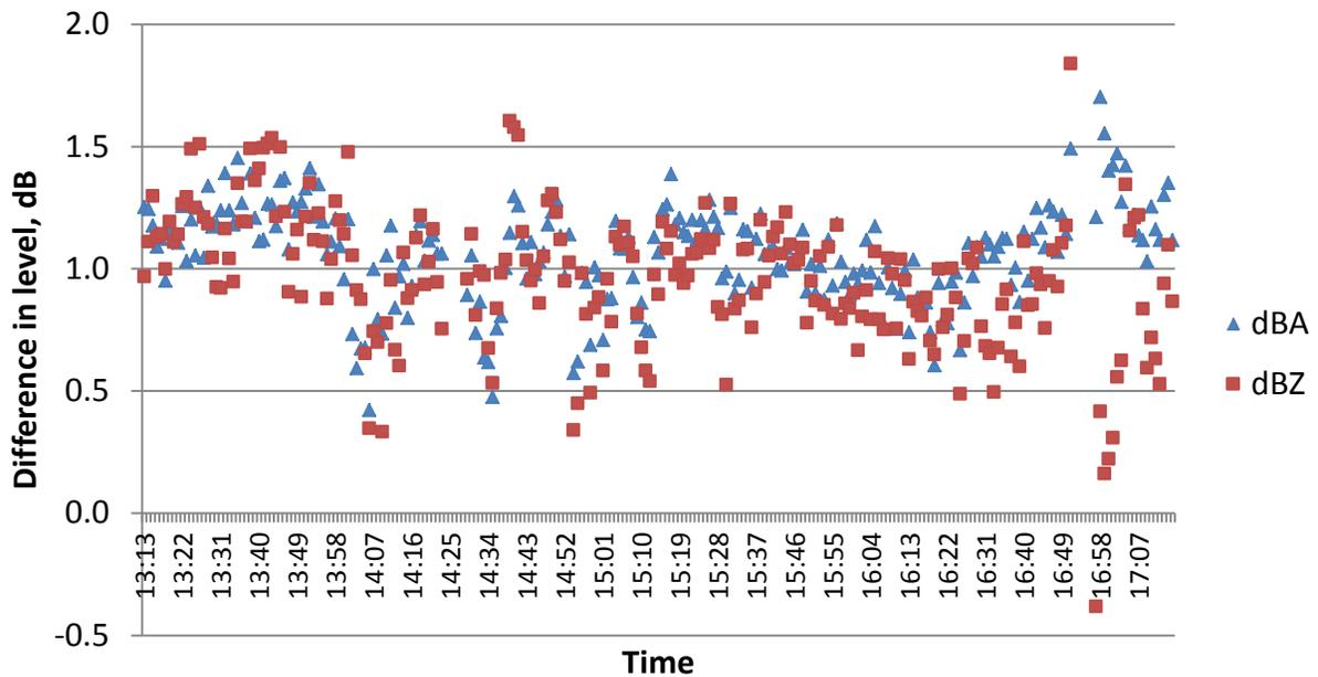
Figure 11. Differences in running  $L_{eq}(5min)$ , I-24, BarRef01 minus NoBarRef02.
