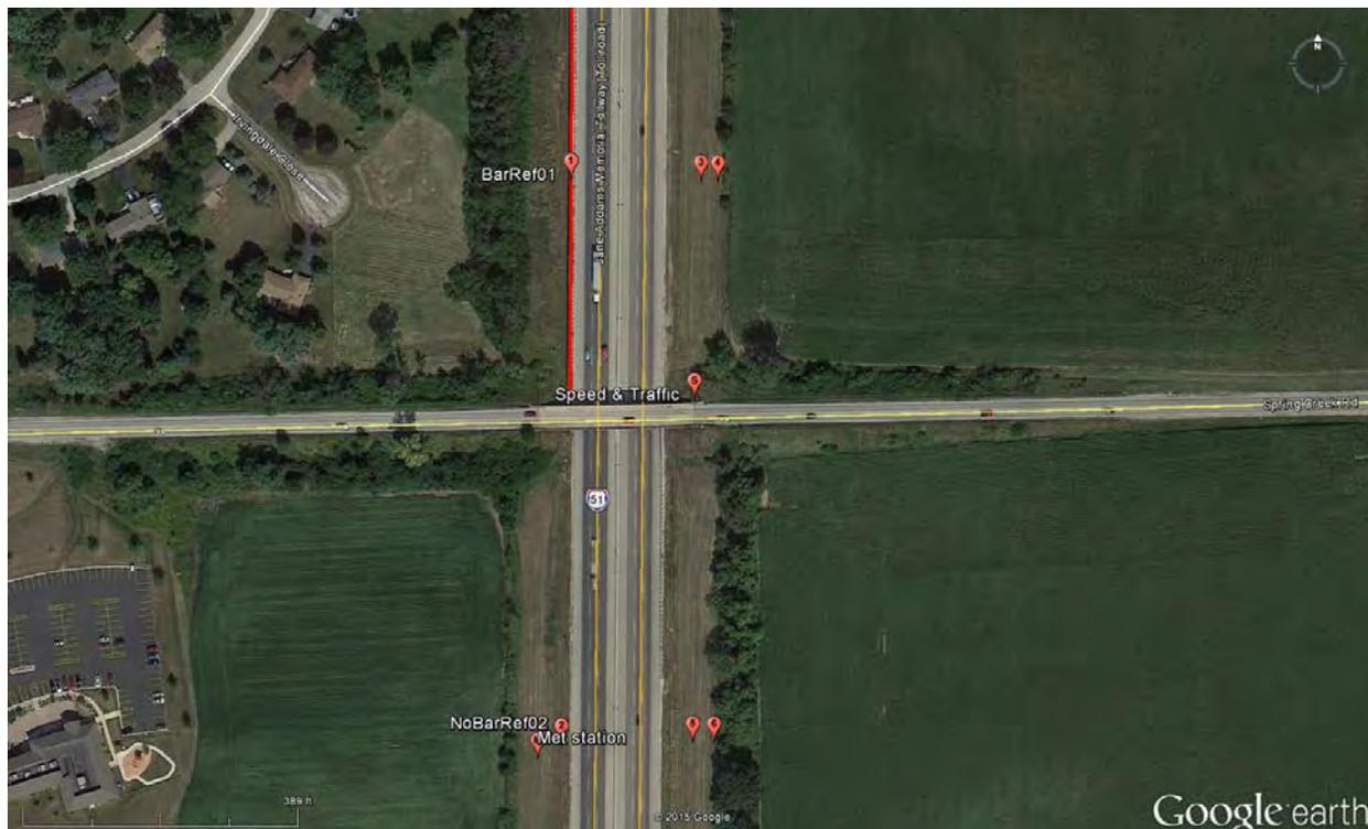
Figure 71. I-90 microphone positions. (Source: Google Earth).
