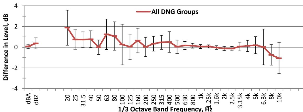
**Figure 44. Averages of the differences in  $L_{eq}(5min)$  +/- one standard deviation (dB), all microphones, for all Downwind Neutral groups, MD-5.**
