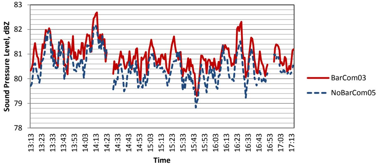
Figure 12. Running  $L_{eq}(5min)$ , I-24, unweighted sound pressure level, dBZ, BarCom03 and NoBarCom05.
