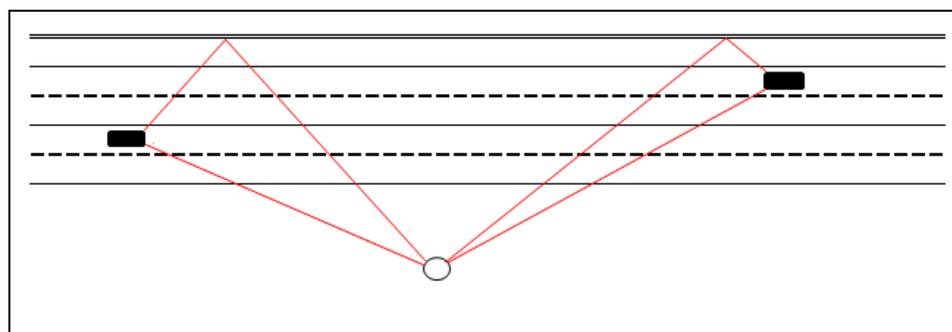
**Figure 1. Plan view of the relationship between direct and reflected sound paths to a receptor across the highway from a noise barrier.**
