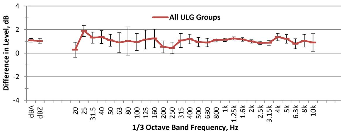
Figure 33. Averages of the differences in  $L_{eq}(5min)$  +/- one standard deviation (dB), BarRef01 minus NoBarRef02, for all Upwind Lapse groups, I-24.
