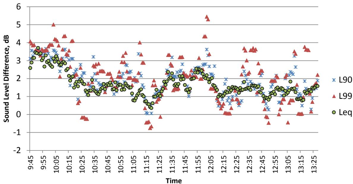
**Figure 64. Differences in broadband A-weighted 5-min  $L_{90}$ ,  $L_{99}$  and  $L_{eq}$ , SR-71, BarCom04 and NoBarCom06.**
