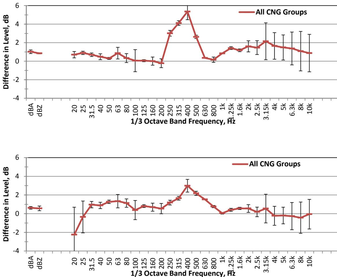
**Figure 67. Averages of the differences in  $L_{eq}(5min)$  +/- one standard deviation (dB), BarCom03, BarCom04, NoBarCom05 and NoBarCom06, for all Calm Neutral groups, I-90.**
