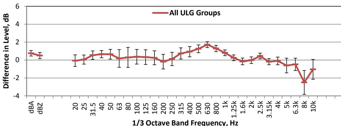
**Figure 53. Averages of the differences in  $L_{eq}(5min)$  +/- one standard deviation (dB), BarCom03 minus NoBarCom05, for all Upwind Lapse groups, I-24.**
