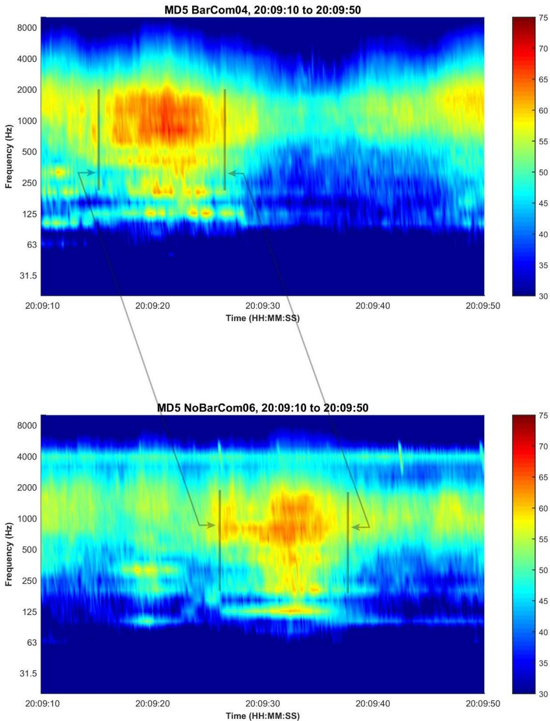
**Figure 73. MD-5 spectrograms for a pickup truck on southbound (barrier) side (approximate event times: Barrier site 20:09:20, No Barrier site 20:09:35). Additional vehicle follows the heavy truck. Top is BarCom04; bottom is NoBarCom06.**
