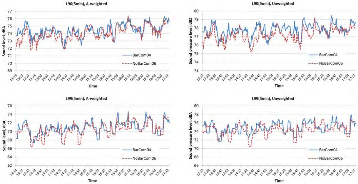
Figure 32.  $L_{90}(5min)$  and  $L_{99}(5min)$ , I-24, BarCom04 and NoBarCom06 – broadband A-weighted sound level (left) and sound pressure level (right)
