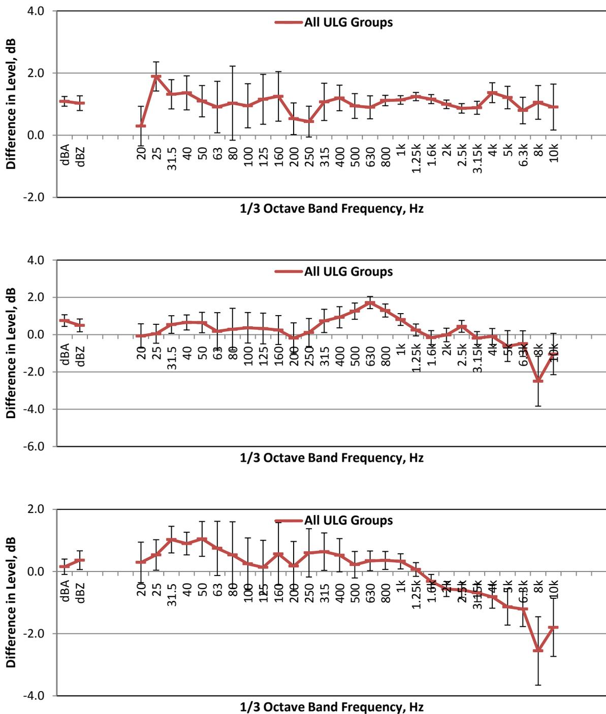
Figure 24. Averages of the differences in  $L_{eq}(5min)$  +/- one standard deviation (dB), all microphones, for all Upwind Lapse groups, I-24.
