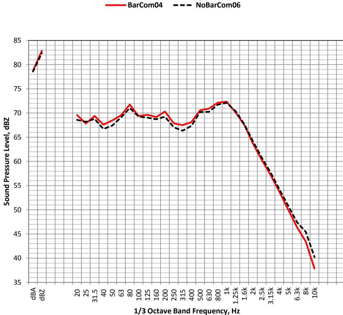
**Figure 23. Sample sound pressure level spectra for BarCom04 and NoBarCom06, I-24, Upwind Lapse group ULG-3-2, 13:26-13:31 ( $L_{eq}(5min)$ , dBZ).**
