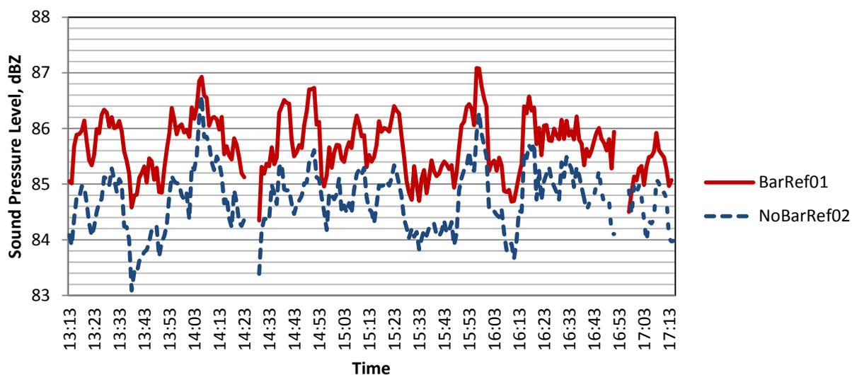
**Figure 9. Running  $L_{eq}(5min)$ , I-24, unweighted sound pressure level, dBZ, BarRef01 and NoBarRef02.**
