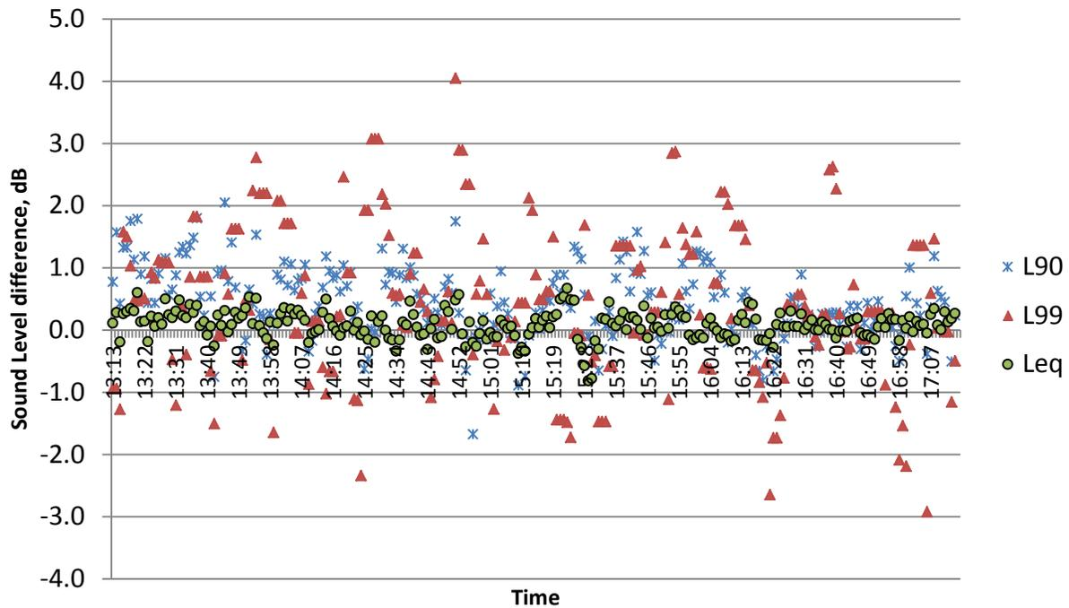
Figure 33. Differences in broadband A-weighted 5-min  $L_{90}$ ,  $L_{99}$  and  $L_{eq}$ , I-24, BarCom04 and NoBarCom06
