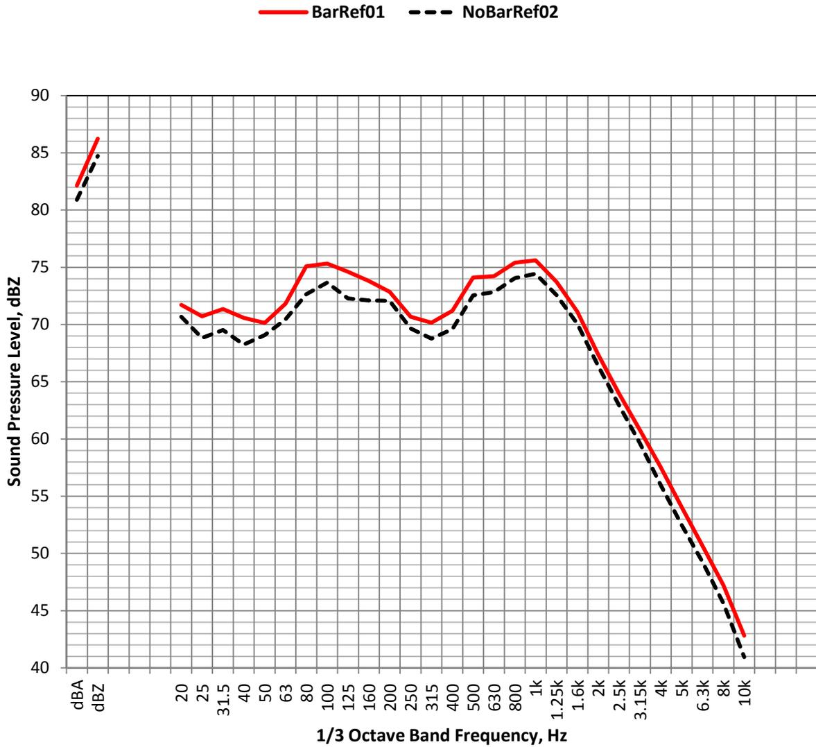
**Figure 21. Sample sound pressure level spectra for BarRef01 and NoBarRef02, I-24, Upwind Lapse group ULG-3-2, 13:26-13:31 ( $L_{eq}(5min)$ , dBZ).**
