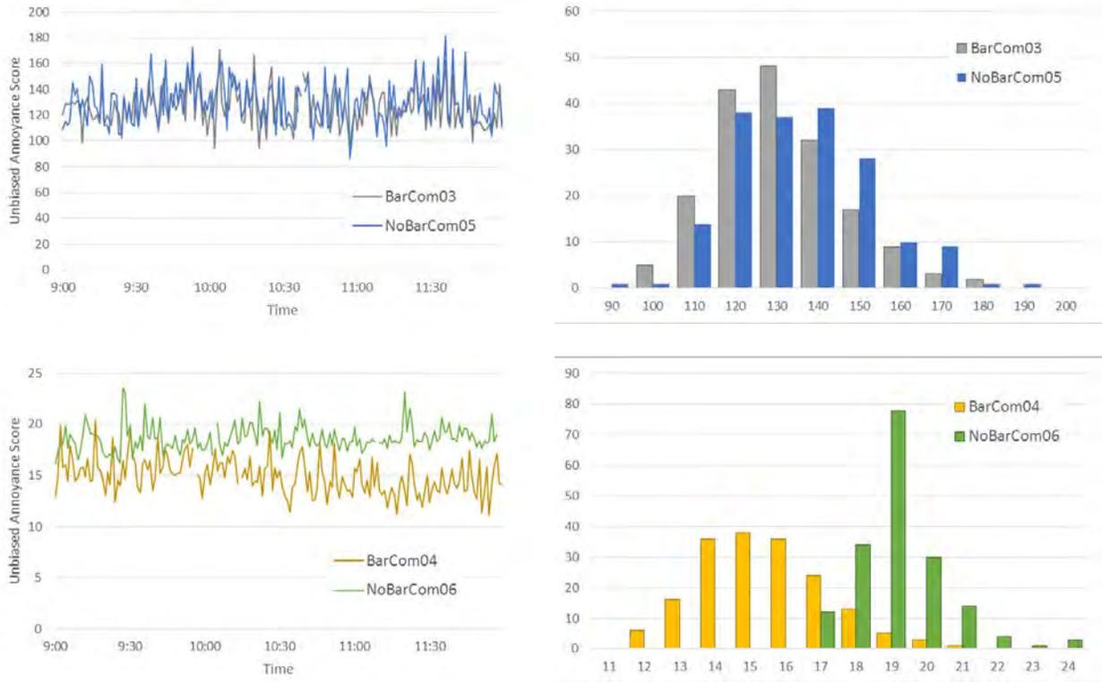
**Figure 79. Comparing UBA computed for lower community microphones, close to the roadway, with upper community microphones, distant from the roadway, at CA SR-71.**
