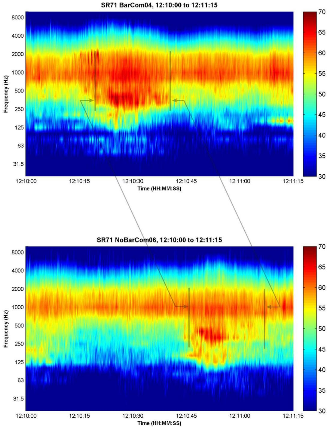
**Figure 72. SR-71 spectrograms for motorcycle on southbound (community) side (approximate event times): Barrier site 12:10:25, No Barrier site 12:10:50. Top is BarCom04; bottom is NoBarCom06.**
