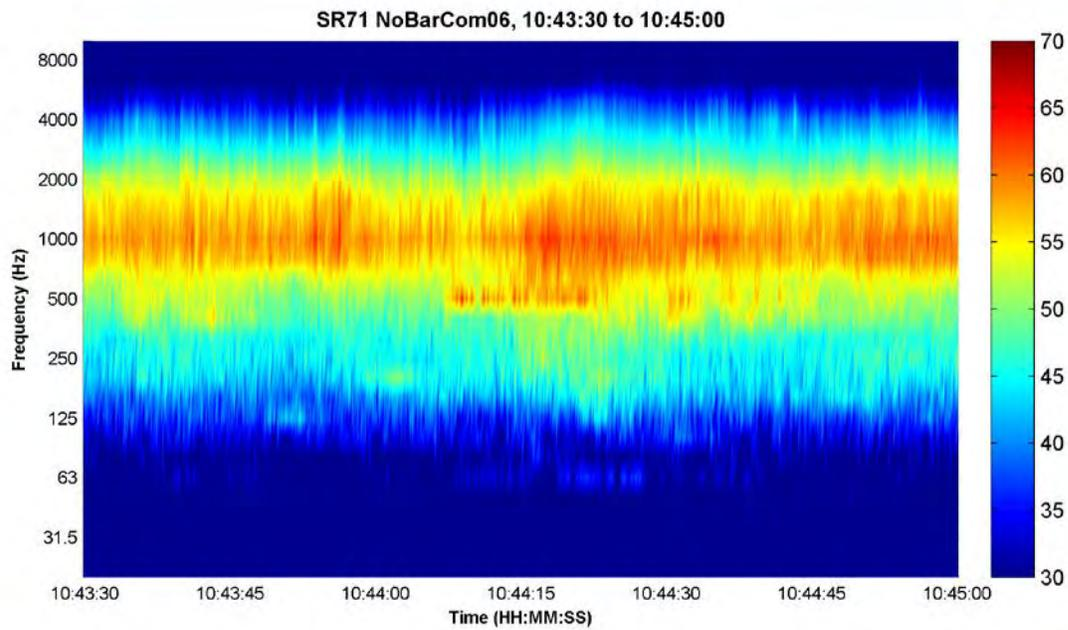
Figure 134. SR-71 spectrograms for heavy trucks on southbound (community) side: top is BarCom04; bottom is NoBarCom06.
