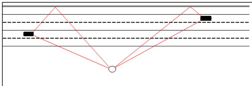
**Figure 1. Plan view of the relationship between direct and reflected sound paths to a receptor across the highway from a noise barrier.**
