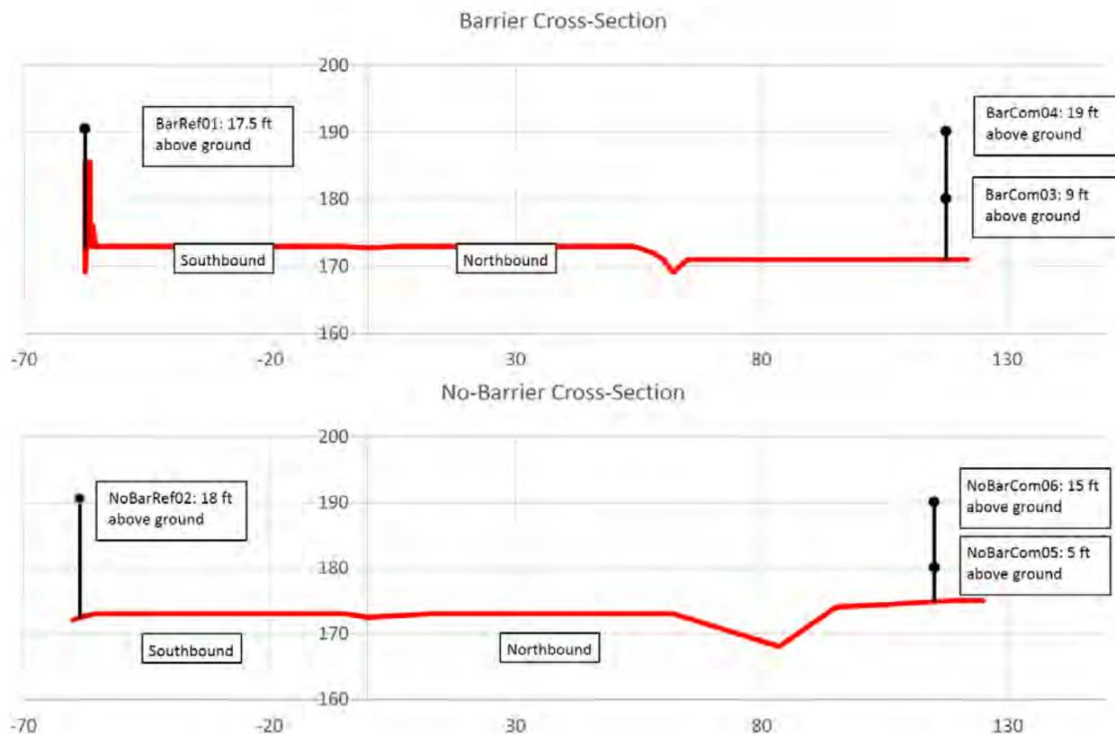
**Figure 143. Cross-sections at the MD-5 Barrier (top) and No Barrier (bottom) sites.**
