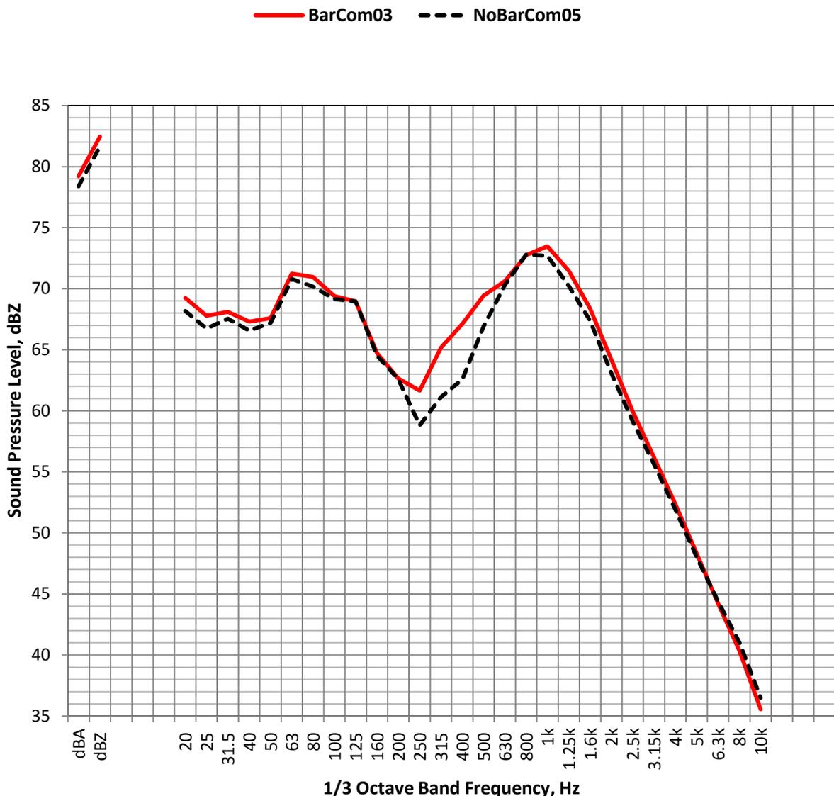
**Figure 52. Sample sound pressure level spectra for BarCom03 and NoBarCom05, I-90, Calm Neutral class, CNG-1-1, Period 15:37 ( $L_{eq}(5min)$ , dBZ).**
