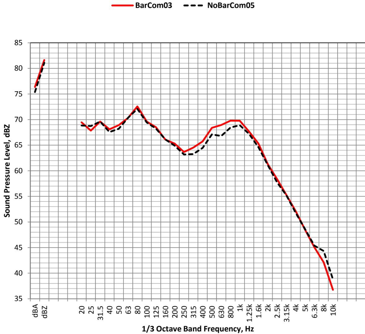
Figure 22. Sample sound pressure level spectra for BarCom03 and NoBarCom05, I-24, Upwind Lapse group ULG-3-2, 13:26-13:31 ( $L_{eq}(5min)$ , dBZ).
