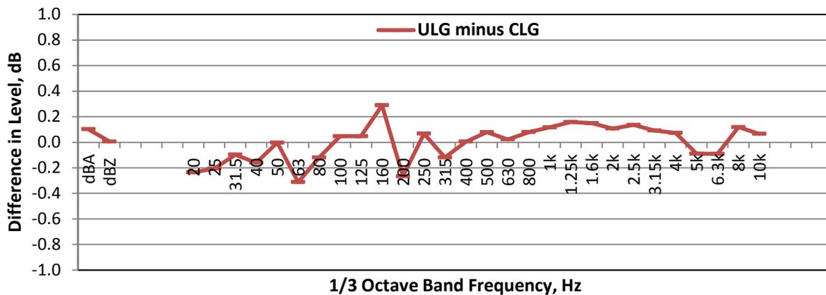
Figure 27. Differences in the Upwind Lapse average differences and the Calm Lapse average differences ( $L_{eq}(5min)$  +/- one standard deviation, dB), all microphones, I-24.
