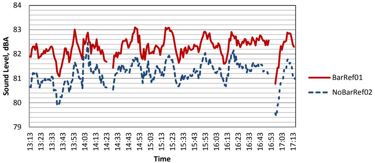
Figure 10. Running  $L_{eq}(5min)$ , I-24, A-weighted sound level, dBA, BarRef01 and NoBarRef02.
