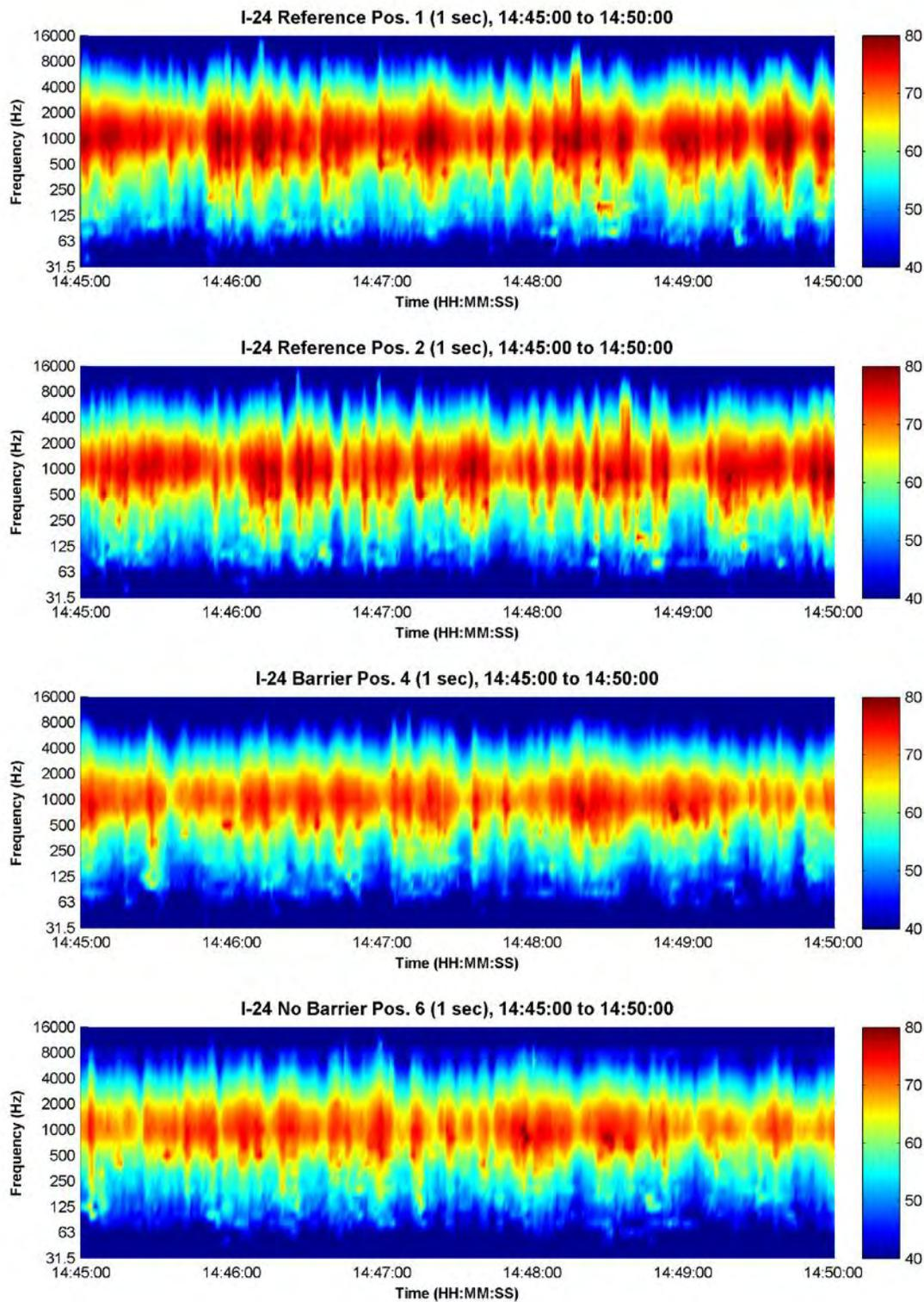
**Figure 38. I-24 5-minute spectrograms; top to bottom: BarRef01, NoBarRef02, and high mics (BarCom04 and NoBarCom06); for Upwind Lapse group ULG-9-1, start time 14:45.**
