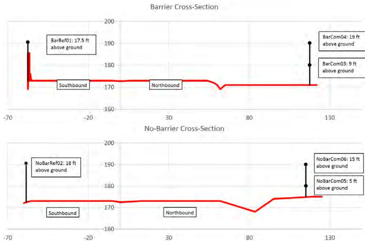
Figure 22. Cross-sections at the MD-5 Barrier (top) and No Barrier (bottom) sites.
