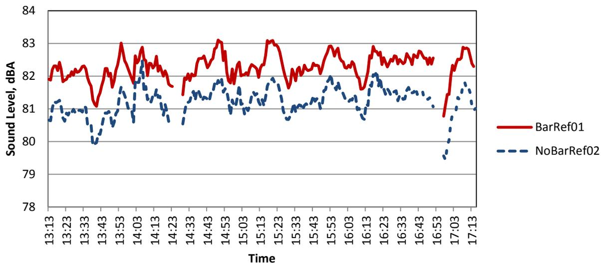
Figure 28. Running  $L_{eq}(5min)$ , I-24, A-weighted sound level, dBA, BarRef01 and NoBarRef02.
