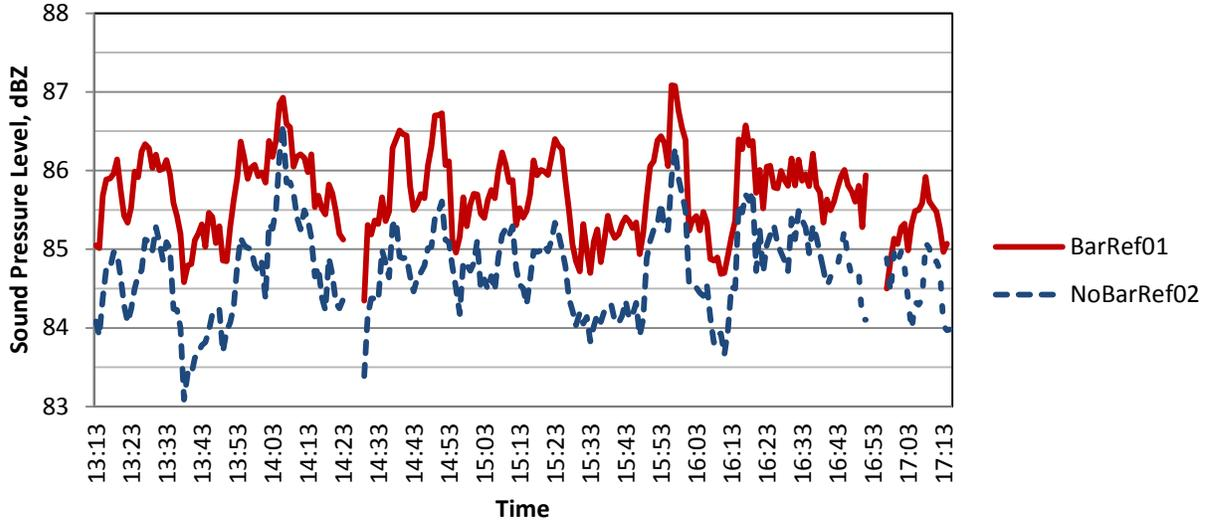
Figure 24. Running  $L_{eq}(5min)$ , I-24, unweighted sound pressure level, dBZ, BarRef01 and NoBarRef02.
