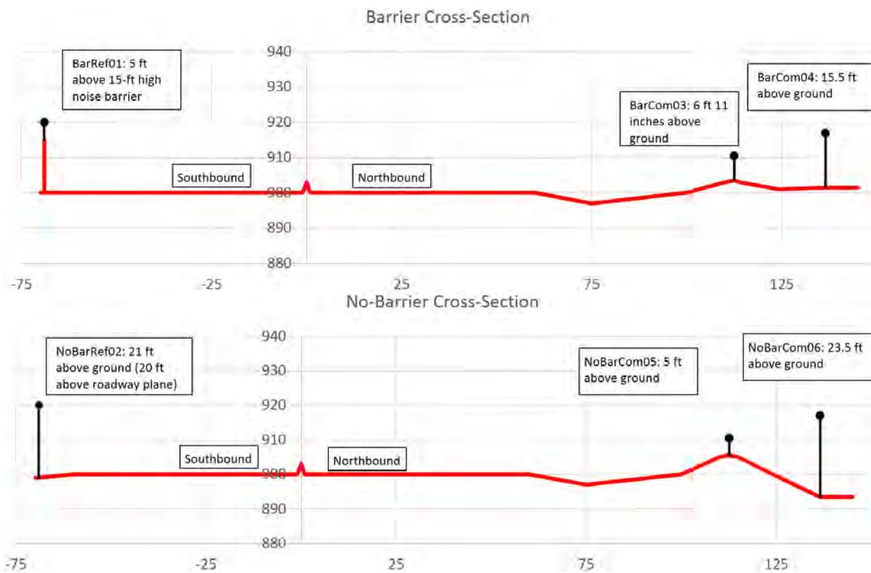
Figure 72. Cross-sections at the I-90 Barrier (top) and No Barrier (bottom) sites.
