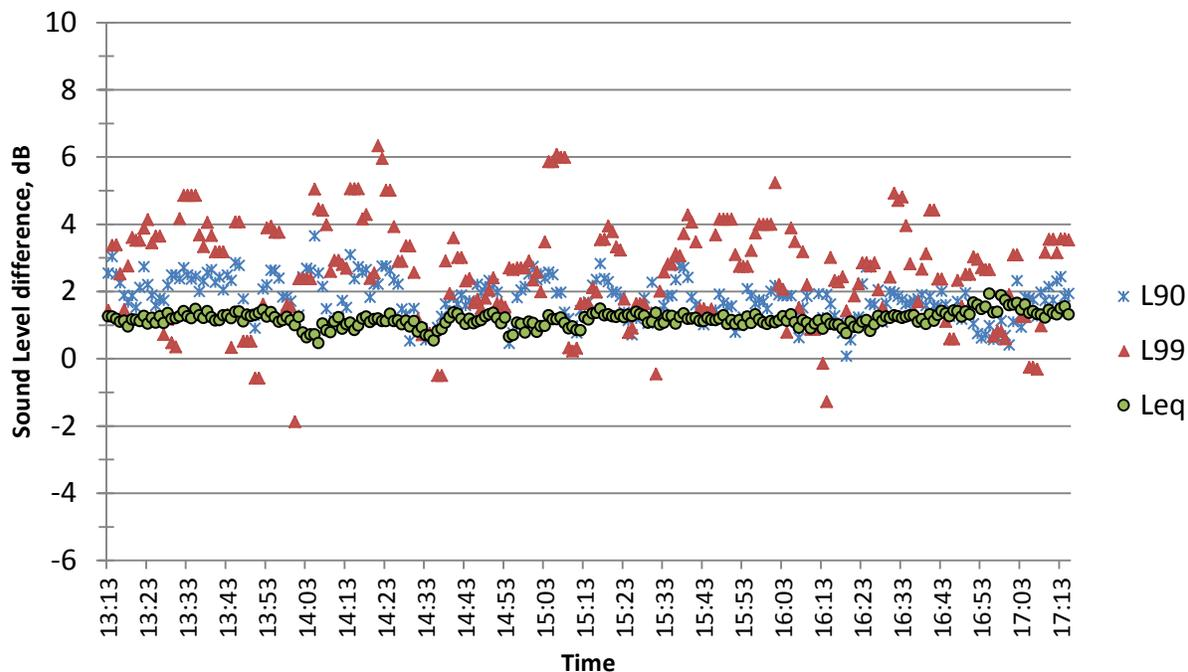
**Figure 36. Differences in broadband A-weighted 5-min  $L_{90}$ ,  $L_{99}$  and  $L_{eq}$ , I-24, BarRef1 and NoBarRef2.**
