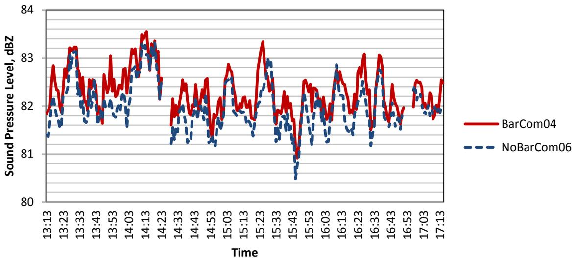
Figure 15. Running  $L_{eq}(5min)$ , I-24, unweighted sound pressure level, dBZ, BarCom04 and NoBarCom06.
