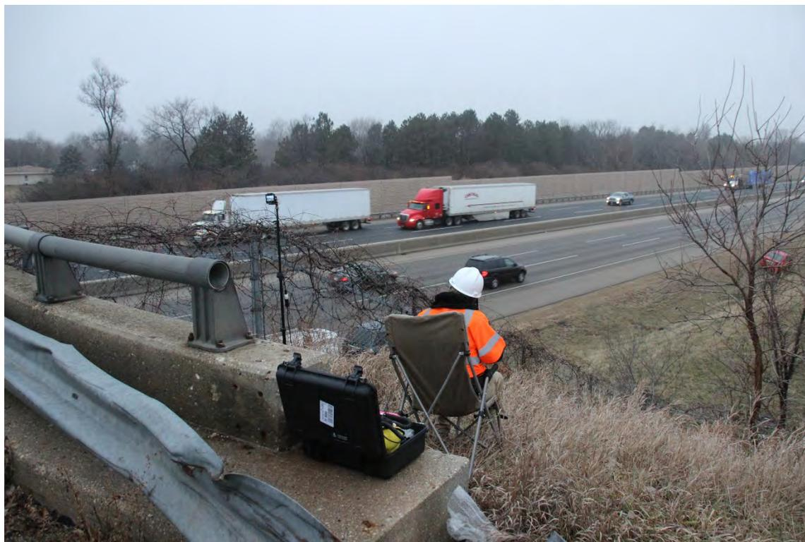
**Photograph 53. SID\_I90 Speed and Traffic Camera**
