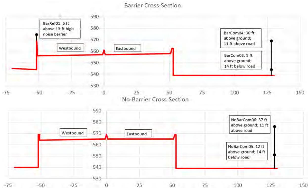
Figure 50. Cross-sections at the Briley Parkway Barrier (top) and No Barrier (bottom) sites.
