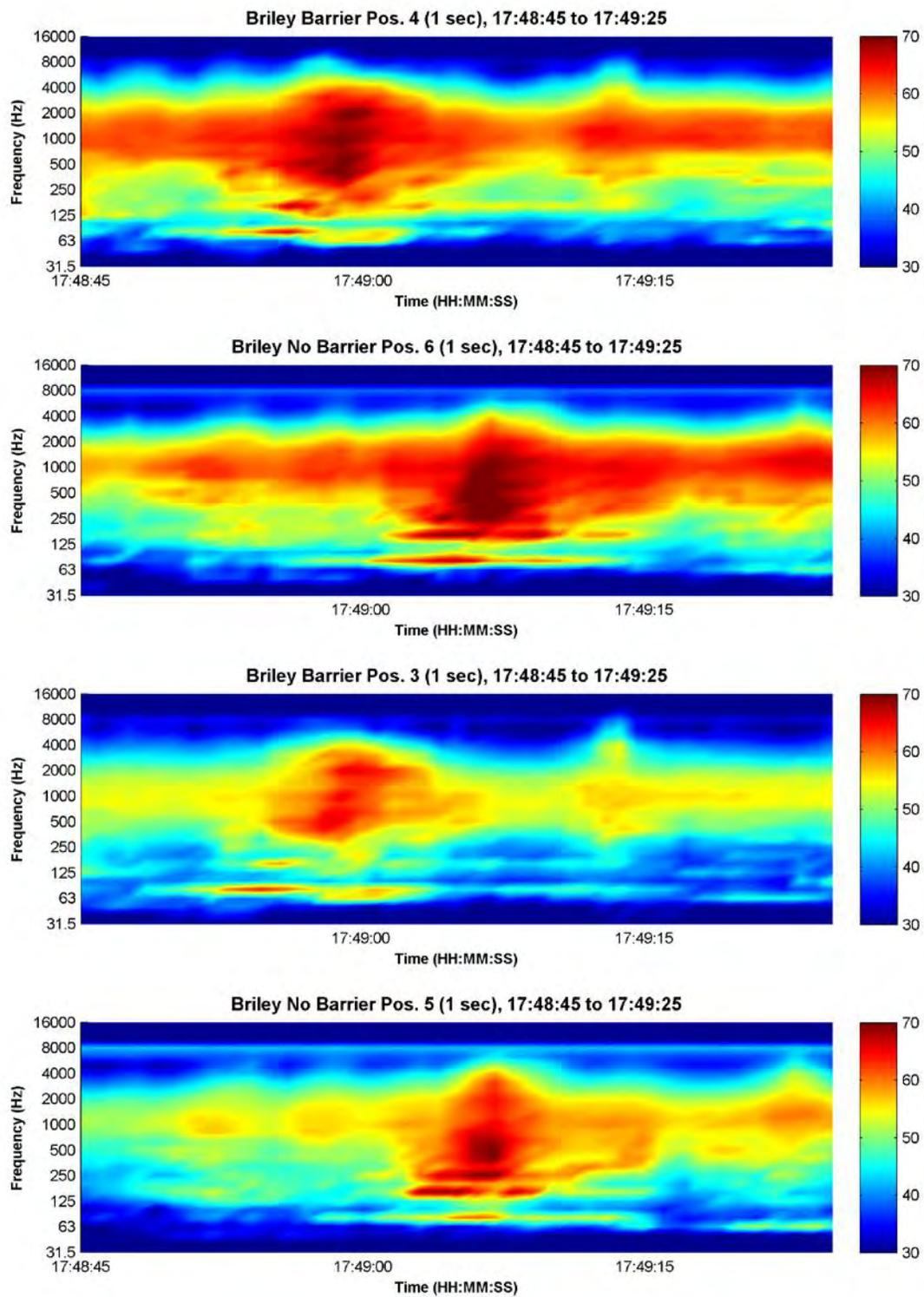
**Figure 69. Spectrogram for a heavy truck eastbound (example 1); top to bottom: high mics (BarCom04 and NoBarCom06), low mics (BarCom03 and NoBarCom05); Briley.**
