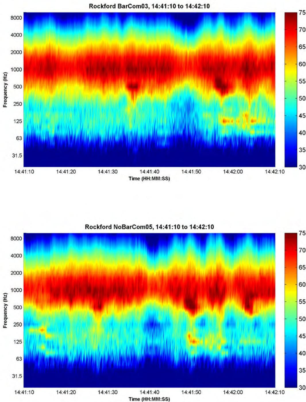
**Figure 101. I-90 spectrograms for a third heavy truck on northbound (barrier) side: top is BarCom03; bottom is NoBarCom05 (approximate event times: Barrier site 14:41:36, No Barrier site 14:41:27).**
