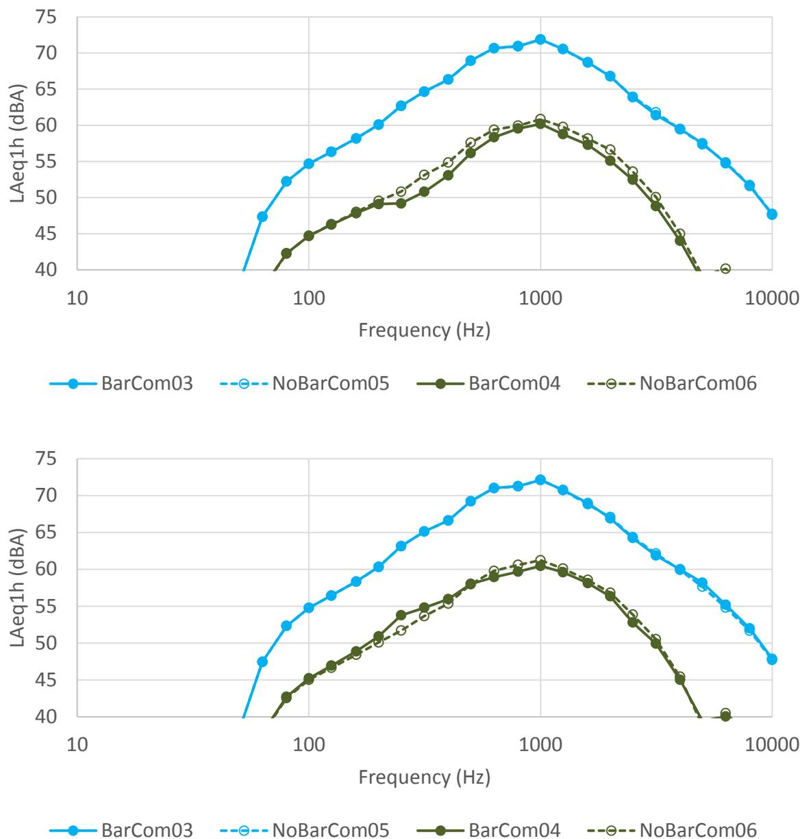
**Figure 133. TNM modeling results: TNM soft ground (top) and TNM hard ground (bottom), SR-71.**
