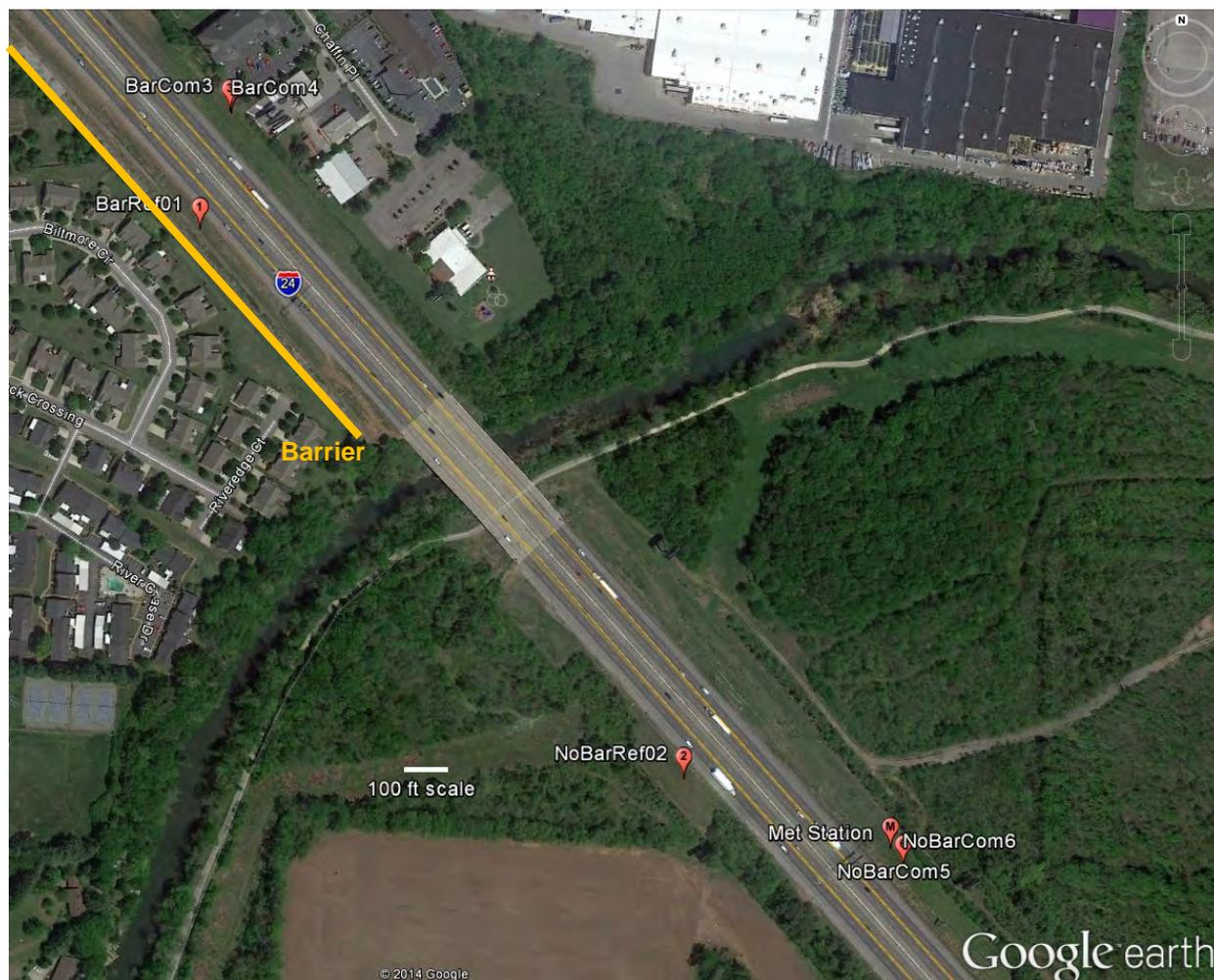
**Figure 4. I-24 microphone positions. (Source: Google Earth.)**
