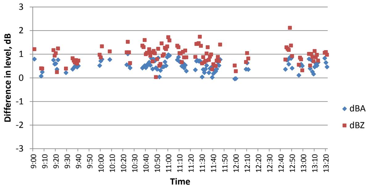
**Figure 30. Differences in running  $L_{eq}(5min)$ , SR-71, BarRef01 minus NoBarRef02.**
