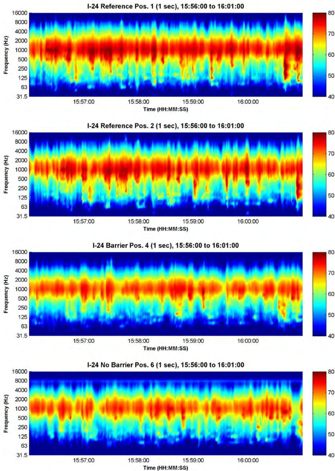
**Figure 40. I-24 5-minute spectrograms; top to bottom: BarRef01, NoBarRef02, high mics (BarCom04 and NoBarCom06); for Calm Lapse group CLG-6-1, start time 15:56.**
