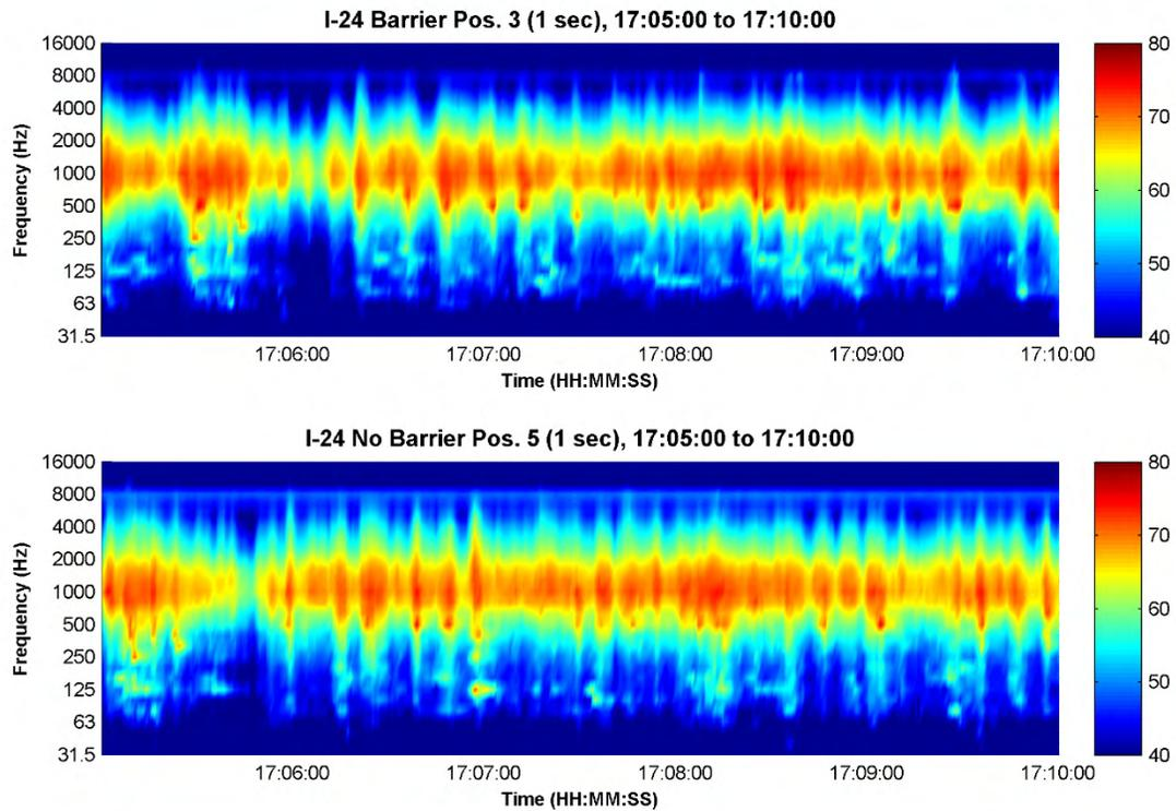
**Figure 43. I-24 5-minute spectrograms; top to bottom: lows mics BarCom03 and NoBarCom05; for Calm Neutral group CNG-2-1, start time 17:05.**
