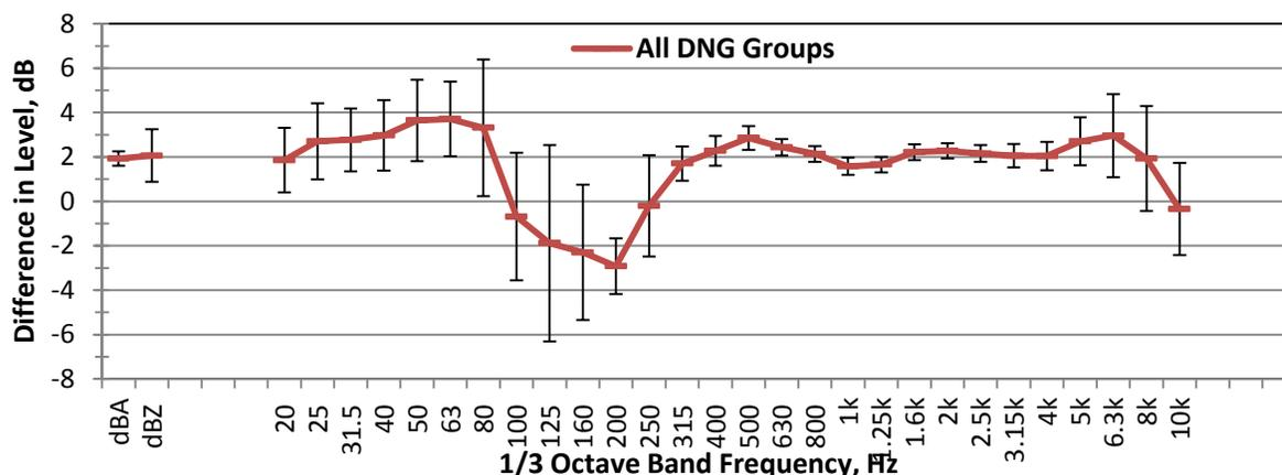
**Figure 63. Averages of the differences in  $L_{eq}(5min)$  +/- one standard deviation (dB), BarCom04 minus NoBarCom06, for all Downwind Neutral groups, SR-71.**
