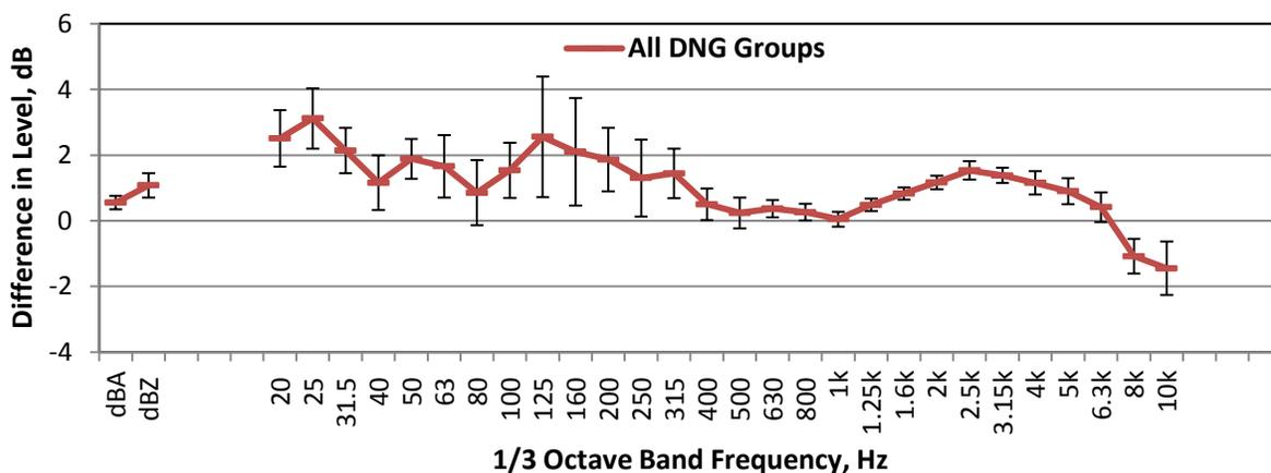
Figure 34. Averages of the differences in  $L_{eq}(5min)$  +/- one standard deviation (dB), all microphones, for all Downwind Neutral groups, SR-71.
