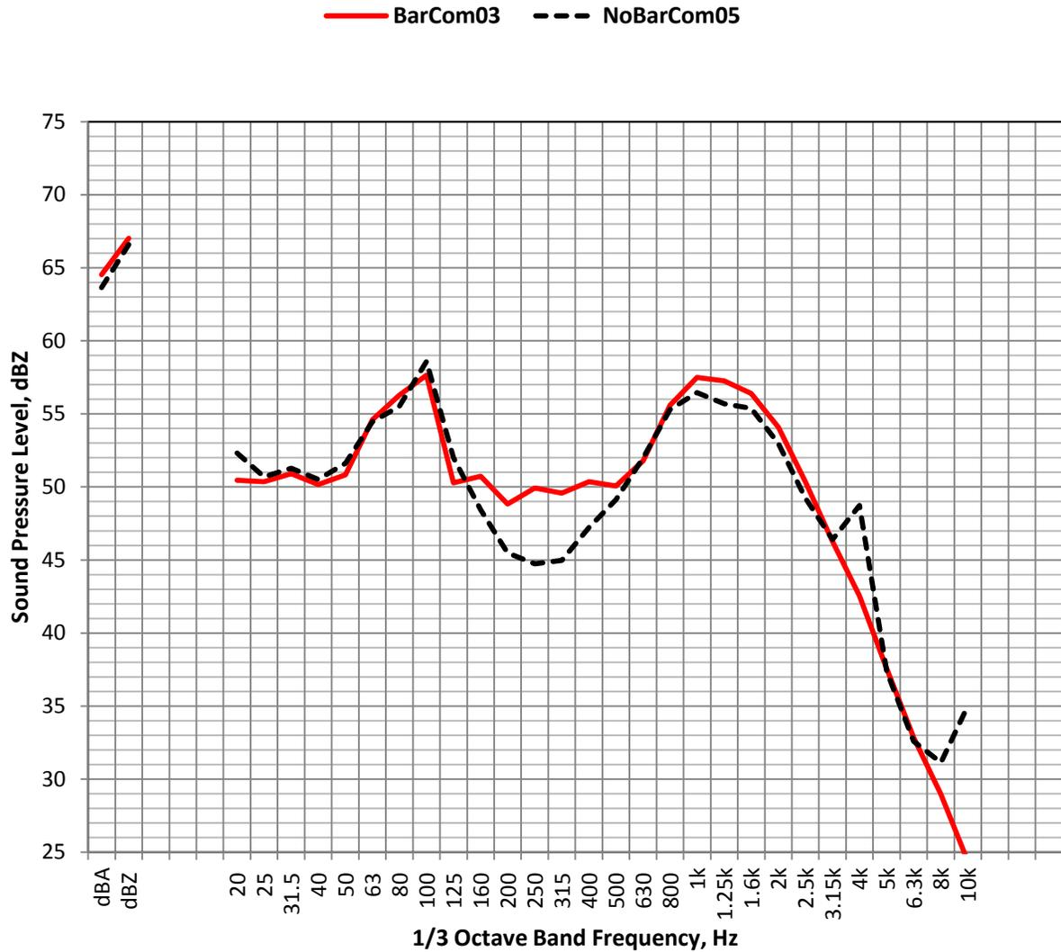
Figure 26. Sample sound pressure level spectra for BarCom03 and NoBarCom05, MD-5, Calm Inversion Group CIG-3-4, 23:15 ( $L_{eq}(5min)$ , dBZ).
