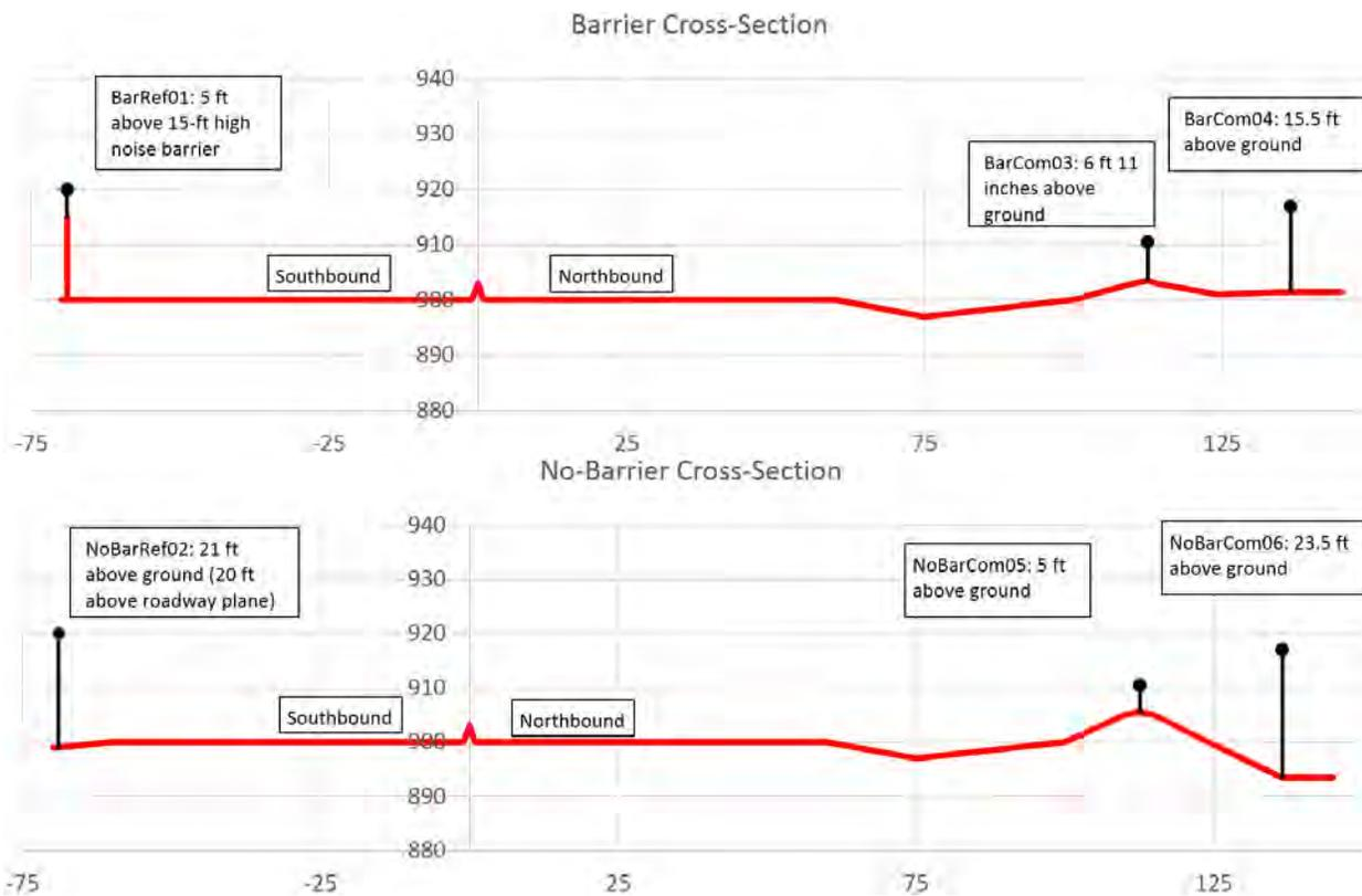
Figure 13. Cross-sections at the I-90 Barrier (top) and No Barrier (bottom) sites.
