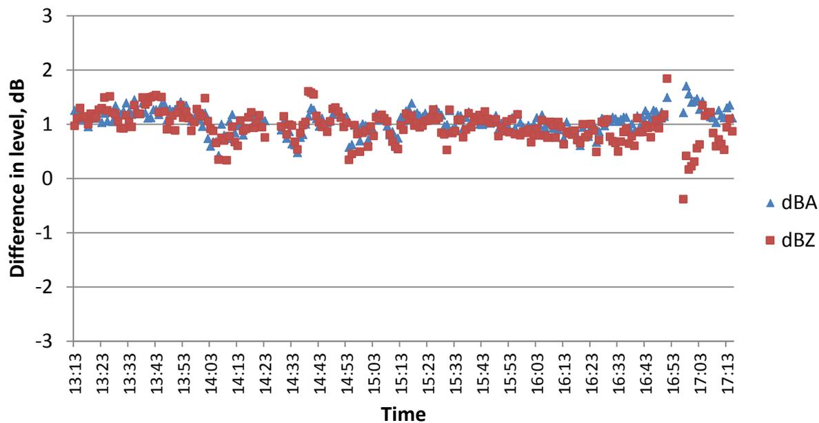
Figure 29. Differences in running  $L_{eq}(5min)$ , I-24, BarRef01 minus NoBarRef02.
