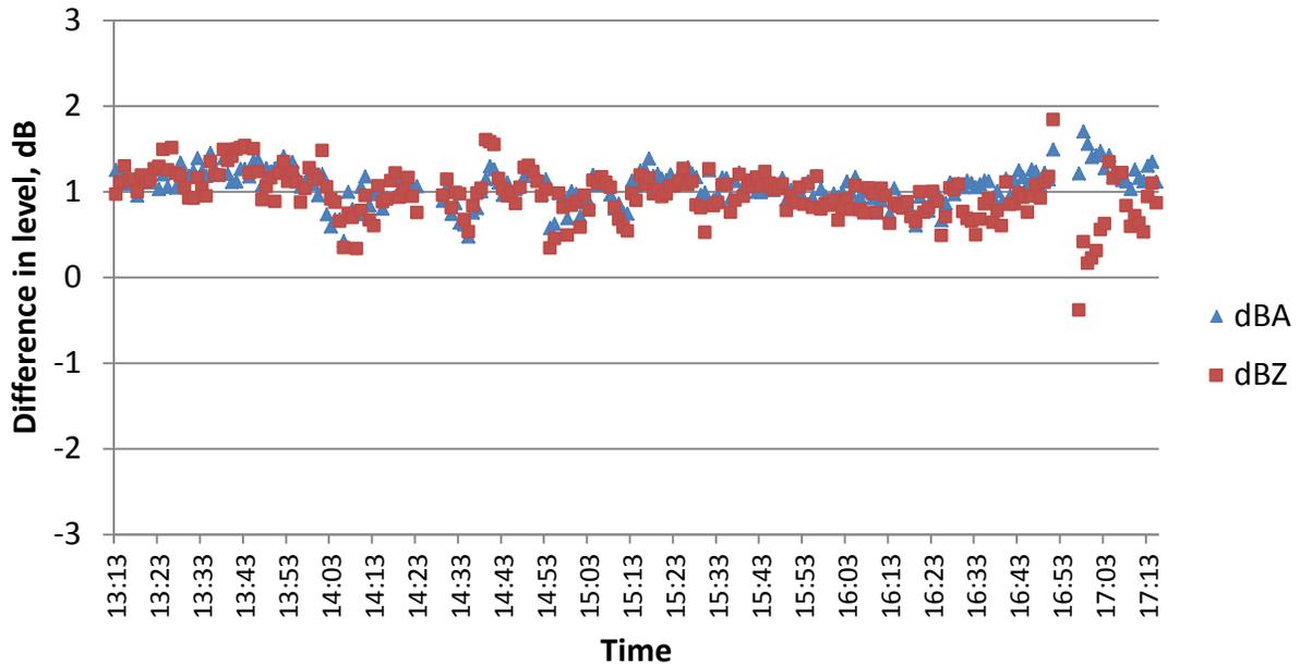
Figure 25. Differences in running  $L_{eq}(5min)$ , I-24, BarRef01 minus NoBarRef02.
