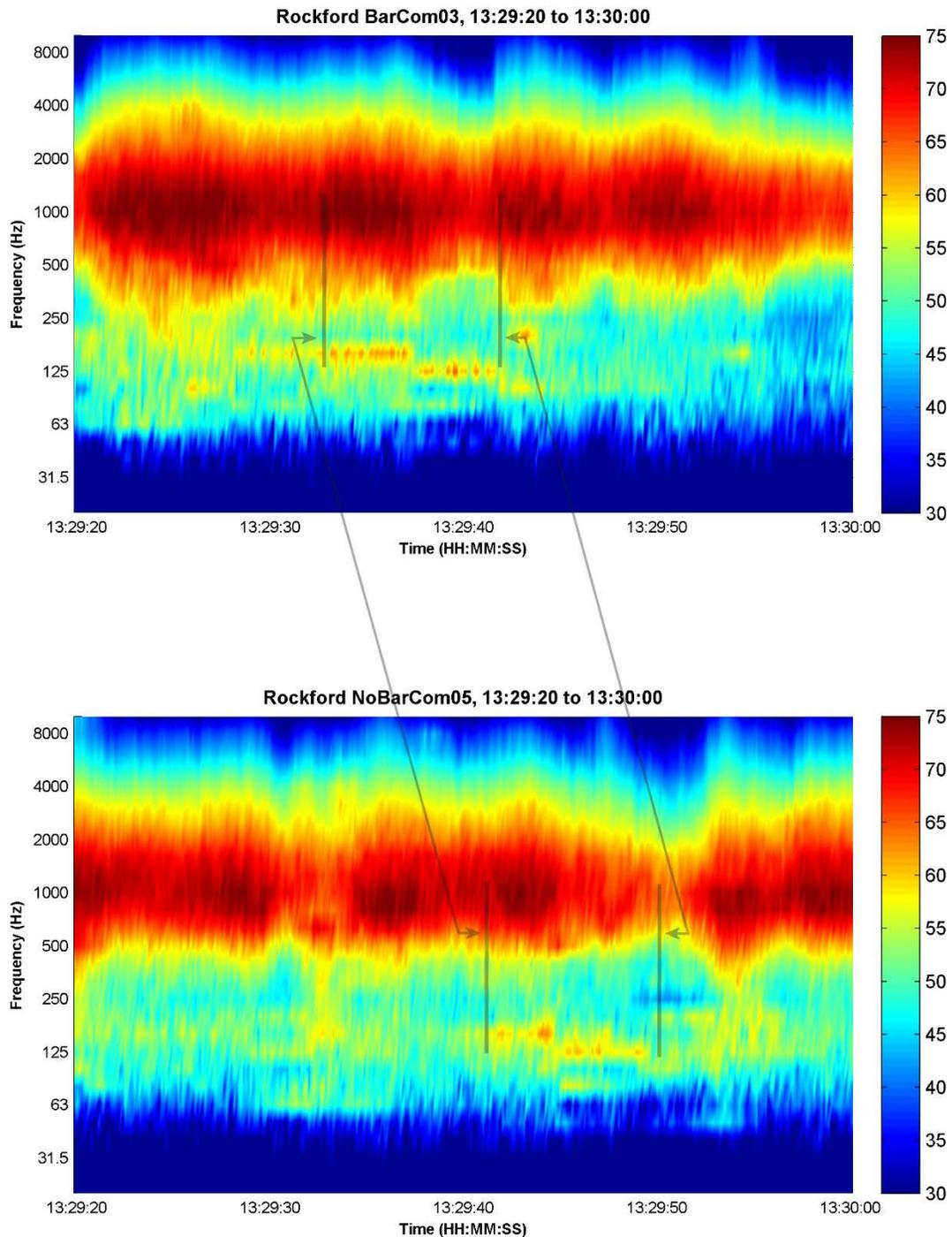
**Figure 75. I-90 spectrograms for a heavy truck on southbound (community) side (approximate event times: Barrier site 13:29:36, No Barrier site 13:29:43). Top is BarCom03; bottom is NoBarCom05.**
