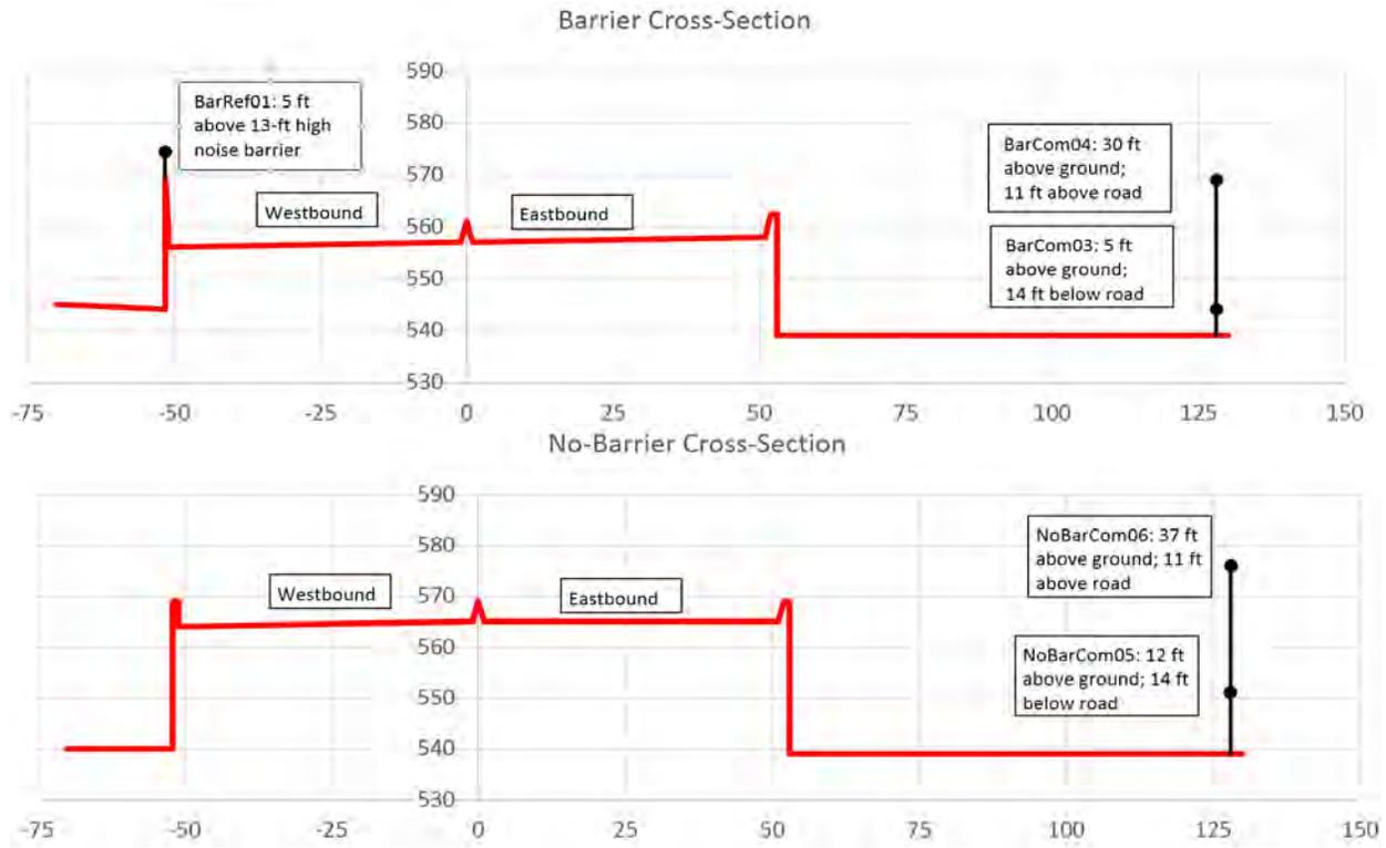
**Figure 9. Cross-sections at the Briley Parkway Barrier (top) and No Barrier (bottom) sites.**
