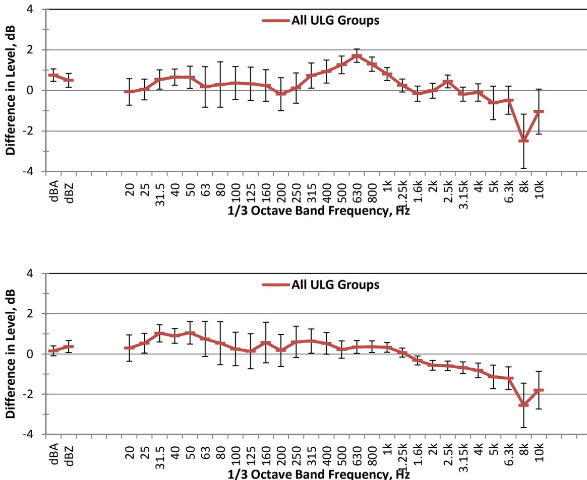
**Figure 66. Averages of the differences in  $L_{eq}(5min)$  +/- one standard deviation (dB), BarCom03 and NoBarCom05 (top) and BarCom04 and NoBarCom06 (bottom), for all Upwind Lapse groups, I-24.**
