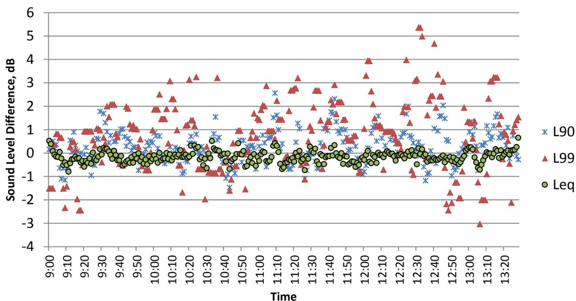
**Figure 47. Differences in broadband A-weighted 5-min  $L_{90}$ ,  $L_{99}$  and  $L_{eq}$ , SR-71, BarCom03 minus NoBarCom05.**
