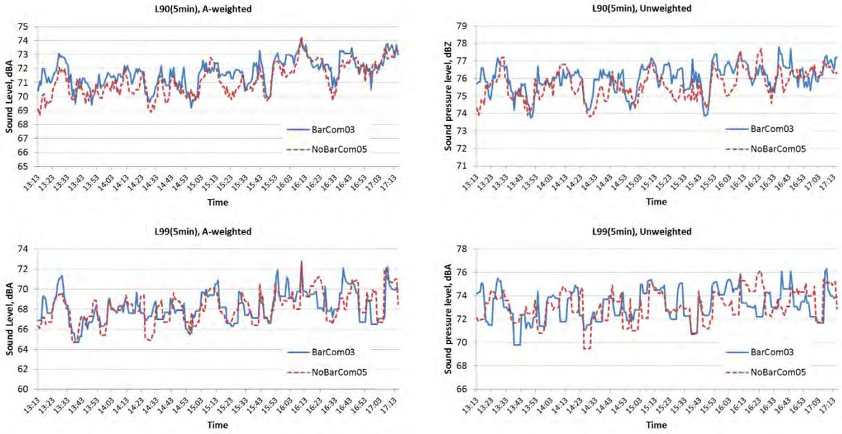
**Figure 30.**  $L_{90}(5min)$  and  $L_{99}(5min)$ , I-24, BarCom03 and NoBarCom05 – broadband A-weighted sound level (left) and sound pressure level (right).
