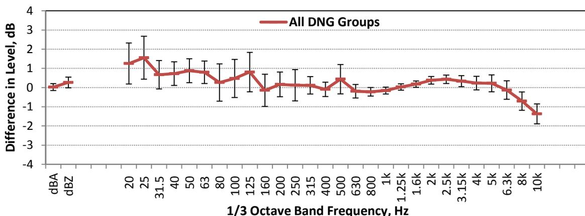
**Figure 46. Averages of the differences in  $L_{eq}(5min)$  +/- one standard deviation (dB), BarCom03 minus NoBarCom05 for all Downwind Neutral groups, SR-71.**
