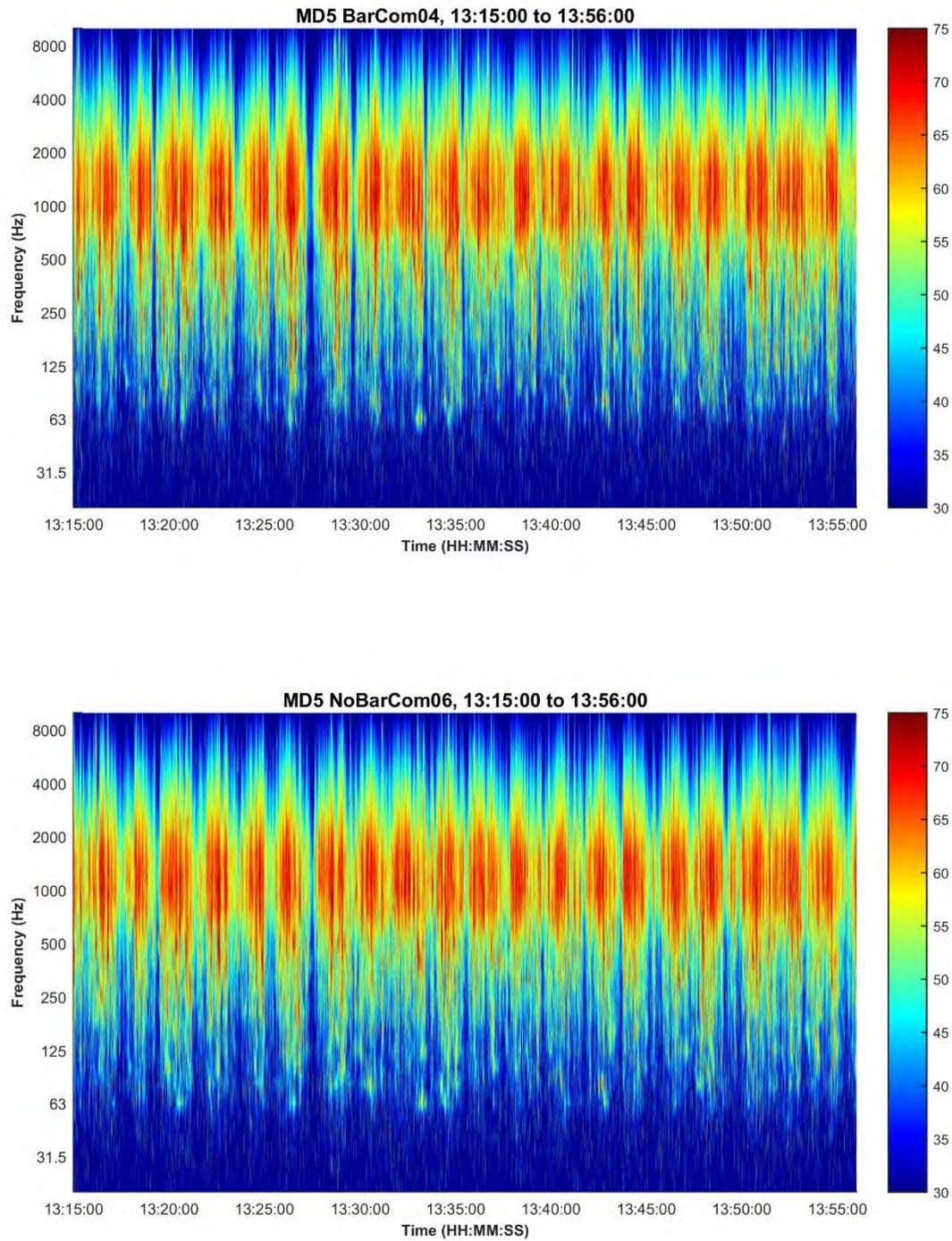
**Figure 188. MD-5 spectrograms for Forty-one minutes of clean data (no contamination from other noise sources): top is BarCom04; bottom is NoBarCom06.**
