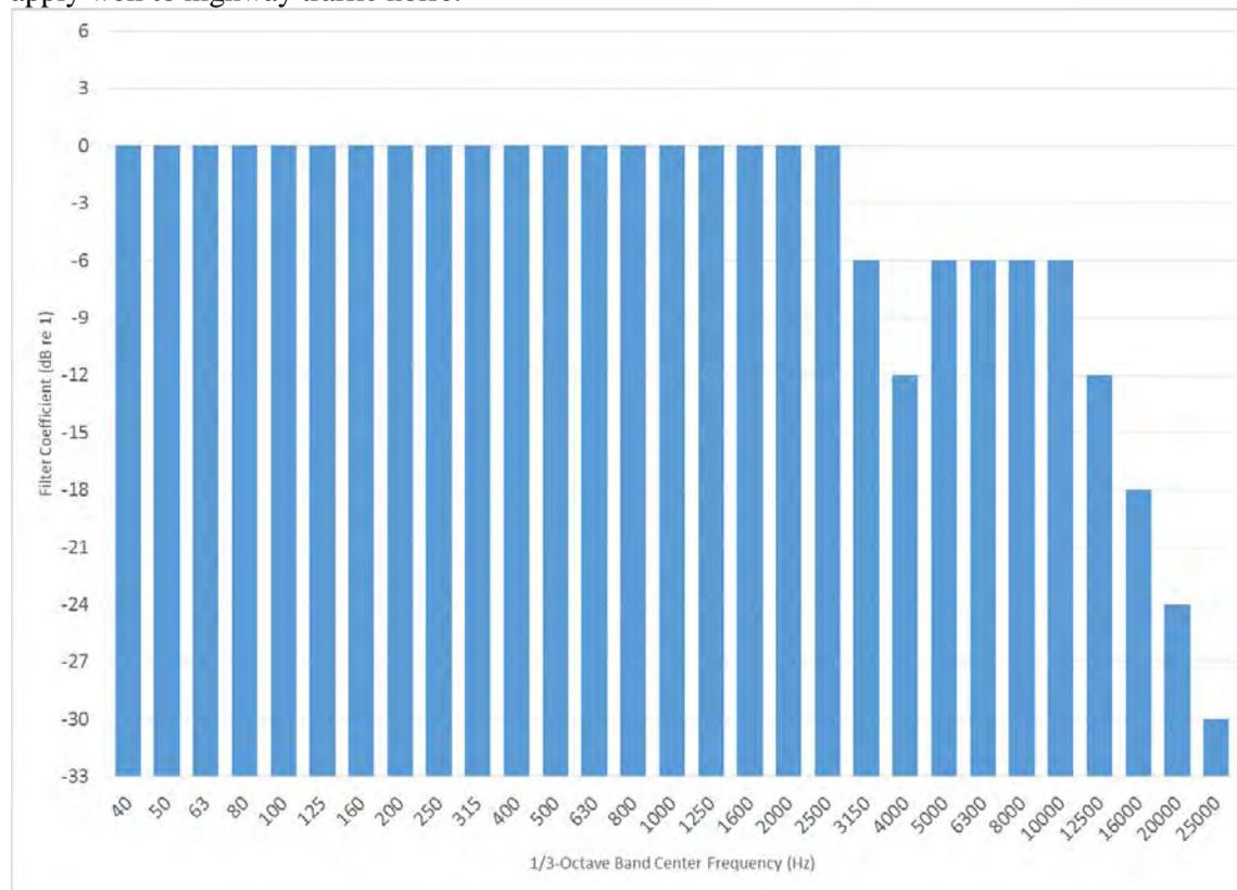
Figure 193. 1/3-octave band graphic equalization applied to nighttime audio.
