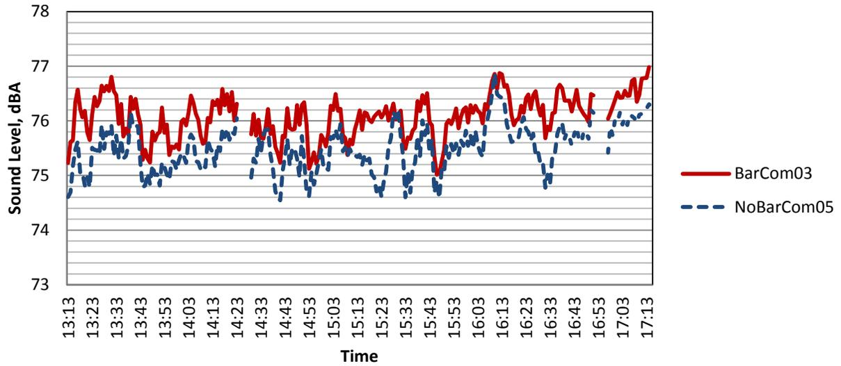
Figure 13. Running  $L_{eq}(5min)$ , I-24, A-weighted sound level, dBA, BarCom03 and NoBarCom05.
