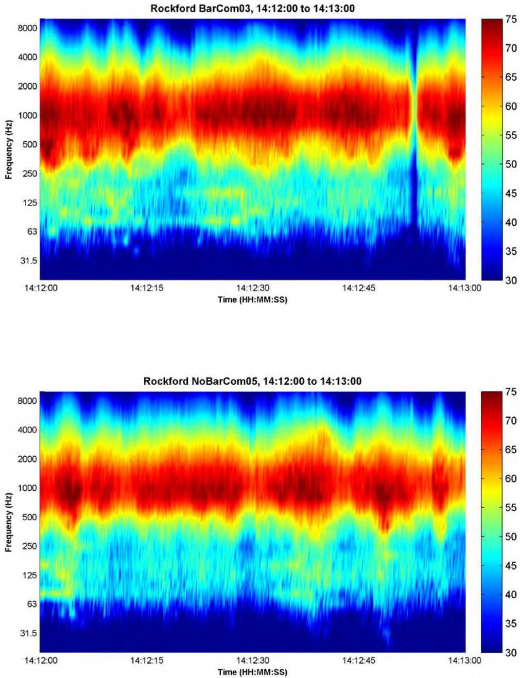
Figure 100. I-90 spectrograms for a second heavy truck on southbound (community) side: top is BarCom03; bottom is NoBarCom05 (approximate event times: Barrier site 14:12:34, No Barrier site 14:12:40).
