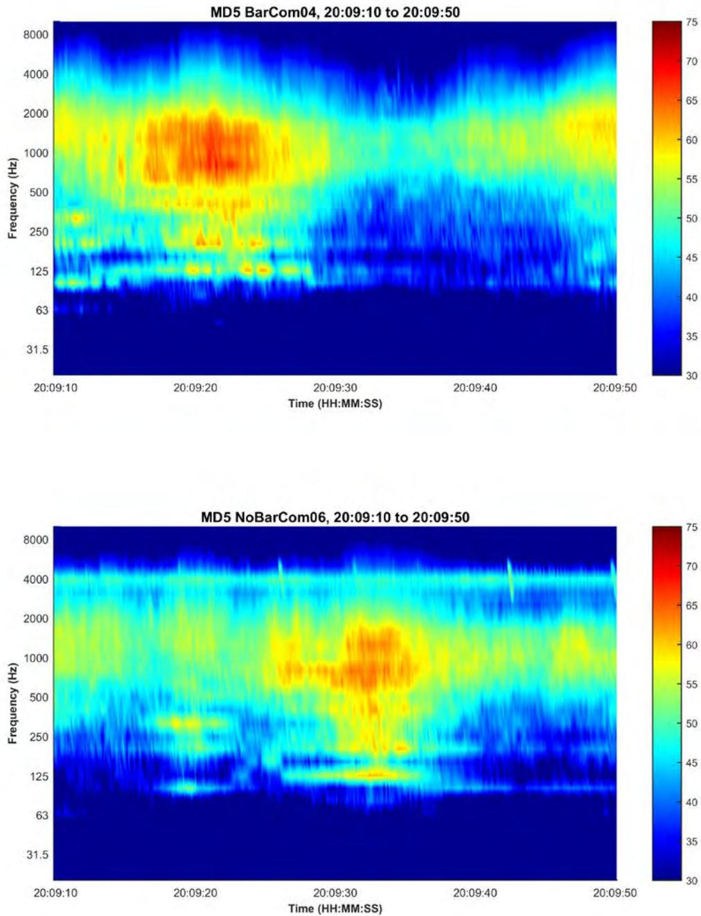
**Figure 186. MD-5 spectrograms for a pickup truck on southbound (barrier) side (approximate event times: Barrier site 20:09:20, No Barrier site 20:09:35.) Additional vehicle follows the heavy truck: top is BarCom04; bottom is NoBarCom06.**
