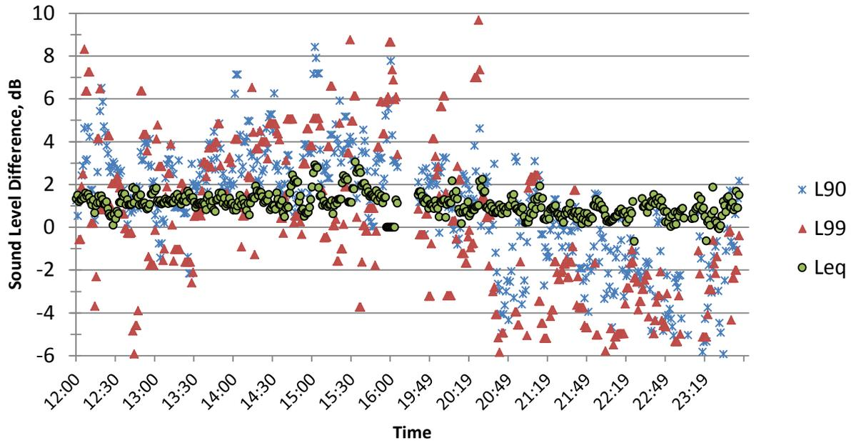
**Figure 59. Differences in broadband A-weighted 5-min  $L_{90}$ ,  $L_{99}$  and  $L_{eq}$ , MD-5, BarCom03 and NoBarCom05.**
