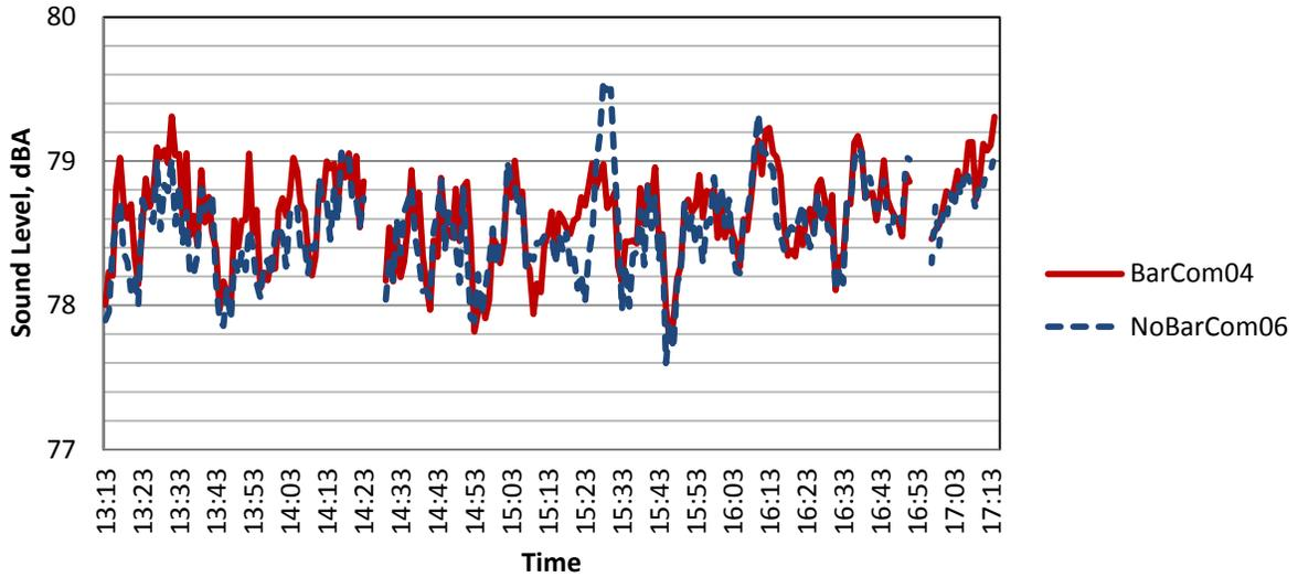
Figure 16. Running  $L_{eq}(5min)$ , I-24, A-weighted sound level, dBA, BarCom04 and NoBarCom06.
