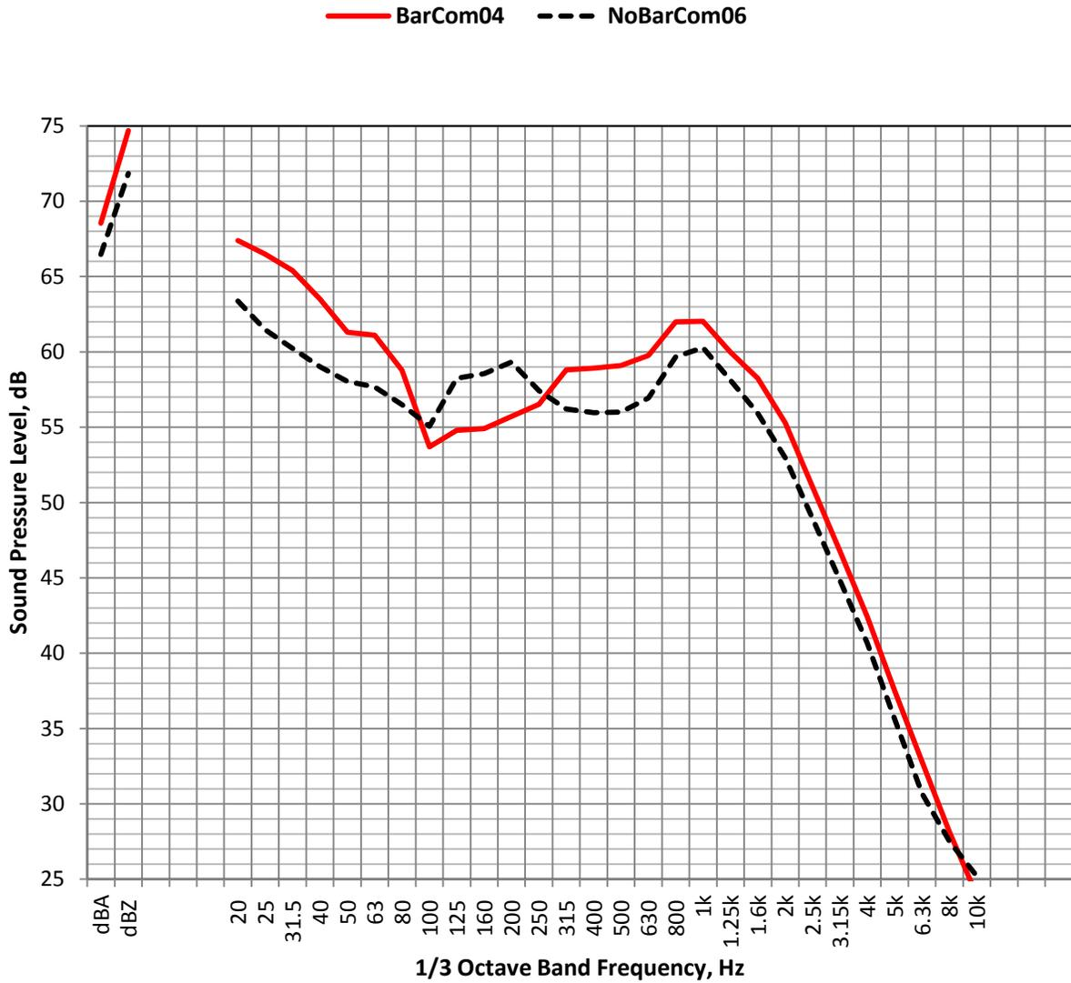
**Figure 62. Sample sound pressure level spectra for BarCom04 and NoBarCom06, SR-71, Downwind Neutral group DNG-3-2, 11:38-11:43 ( $L_{eq}(5min)$ , dBZ).**
