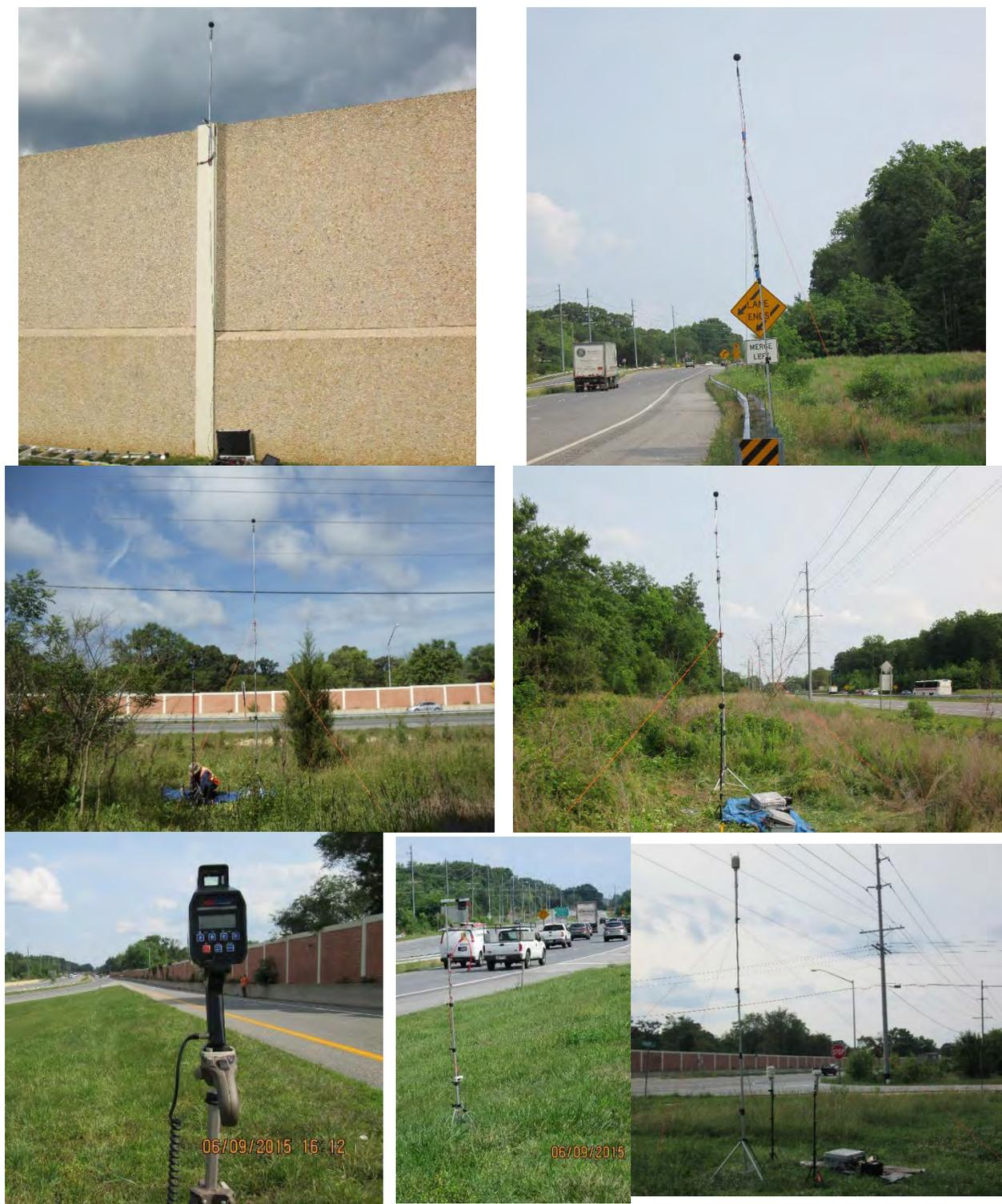
**Figure 23. MD-5 BarRef01 (top left), NoBarRef02 (top right), BarCom03 and BarCom04 (middle left), NoBarCom05 and NoBarCom06 (middle right), traffic speed (bottom left), traffic video (bottom middle), meteorological station (bottom right) (Source: research team members).**
