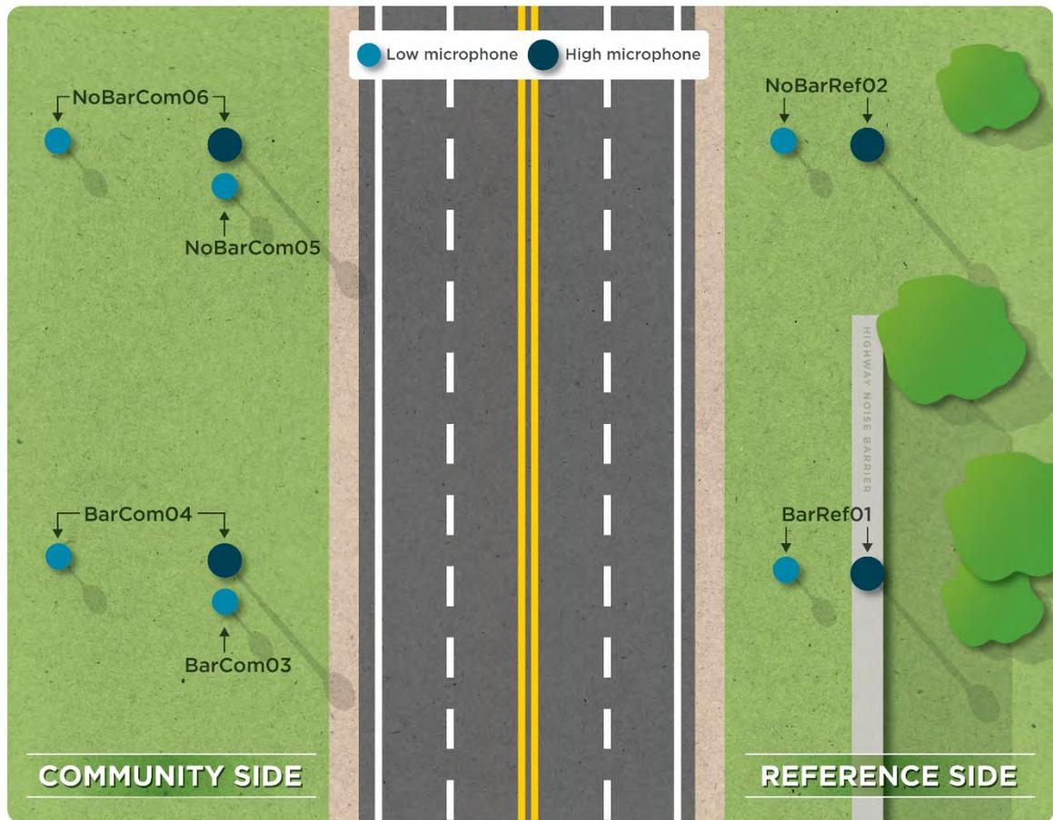
**Figure 2. Typical microphone positions.**
