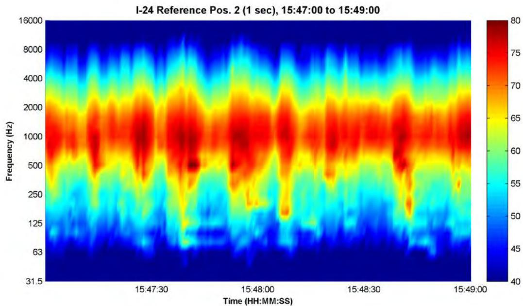
Figure 44. I-24 spectrograms for a group of heavy trucks; top to bottom: BarRef01, NoBarRef02.
