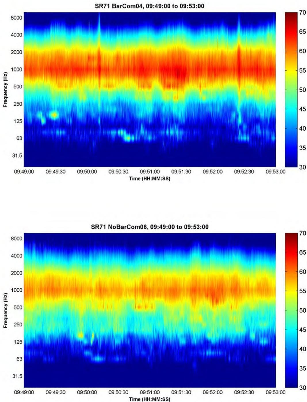
**Figure 76. SR-71 spectrograms for 4-minute block of data in the morning at 09:49: top is BarCom04; bottom is NoBarCom06.**
