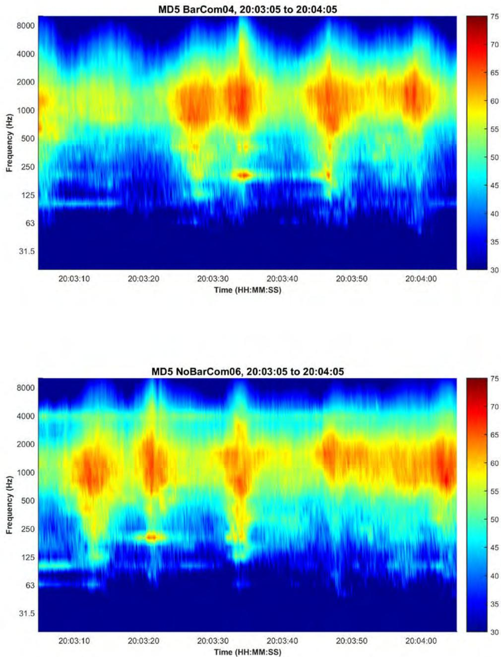
**Figure 187. MD-5 spectrograms for Motorcycle on northbound (community) side. (approximate event times: Barrier site 20:03:35, No Barrier site 20:03:22.) Additional vehicles come before and after the motorcycle: top is BarCom04; bottom is NoBarCom06.**
