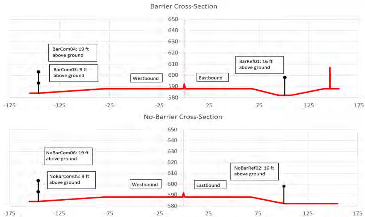
**Figure 5. Cross-sections at the I-24 Barrier (top) and No Barrier (bottom) sites.**
