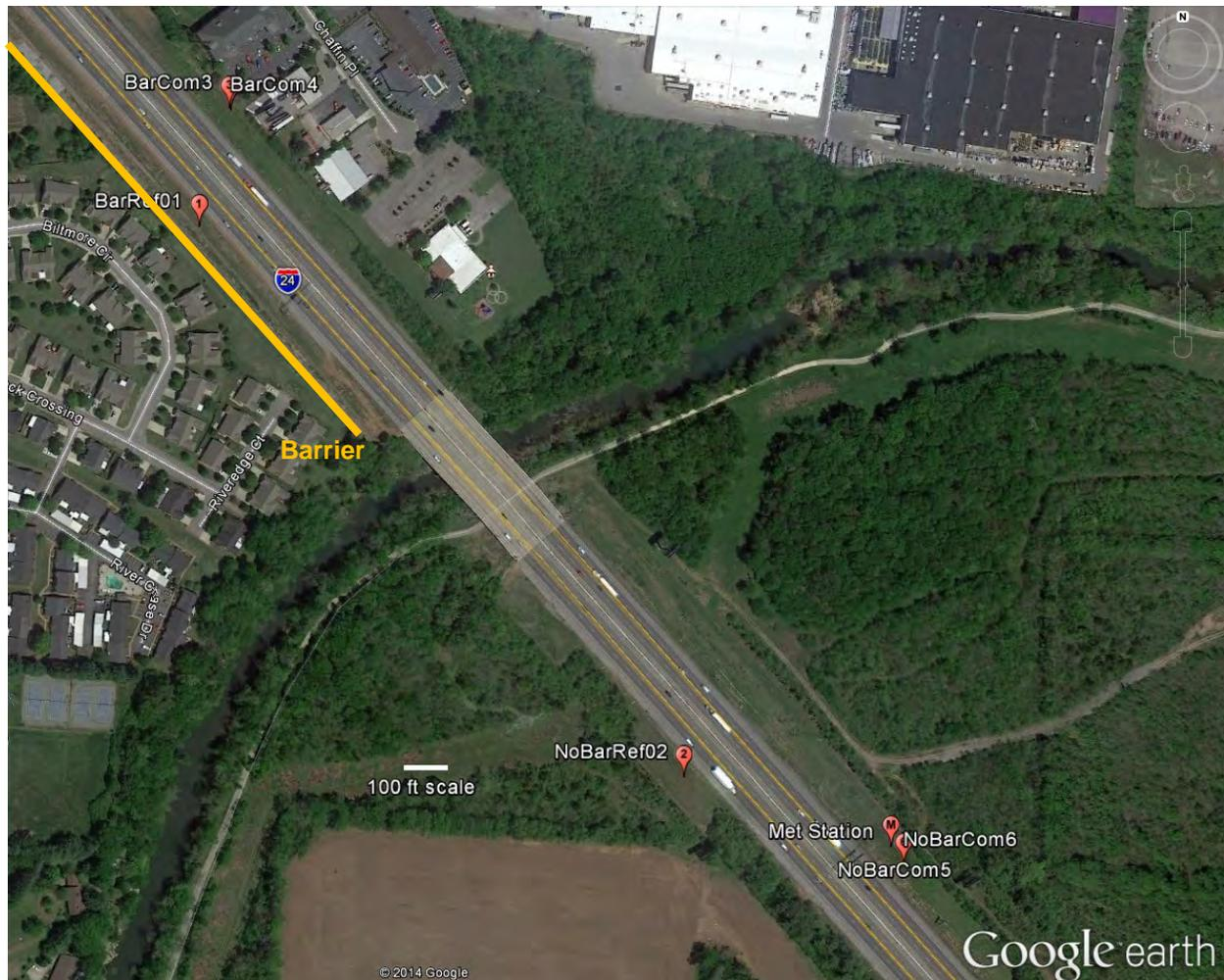
**Figure 7. I-24 microphone positions. (Source: Google Earth.)**
