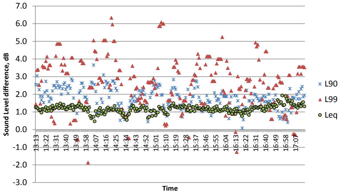
Figure 29. Differences in broadband A-weighted 5-min  $L_{90}$ ,  $L_{99}$  and  $L_{eq}$ , I-24, BarRef1 and NoBarRef2
