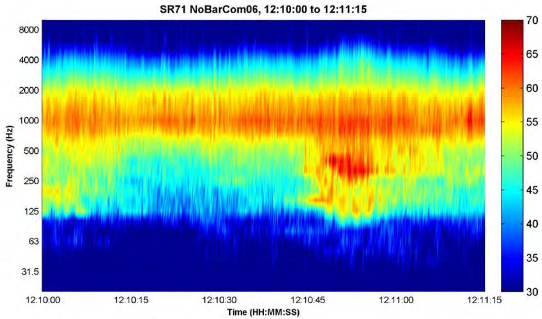
**Figure 135. SR-71 spectrograms for motorcycle on southbound (community) side: top is BarCom04; bottom is NoBarCom06.**
