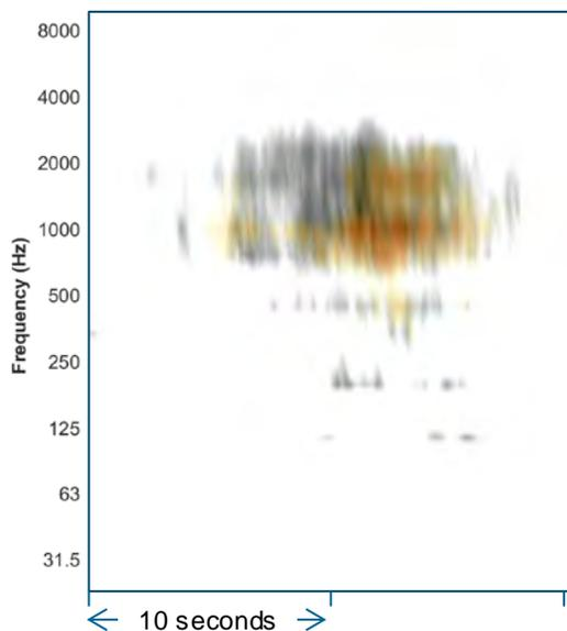
**Figure 74. Overlay of MD-5 pickup truck passby hot spots for levels greater than ~60 dBA: BarCom04 (hot spot now represented in gray/black) and NoBarCom06 (hot spot represented in orange/red).**
