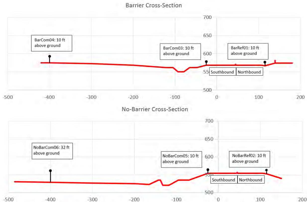
**Figure 108. Cross-sections at the SR-71 Barrier (top) and No Barrier (bottom) sites.**
