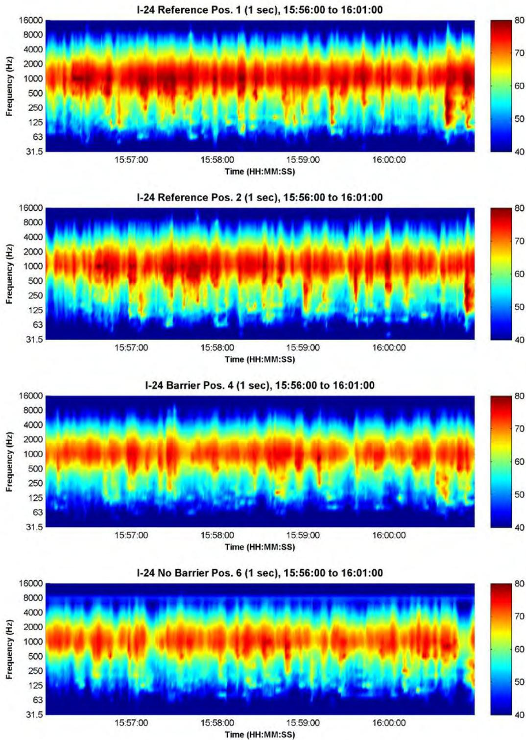
**Figure 77. I-24 five-minute spectrograms; top to bottom: BarRef01, NoBarRef02, high mics (BarCom04 and NoBarCom06); for Calm Lapse group CLG-6-1, start time 15:56.**
