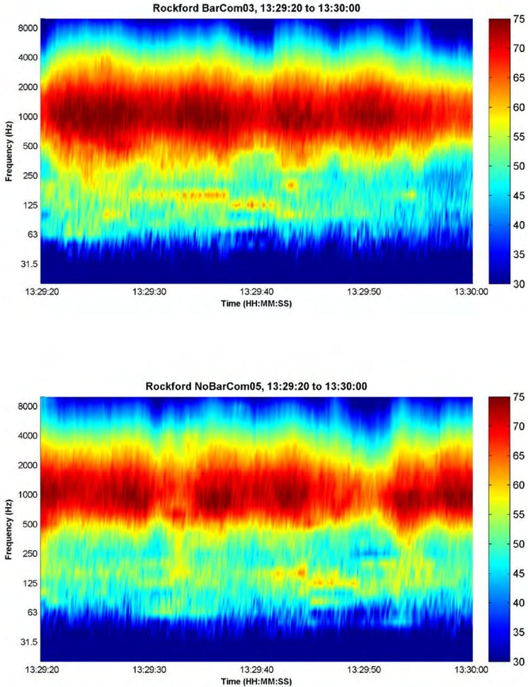
**Figure 99.** I-90 spectrograms for a heavy truck on southbound (community) side: top is BarCom03; bottom is NoBarCom05 (approximate event times: Barrier site 13:29:36, No Barrier site 13:29:43).
