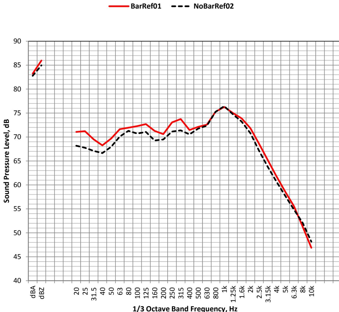
**Figure 32. Sample sound pressure level spectra for BarRef01 and NoBarRef02, SR-71, Downwind Neutral group DNG-3-2, 11:38-11:43 ( $L_{eq}(5min)$ , dBZ).**
