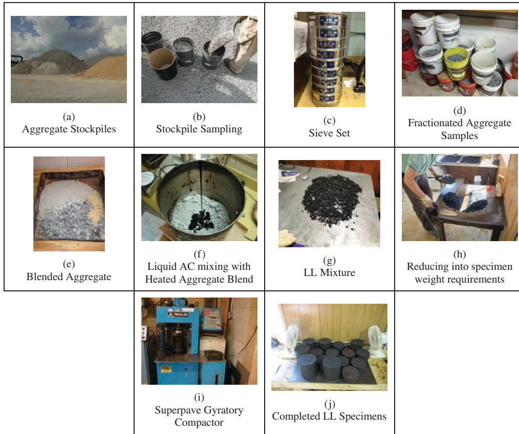
Figure 4-1. Laboratory-mixed-laboratory-compacted (LL) specimen fabrication.
