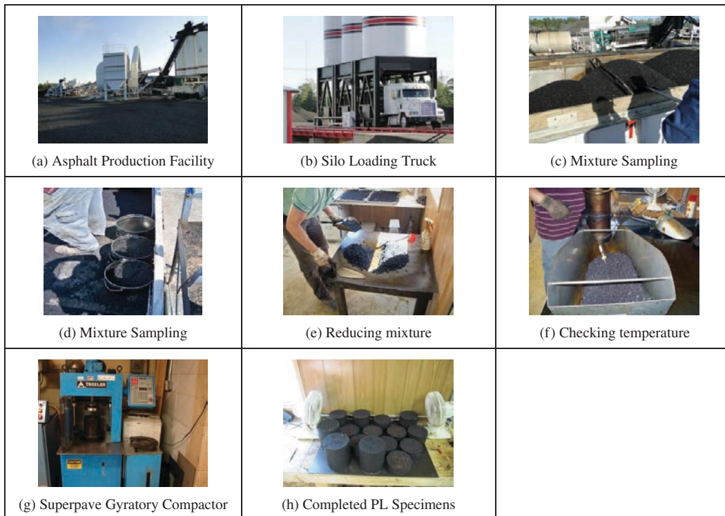
Figure 4-2. Plant-mixed-laboratory-compacted (PL) specimen fabrication.
