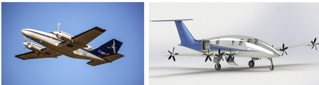
FIGURE 4.5 A nine-passenger Cape Air Cessna 402 and an advanced nine-passenger distributed electric propulsion conceptual aircraft. SOURCE: Courtesy of Cape Air ( left ) and NASA ( right ).
