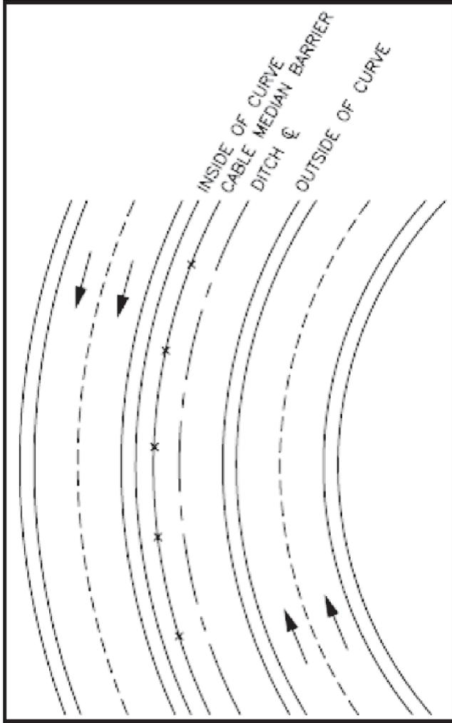
FIGURE 4 Recommended cable barrier placement on a horizontal curve (Figure 2-26 from Cooner et al. 2009).
