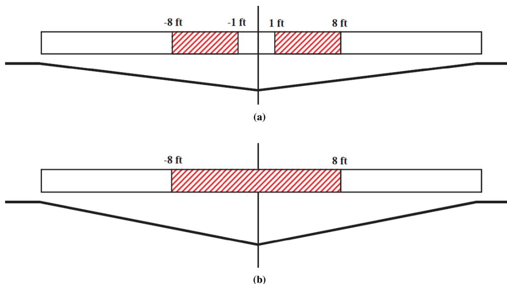
FIGURE 2 Override criteria for V-shaped medians (Figure 6.1 from *NCHRP Report 711*) (Marzougui et al. 2012).
