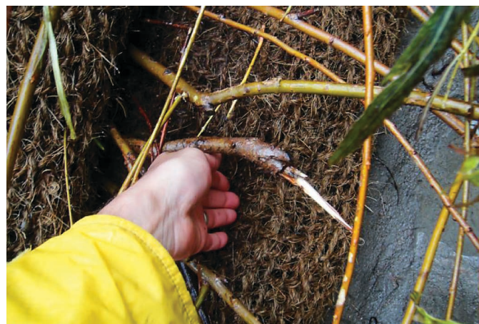
Figure 3.29. Photograph showing broken stem at the end of Test 6 (150 ft 3 /s).
