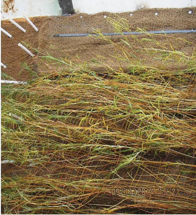
Figure 3.23. Tray 2 at the end of Test 6 (150 ft 3 /s). Note soil washout and collapse of the uppermost soil lift.
