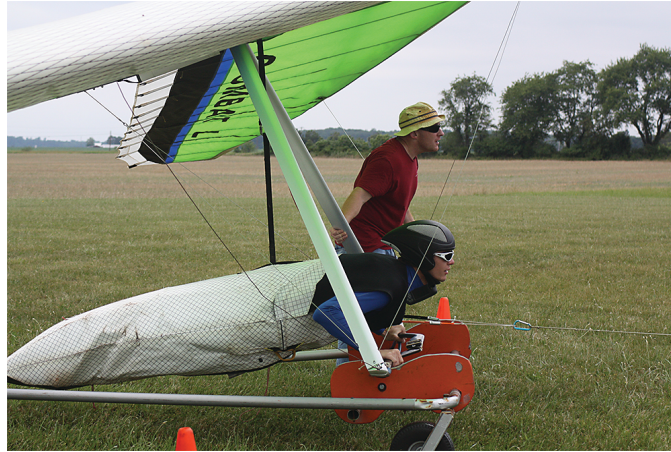
FIGURE 31 WSC hang glider positioned on a dolly for takeoff (Credit: A. Elchin, Highland Aerosports, Ridgely, Maryland. Used with permission.).
