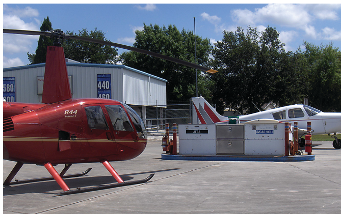
FIGURE 22 Helicopter positioned close to fuel pump for fueling purposes (Source: S. Quilty, SMQ Airport Services, Lutz, Florida. Used with permission.).
