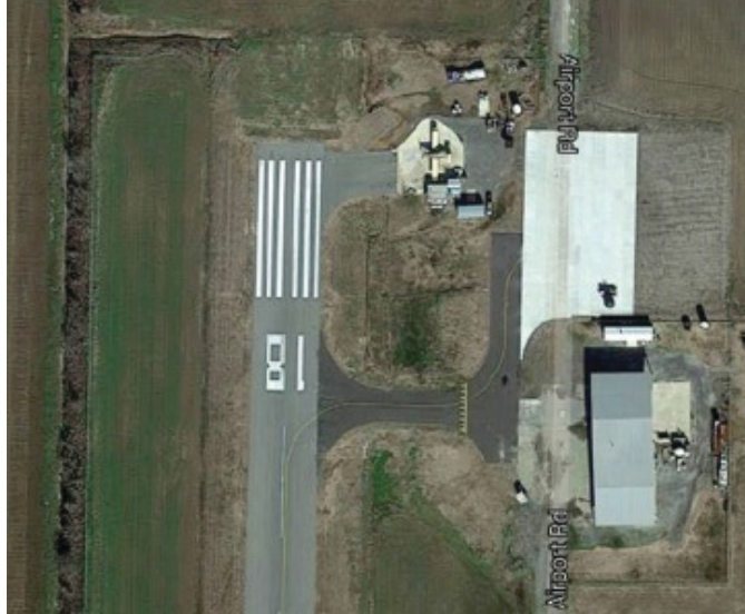
FIGURE 11 Staging of agricultural equipment near a runway end (Source: Imagery © 2015 DigitalGlobe, State of Arkansas, USDA Farm Service Agency; map data © 2015 Google. Fair use.).
