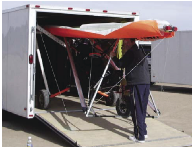
FIGURE 35 WSC aircraft transported in a trailer (Source: FAA 2008a.).
