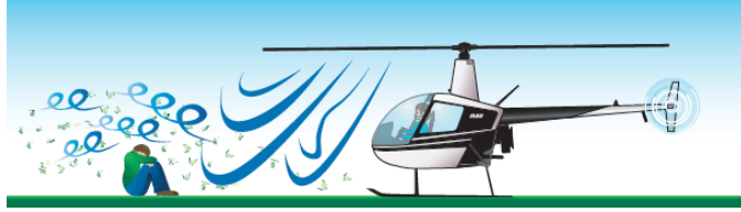
FIGURE 23 Rotor downwash is a major safety issue (Source: FAA 2012a).
