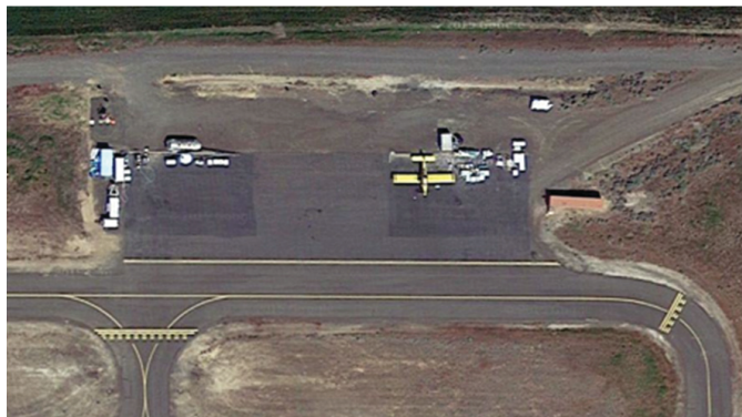
FIGURE 12 Staging of agricultural equipment near a runway end for two operators (Source: Imagery © 2015 DigitalGlobe, State of Oregon. Fair use.).
