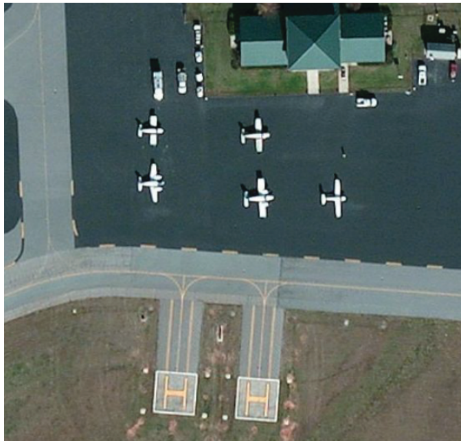
FIGURE 19 Helipad locations and markings at the Athens, Georgia, airport ( Source: © 2016 Microsoft Corporation © 2016 HERE. Fair use. ).
