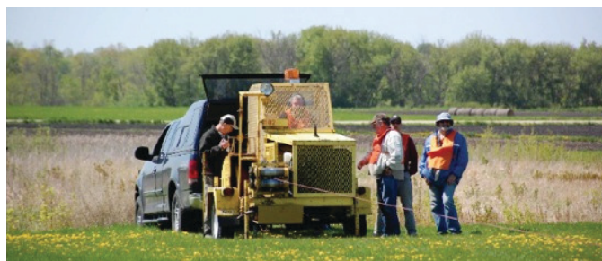
FIGURE 45 Glider winch equipment past the runway end (Credit: D. Ingraham, Cross Country Soaring, Faribault, Minnesota. Used with permission.).
