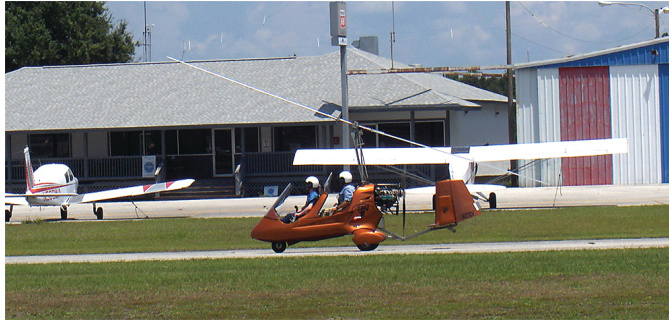
FIGURE 25 Two-seat light sport gyroplane ( Credit: S. Quilty, SMQ Airport Services, Lutz, Florida. Used with permission. ).
