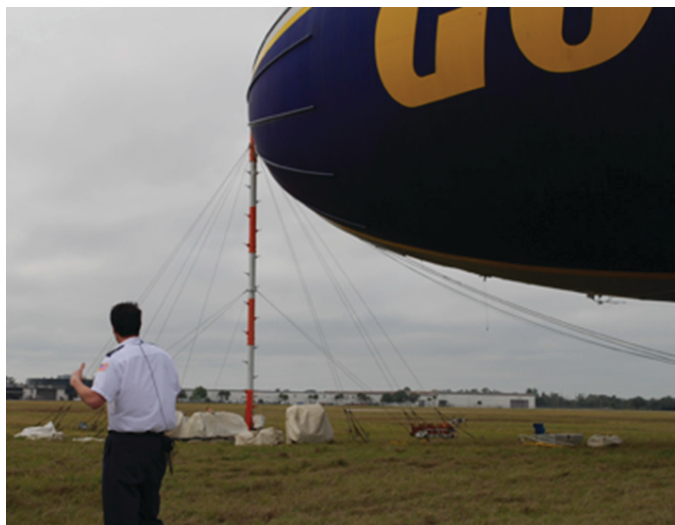
FIGURE 10 Blimp moored at the bow ( Credit: S. Walsh, Lakeland Linder Regional Airport, Florida. Used with permission. )
