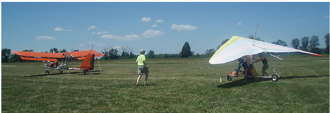
FIGURE 32 Powered ultralight towing an unpowered WSC hang glider set on a dolly (Credit: A. Elchin, Highland Aerosports, Ridgely, Maryland. Used with permission.).
