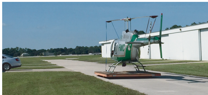
FIGURE 20 Portable dolly used to position skid-equipped helicopter (Source: E. Conrad, Lakeland Linder Regional Airport, Florida. Used with permission.).
