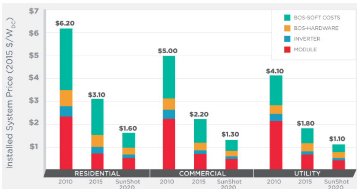
FIGURE 2.3 Installed photovoltaic (PV) system prices in 2010 and 2015 and estimated prices that will meet SunShot 2020 targets. NOTE: BOS, balance of system, including all components other than the PV panels, such as wiring, mounting hardware, batteries for storage, and so on. Source: “The Role of Advancements in Solar Photovoltaic Efficiency, Reliability, and Costs,” (2016) National Renewable Energy Laboratory NREL/TP-6A20-65872, p. 15. (available at http://www.nrel.gov/docs/fy16osti/65872.pdf ), accessed on October 15, 2015.
