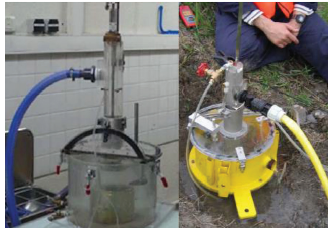
FIGURE 69 Jet erosion test (Hanson and Cook 2004).
