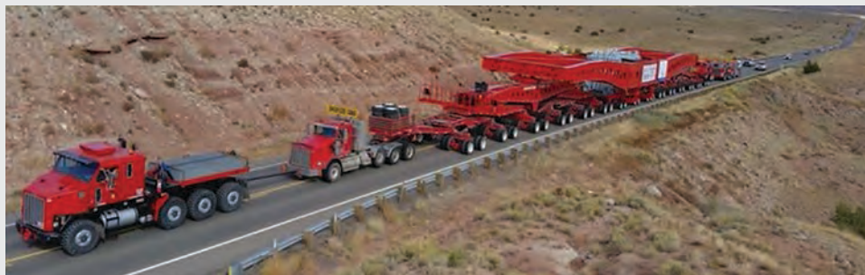
Megaload using dual lane loading, trunnion axles, and push trucks.
