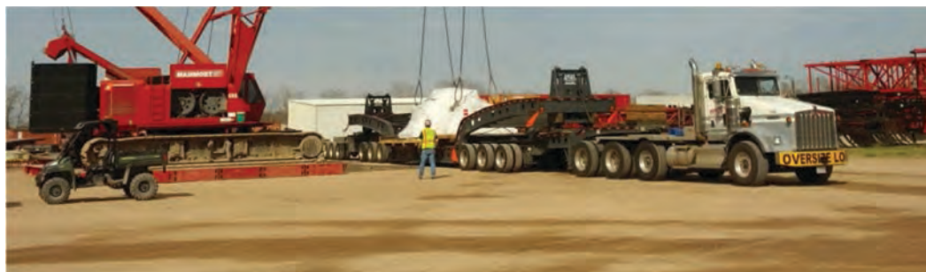
Figure 3-13. 13-axle configuration of Move 3.
