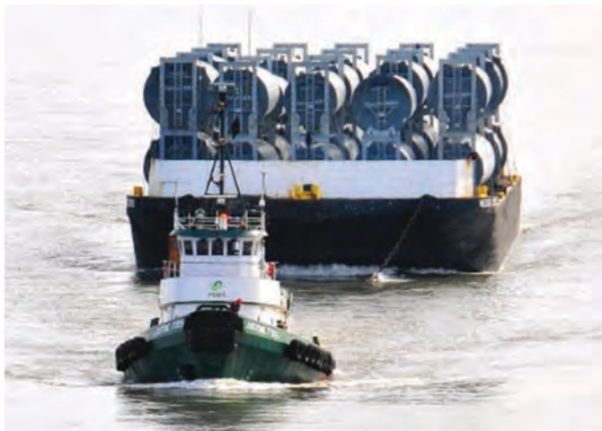
Figure 4-9. Barge transportation of wind tower bases.
