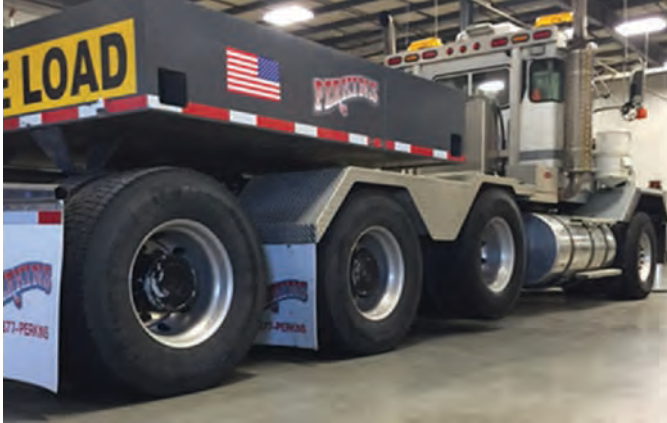
Figure A-49. Truck with lift axle in up position.
