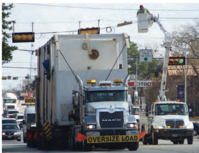
Figure 4-5. Lift truck used to raise a traffic signal.
