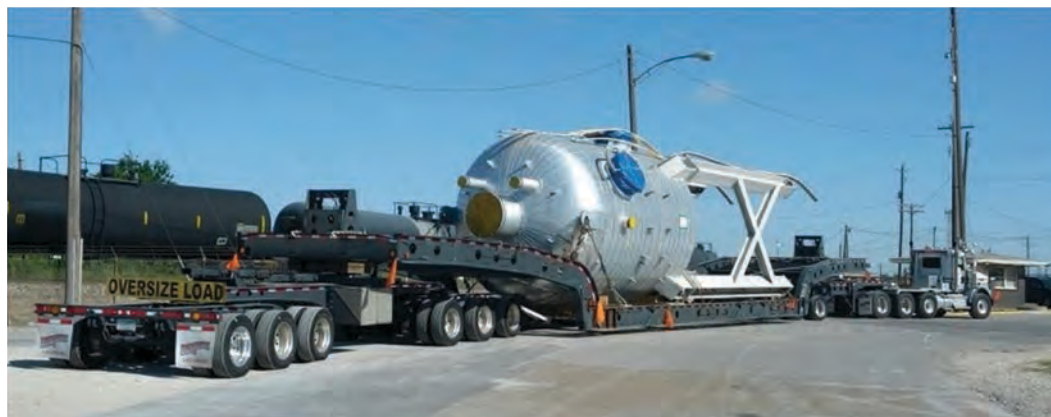
Figure 3-8. Cornering with a rear steer in Move 2.
