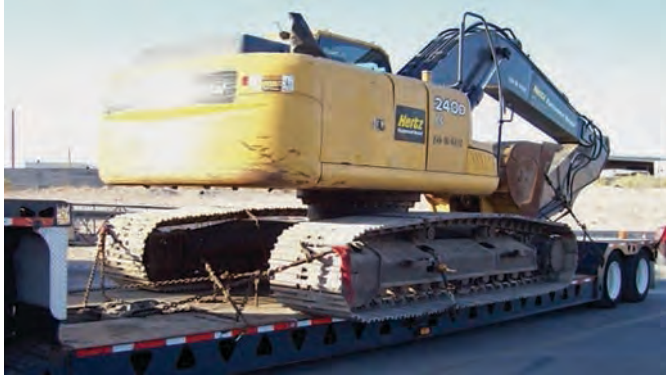
Figure A-1. Excavator on a removable gooseneck tandem axle trailer.
