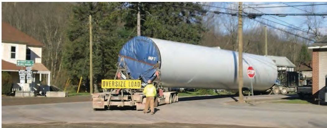
Figure A-40. OSOW load cornering a two-lane roadway.
