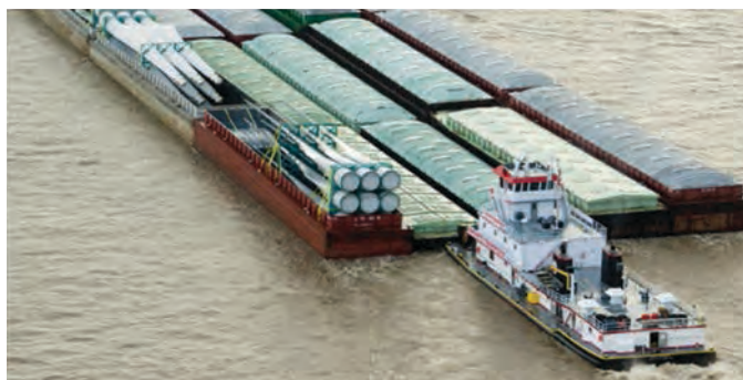
Figure 4-3. Wind tower blades moving with covered hopper barges.
