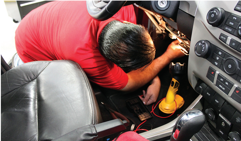
An installer equips an NDS car in Buffalo, New York, with instrumentation for recording acceleration, braking, speed, and other data.
