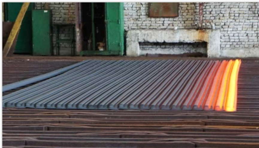
FIGURE 3 Block rail cooling after rolling.
