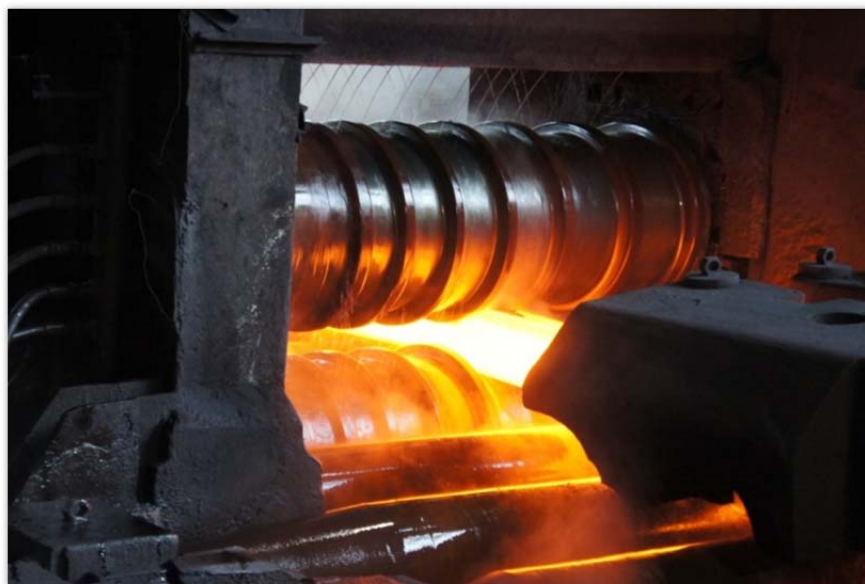
FIGURE 2 Block rail being rolled.
