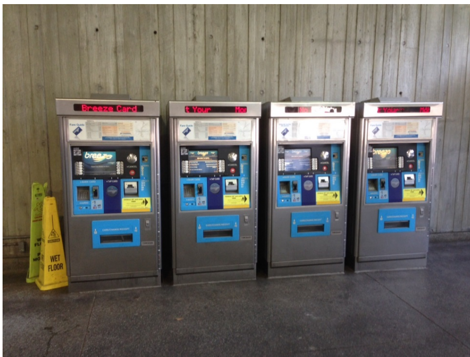
FIGURE 4 Four Breeze ticket vending machines in MARTA Midtown Station. The same equipment is used for heavy rail and streetcar tickets.
