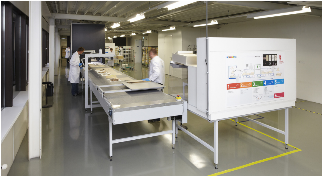
FIGURE 3.11 A Rapid Capture Digitization System with a Conveyor Belt Developed by Picturae
