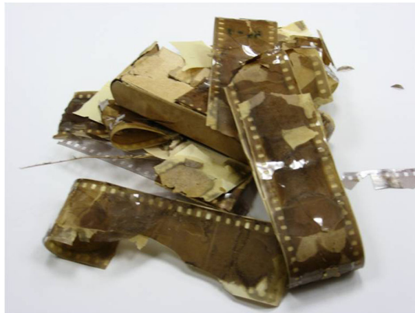
FIGURE 4.3 Deteriorated Acetate Film
