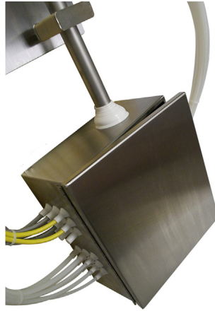
FIGURE 6.62 The electric cabinet is mounted at 30–45 degrees, preventing debris or liquids from accumulating on the top surface. The gaps formed by electric cables entering or leaving the enclosure can be closed by means of plastic caps. However, in this example, liquid tightness is not completely guaranteed. Courtesy of Central States Industrial, www.pipetite.us .
