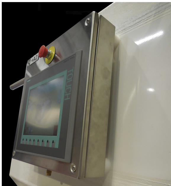
FIGURE 6.78 Touchscreen display installed inclined. Courtesy of OctoFrost Group; Frank Moerman, ©2016.
