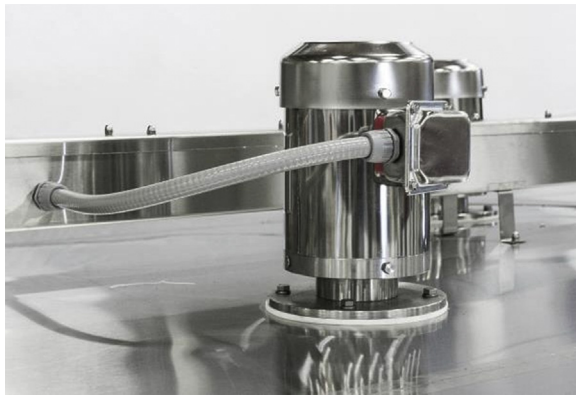
FIGURE 6.54 Wash-down motor. However, it is preferable to avoid hosing of motors, outlets, and electrical cables. The electrical connection to the motor should be waterproof and the cable gland of the motor should be positioned in a direction pointing away from the food contact zone and away from direct spraying when cleaning. Courtesy of CES NV.
