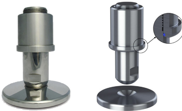
FIGURE 6.30 Heavy-duty adjustable feet with the threaded spindle completely covered by a sleeve provided with O-rings. By adhering to the smooth surface of the screw, this gasket prohibits any intrusion of dirt. Where required, the spindle can be welded to the footplate to avoid liquids or product residues from gathering in the hole in the footplate. Photo left, courtesy of Martin S.R.L., photo right, courtesy of NGI A/S.
