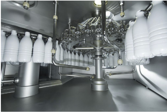
FIGURE 6.7 Equipment surfaces in the product zone must be self-draining, and internal angles and corners well radiused. Courtesy of Kronos AG.
