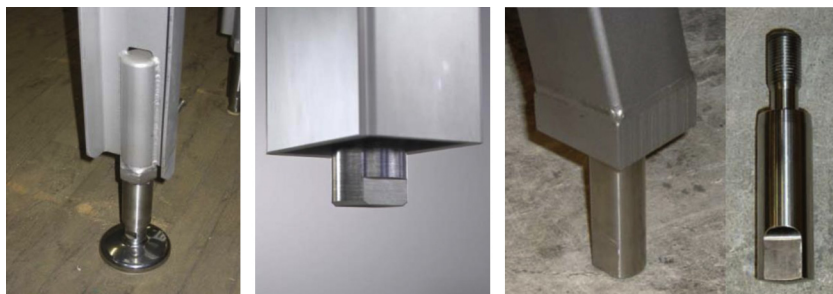
FIGURE 6.34 Adjustable feet with the threaded spindle completely concealed in closed profiles/pipes. In the first example (photo on the left), the thread of the foot is covered by the closed pipe, welded in a sheet metal leg (courtesy of Den Rustfri Stålindustri Kompetencecenter ). In the second example (photo in the middle), the foot can be screwed in and out at the bottom of the frame's legs (courtesy of Alfa-Laval AB ), while the thread still remains covered in the leg. In the third example (photo right), the leveling foot is screwed in leveling foot mount (courtesy of Schenck Process LLC ). In the second and third examples, the contact surface of the feet with the floor is rather small, which will locally exert a (very) high pressure, especially if used to support heavy equipment prone to vibration/oscillatory movement.
