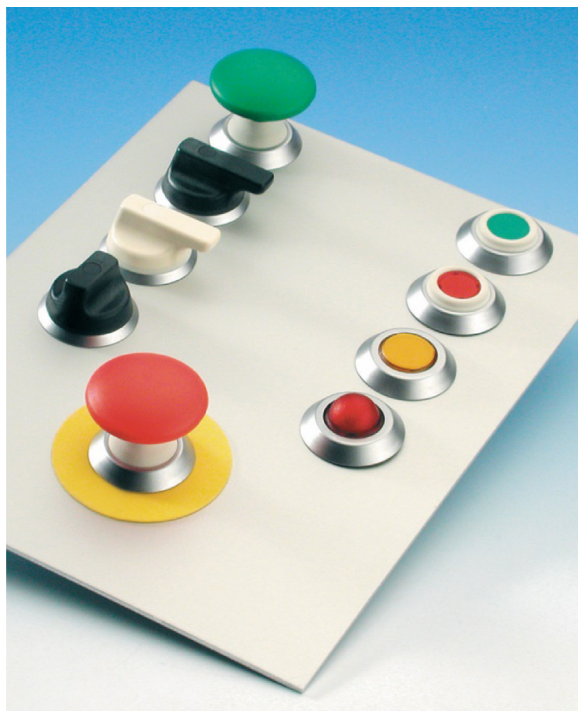
FIGURE 6.75 Control panel with hygienic control and indicator devices. An IP67 or IP67K ingress protection rating for control panel enclosures is highly recommended. Courtesy of K.A. Schmersal GmbH & Co. KG.
