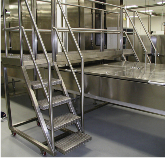
FIGURE 6.56 Products transported by a conveyor belt are protected from the environment by means of covers provided with “D” handles at their sides. Courtesy of Bay State Industrial Welding & Fabrication, Inc.
