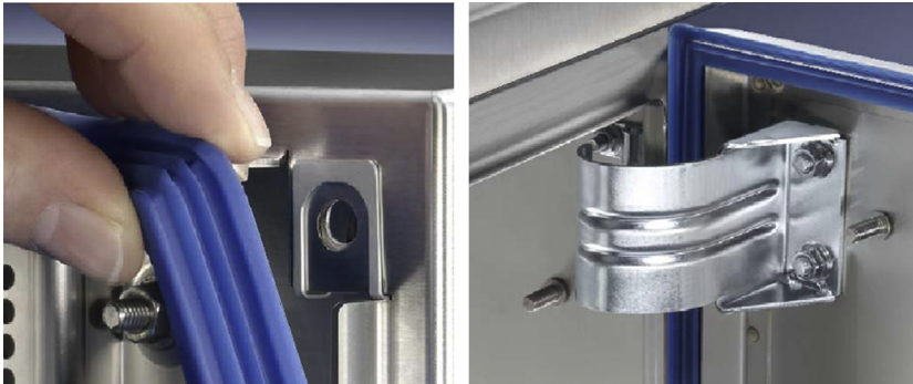
FIGURE 6.65 Seal with folded lip along the top inside edge of the door should be of a removable type, and hinges installed inside the sealing zone create an easy-clean design on the outside. Courtesy of Rittal GmbH & Co. KG.
