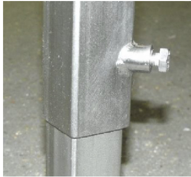
FIGURE 6.4 Penetration of hollow sections of equipment such as frames with bolts is not allowed. Hollow sections shall be hermetically sealed (Kold et al., 2016).
