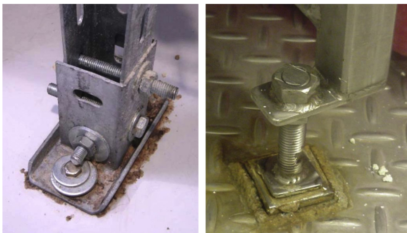
FIGURE 6.24 The foot has plenty of pits, folds and other imperfections where dirt and liquids may build up. In particular the exposed treads, bolt nuts and washers create a lot of crevices. The footbase forms a difficult-to-drain flat surface, and dirt and water may penetrate under the footplate. In this manner, they form a niche where microorganisms may grow. Photo left, courtesy of Mondelez International, 2016; photo right, American Meat Institute, © 2016.
