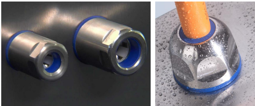
FIGURE 6.67 Hygiene compatible cable glands with seal (blue) directly at the cable entry. The outside of the gland has minimum radii on the hexagon. The connection does not leave an external thread. Due to the presence of a seal with square cross section, the termination between the cap nuts and the enclosure is flush. Photo left: courtesy of Rittal GmbH & Co. KG; photo right: courtesy of Pflitsch GmbH & Co. KG.
