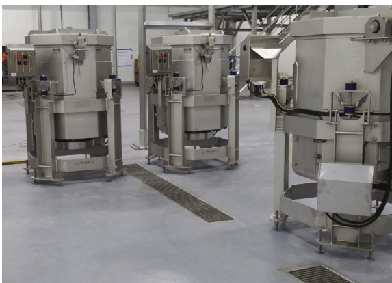
FIGURE 6.21 Channelized frame construction eliminating hollow tubes and threaded leg adjusters. Courtesy of Rudi Groppe, Heizen Manufacturing International, © 2016.
