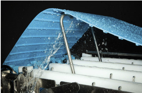
FIGURE 6.9 Belt lifting device used to provide improved access for cleaning and disinfection of the conveyor bed (frame and wear strips), as well as the bottom side of the conveyor belt. Courtesy of Intralox.
