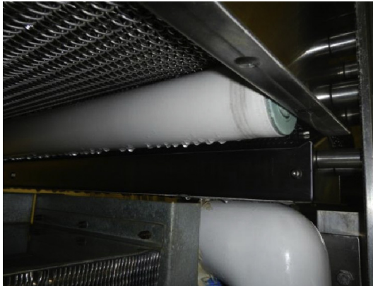
FIGURE 6.50 Hollow rollers and pulleys shall not be used. Courtesy of General Mills.
