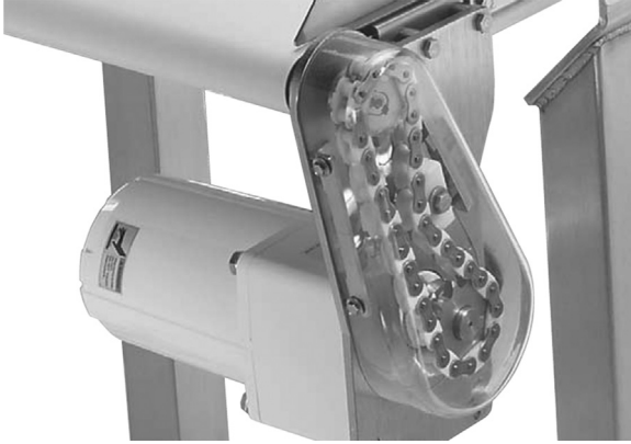
FIGURE 6.47 The drive motor is located below the line of the product flow. Gears, chains (stainless steel or polyacetal), and motors of belt drives must be covered to avoid any contamination of product. However, a chain guard (essential from an occupational safety point of view), when open, may provide a place where product may accumulate, allowing microbes to multiply to large numbers and so posing a contamination risk for the food product on the belt. A transparent chain guard may allow detection of any product debris inside the chain guard. Courtesy of Dorner Mfg. Corp.
