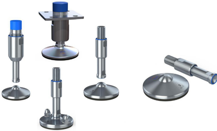
FIGURE 6.31 Hygienic adjustable equipment feet admitting slopes up to 15 degrees on floors. Footbase plate and spindle are two separate entities. The concave end of the spindle fits in a diametrically centered elevation of the footbase plate, having the form of a spherical dome. An O-ring fitted in the concave spindle end must prevent access of impurities, filth or bacteria in the joint. The adjustment sleeve covers the threaded surface, and at the same time functions as a nut. The O-rings inserted inside the adjustment sleeve adhere tightly to the smooth surface of the screw, and prevent dirt from entering the thread section. Courtesy of NGI A/S.
