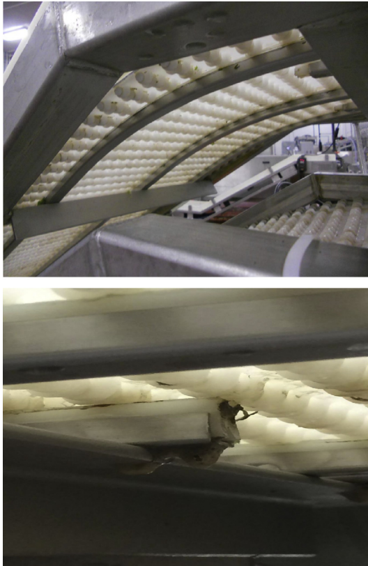
FIGURE 6.8 Despite their general acceptance over the last two decades and their mechanical versatility, modular belts, relying as they do on hinges and pins, are difficult to clean. Especially, the pinholes in the hinges and pins are major dirt and bacteria traps. Hence, all parts of modular conveyor belts at the running side shall be readily accessible for inspection so as to facilitate the detection of all potential contaminants, as well as cleaning procedures.
