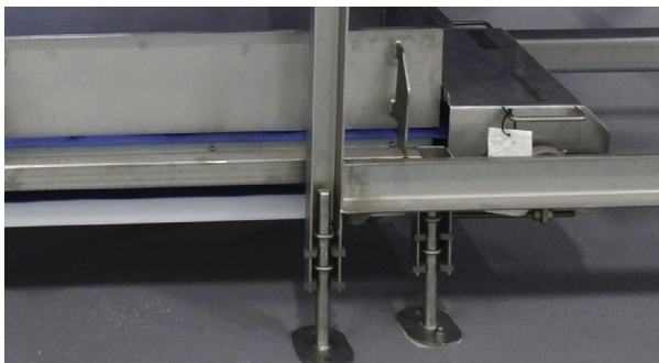
FIGURE 6.40 Threadless adjustable feet hygienically fixed onto open profile legs. Courtesy of Rudi Groppe, Heinzen Manufacturing International, © 2016 .
