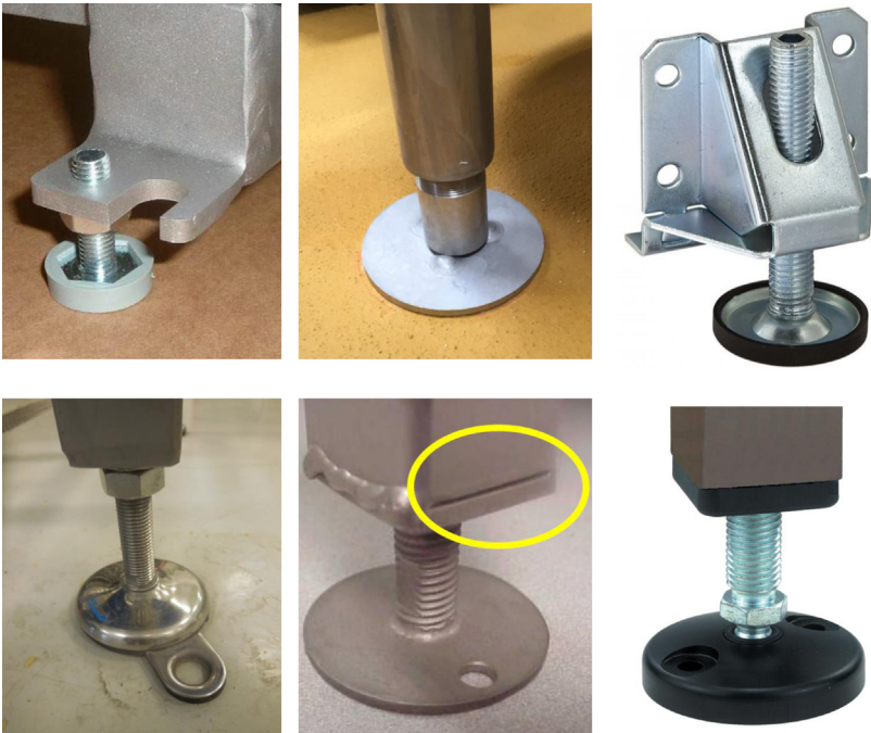
FIGURE 6.33 Adjustable feet with exposed threaded spindle easily become prone to contamination and are difficult to clean. Lower middle photo shows a hollow leg which is not hermetically closed. Photo at lower center courtesy of Joe Stout, Commercial Food Sanitation LLC - Intralox, © 2016.
