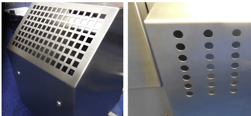
FIGURE 6.59 Punched stainless steel guards with 40/50% open area maximum. They must be opened for cleaning the inside. Frank Moerman, © 2016.
