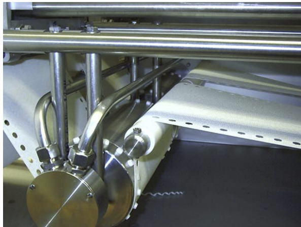
FIGURE 6.71 Cables can be protected from dirt layering and damage by encapsulating them in hermetically closed cable housings such as stainless steel pipes, especially in the neighborhood of the food contact and splash area (Den Rustfri Stålindustri Kompetencecenter, 2006).
