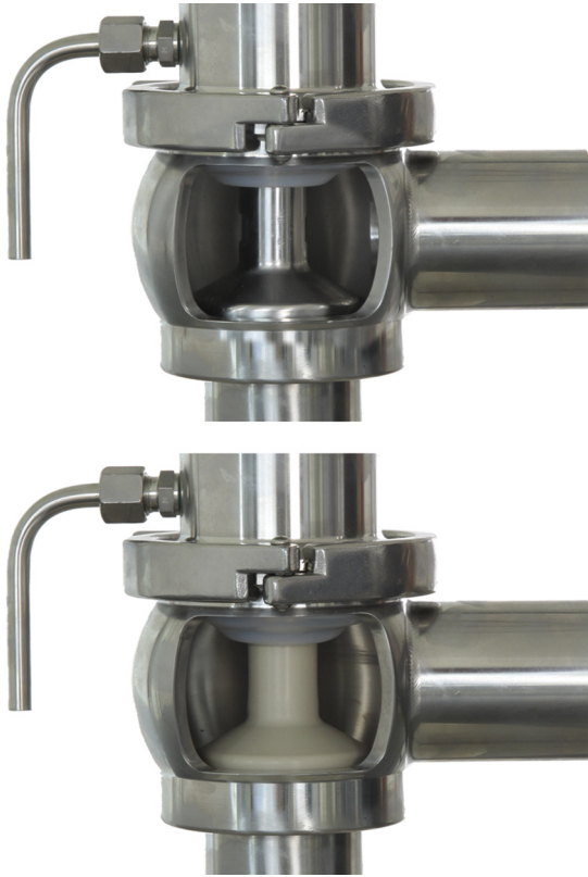
FIGURE 7.60 Linear plug and stem valves where a PTFE diaphragm with superior mechanical characteristics provides hermetic protection of the spindle travel during aseptic applications. Contrary to bellow sealed linear plug and stem valves, this valve is suitable for process operations handling liquid food with abrasive particles or products that crystallize in the atmosphere, such as lactose or instant coffee. Courtesy of Pentair Süidmo GmbH.
