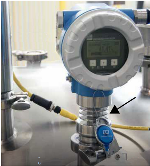
FIGURE 7.78 Changes in ambient temperature around the measurement system due to high process/utility temperatures can be minimized by means of a cooling element mounted between the gauge and the hot process/utility system. Courtesy of Endress + Hauser AG.
