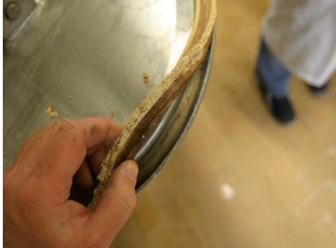
FIGURE 7.12 Seals for mandoor covers must be of a removable type to allow for inspection, cleaning and replacement. Food debris may accumulate under the seal, providing nutrients for microorganisms. Courtesy of Burggraaf & Partners B.V.
