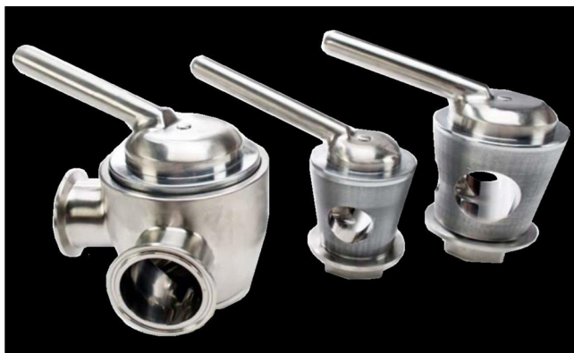
FIGURE 7.63 Plug cock valves are unsuitable to be cleaned in-place, because product can get caught around the clearance between the plug and the valve body during rotation of the plug in the turned-off position. But, as they are easy to dismantle, they can be cleaned manually. Courtesy of Sanitary Solutions, Inc.
