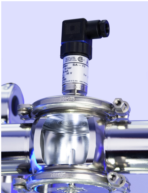
FIGURE 7.83 A pressure transmitter with tubular membranes, having the same inner diameter as the adjacent pipeline, can be easily integrated into the process line. Installation usually occurs by means of a clamp fitting, in a standard spherical valve body welded into the piping. The stainless steel diaphragm is sealed by O-rings fitted into grooves so that there is no metal-to-metal joint on the product side. This way of mounting of pressure transmitters provides a dead space-free, flush transition from the process line to the pressure transmitter. At the bottom side a temperature measurement device is installed, again by means of a clamp fitting. Courtesy of WIKA Alexander Wiegand SE & Co. KG.
