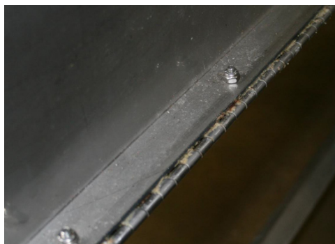
FIGURE 7.10 The piano hinge prohibits removal of the cover, and allows food residues to accumulate in the hinge. In the piano, microorganisms may find a niche to grow (Don Graham, Graham Sanitary Design Consulting LCC, ©2010).
