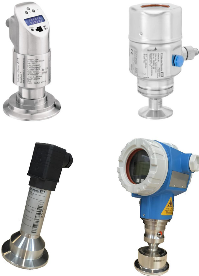
FIGURE 7.77 Hygienically designed electronic pressure measurement devices with stainless steel or plastic housing. The external housing and wiring may not collect dust or soil, requiring a design with smooth transitions and free from pockets. To be self-draining the instrument housing can be made with a sloped top surface, although it is possible to install pressure measurement devices with angles of more than 30 degrees from the vertical. Courtesy of Endress + Hauser AG.
