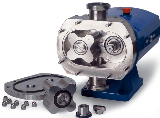
FIGURE 7.46 Nowadays there are hygienically well-designed rotary lobe pumps available with the ports arranged in the vertical plane. Slots in the rotor retaining nuts create turbulences in the flow passing the narrow gap between end cover and lobes. They provide enhanced cleanability of the end cover and the front surfaces of the lobes. Courtesy of Alfa Laval AB.
