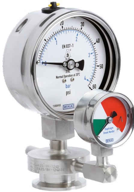
FIGURE 7.91 Diaphragm monitoring system. With regular on-site inspection, a pressure gauge with green-red display will be sufficient to detect failure of the diaphragm in contact with the process. When the pointer goes in the red (right corner of the diaphragm monitoring device), the operator knows that the diaphragm in contact with the process is broken. Courtesy of WIKA Alexander Wiegand SE & Co. KG.
