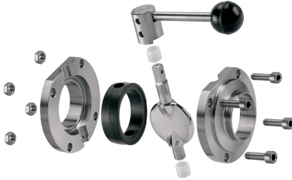
FIGURE 7.54 Butterfly valve having a highly polished stainless steel disc with a surface roughness R_a \leq 0.8 \mu\text{m} . The bearing bushes are clipped onto the disc stems, avoiding any metal-to-metal abrasion and ensuring smoother disc movement. The rubber seal clamped between the halves of the body provides both a seat for the disc to close on and a seal for the disc spindles. However, as they are not hermetically sealed, they are not suitable for aseptic duties. Courtesy of Alfa Laval AB.
