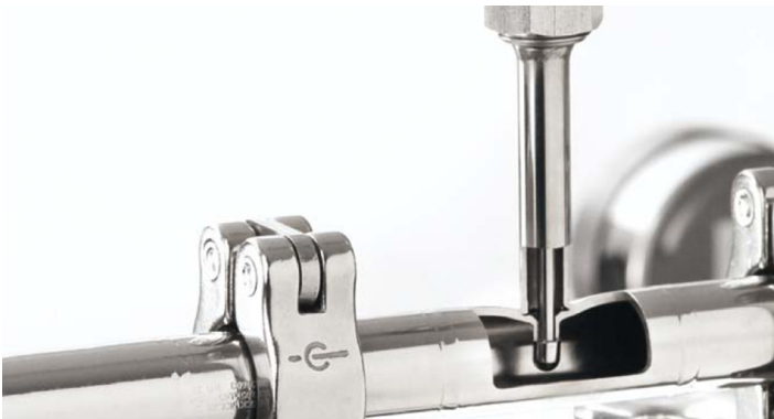
FIGURE 7.95 This flow-through thermowell is directly orbitally welded into the pipeline. The measuring insert can be withdrawn from the thermowell to calibrate the thermometer on-site. Courtesy of WIKA Alexander Wiegand SE & Co. KG.
