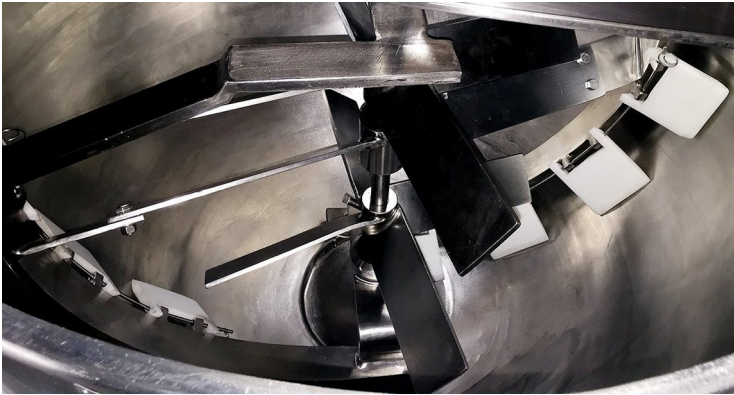
FIGURE 7.20 This agitator may cause hygiene problems because of the bolts and plastic scrapers. Cases are known where plastic scrapers were broken and pieces lost in the product as a foreign body contaminant.
