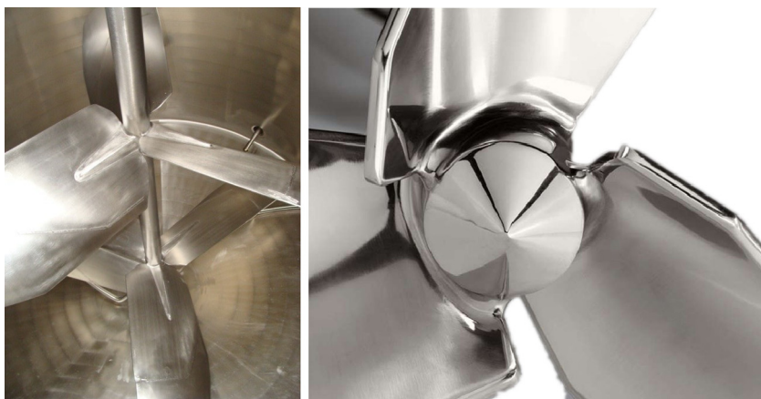
FIGURE 7.19 All-welded impeller assembly (e.g., hubs, blades, end cap). The agitator paddle blades being attached to the shaft by welding must have their welds ground and polished. Photo right, courtesy of Intechwell/Alfa Laval AB.
