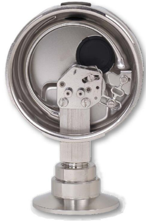
FIGURE 7.88 Mechanical gauges in particular, such as the bourdon gauge, require a diaphragm seal. Diaphragm seal gauges can cope with a greater range of process temperatures and aggressive products. Courtesy of WIKA Alexander Wiegand SE & Co. KG.
