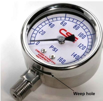
FIGURE 7.76 Weep holes can be provided in the bottom of the vacuum gauge case to ensure proper drainage of condensate, cleaning solutions, etc.
