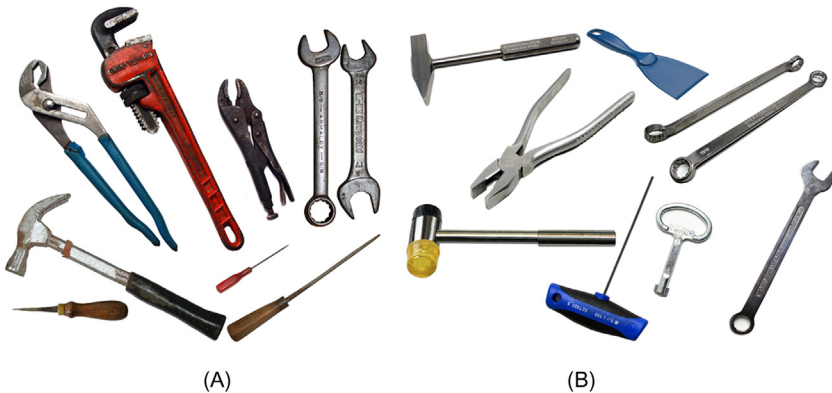
FIGURE 8.43 (A) The maintenance tools suffer from corrosion, are painted (paint may peel off), contain niches and threads; have wooden handles or knurling soft rubber grips; or the tool heads may damage the stainless-steel surfaces of equipment and components. (B) These maintenance tools are made of stainless steel (noncorrosive), easy to inspect, clean, and disinfect, with smooth finish and hard plastic grips, and with fitted heads for equipment longevity. A system of color coding allows maintenance tools to be dedicated for use in specific zones, such as low, medium, or high hygiene areas. Courtesy of John Butts, Land O’Frost; courtesy of Steritool (Frank Moerman, © 2016).
