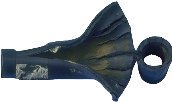
FIGURE 8.7 Inside of a leaking hose, revealing the presence of many cracks which are quite common after a long period of service in contact with liquid food and aggressive cleaning/disinfecting solutions. ( Frank Moerman, © 2016. )
