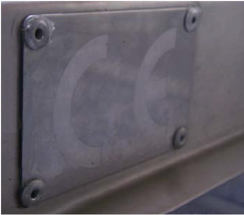
FIGURE 8.26 The name plate is fastened with pop rivets. The small holes may accumulate dirt and become a niche for microorganisms to grow. Food debris, dirt, liquids, and microorganisms also may find their way behind the name plate. Courtesy of Mondelēz International, © 2016.
