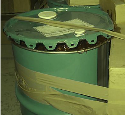
FIGURE 8.9 A clearly damaged grease container on arrival in the factory site. This grease should not be used because it will no longer meet the requirements of a food-safe product (Steenard et al., 2009).
