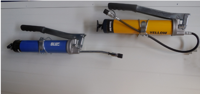
FIGURE 8.34 Color coding of lubrication tools prevents cross-contamination and misapplication of lubricants. Courtesy of Enluse B.V. (Frank Moerman, © 2016).
