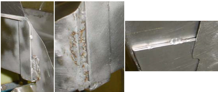
FIGURE 8.20 Noncontinuous welding of overlapping sheets of metal allow product debris and microorganisms to accumulate between the two sheets of metal. The overlapping sheets of metal also create a step. Courtesy of John Butts, Land O'Frost, © 2016.
