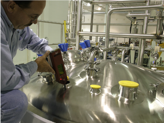
FIGURE 8.13 Quality technician doing Positive Material Identification on a stainless-steel vessel using an X-ray fluorescence gun. Courtesy of Holland Applied Technologies.
