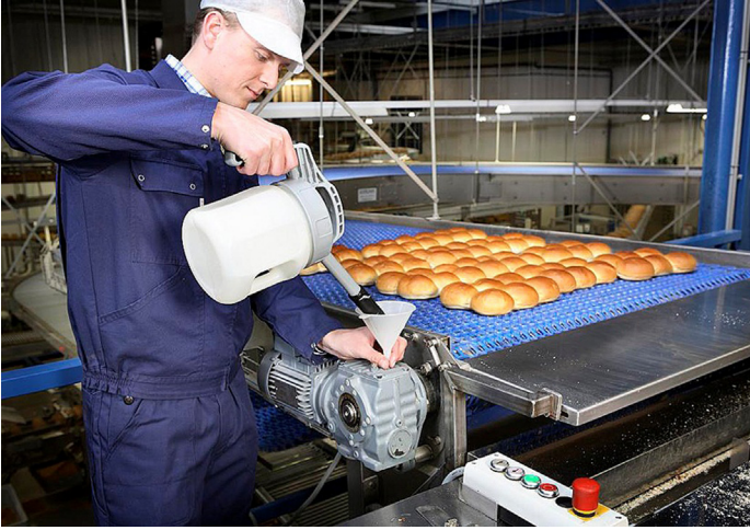
FIGURE 8.36 The equipment should be filled carefully with a clean can and a clean funnel (Steenard et al., 2009). Courtesy of Van Meeuwen Lubrication B.V.
