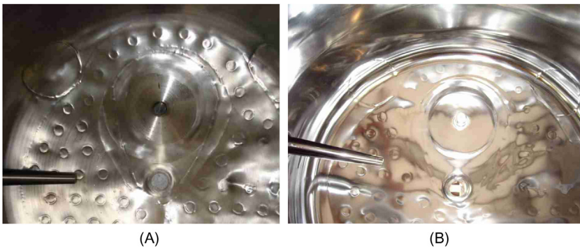
FIGURE 8.32 Remediation of poor “factory” electro-polished equipment: (A) before mechanical and electro-polishing; (B) after mechanical and electro-polishing. Courtesy of Ultraclean Electropolish Inc.
