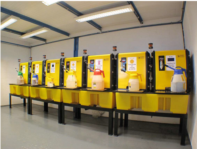
FIGURE 8.39 A correct storage facility helps to prevent contamination. Here, the food-grade lubricants are stored off the floor and in clearly labeled containers (Steenard et al., 2009) (Courtesy of Enluse B.V.). Courtesy of Van Meeuwen Lubrication B.V.
