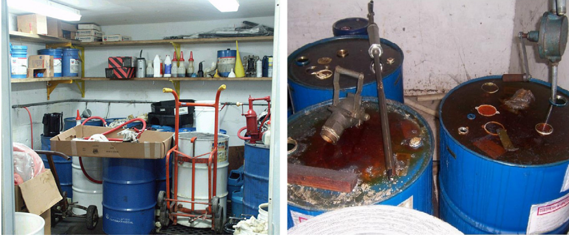
FIGURE 8.38 Incorrect storage: contamination and use of incorrect lubricants can easily occur (Steenard et al., 2009).
