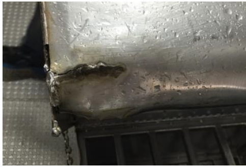
FIGURE 8.19 Poor weld repair. Courtesy of Joe Stout, Commercial Food Sanitation LLC - Intralox, © 2016.
