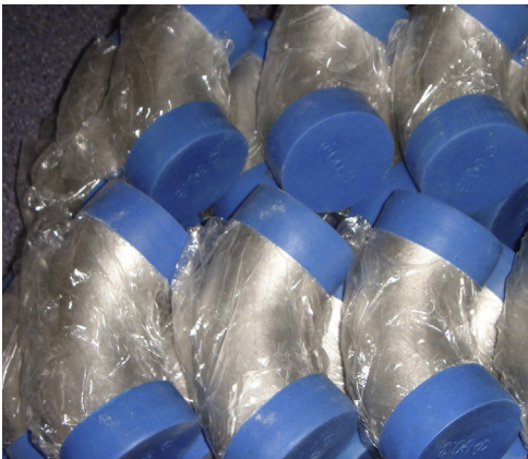
FIGURE 8.17 The stainless-steel equipment components are wrapped with plastic film, and their inlet and outlet connections are fitted with protective caps to protect them against corrosion, dirt, pests, etc. during transport and storage. Courtesy of Zhejiang Jugang Pipe Co, Ltd.
