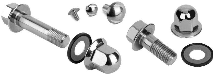
FIGURE 8.24 Hexagon-headed bolts with plain bolt head are accepted, although hygienic bolts with domed bolt head are more preferred. The thread of the bolts can be covered with a hexagonal domed nut. Metal-backed elastomer gaskets may seal the crevice between the bolt-head or domed nut and the food-contact surface. Courtesy of NovoNox KG.
