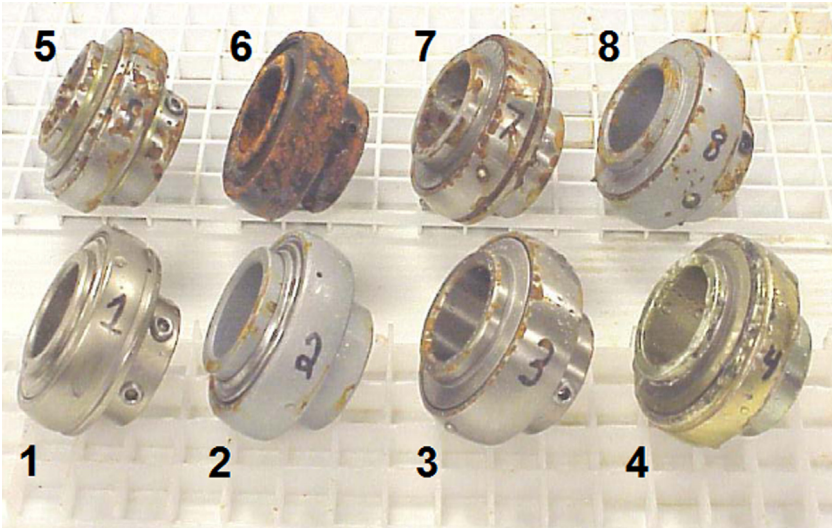
FIGURE 8.11 Bearings made from different materials of construction were subjected to immersion tests in salt brine. Bearings No. 1, 2 and 8 are thin dense chrome plated; bearings No. 3, 5, and 7 are 400 series stainless steel; bearing No. 4 is coated; and bearing No. 6 is black oxide coated. Courtesy of John Butts, Land O'Frost, © 2016.
