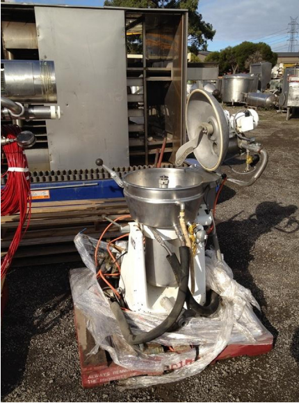
FIGURE 8.50 Decommissioned or idle equipment must be stored in an appropriate way to ensure it does not become a source of contaminants or harbor pests. When stored outdoors, it should be placed on a hard standing (e.g., concrete, sealed, or paved area) and covered, which is not the case in this example. Moreover, the equipment is not appropriately covered.
