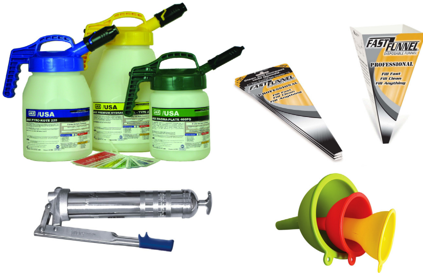
FIGURE 8.35 Dedicated lubrication equipment should be used for lubrication and greasing. In high-hygiene areas, the use of a stainless-steel grease gun and disposable funnels is recommended. Color coding of funnels and dispensing drums prevents cross-contamination and misapplication of lubricants. This color coding also may assign lubrication tools to a specific hygiene area. Additionally, color-coded labeling of all lubrication points will further prevent mixing of lubricants (e.g., food-grade and non – food-grade lubricants). Courtesy of Justrite Manufacturing Company, L.L.C.; courtesy of S & S Concepts Inc.; courtesy of KitchenWerks.
