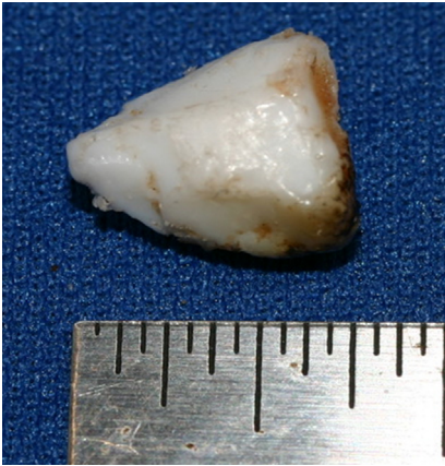
FIGURE 8.1 Small piece of a damaged scraper found in a failed pump. Courtesy of Joe Stout, Commercial Food Sanitation LLC - Intralox, © 2016.
