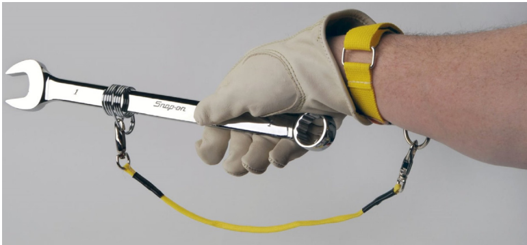
FIGURE 8.44 Although the tool is secured, the lanyard gives technicians unrestricted tool use and doesn't impede mobility or compromise personal safety equipment. Courtesy of Snap-on Industrial.
