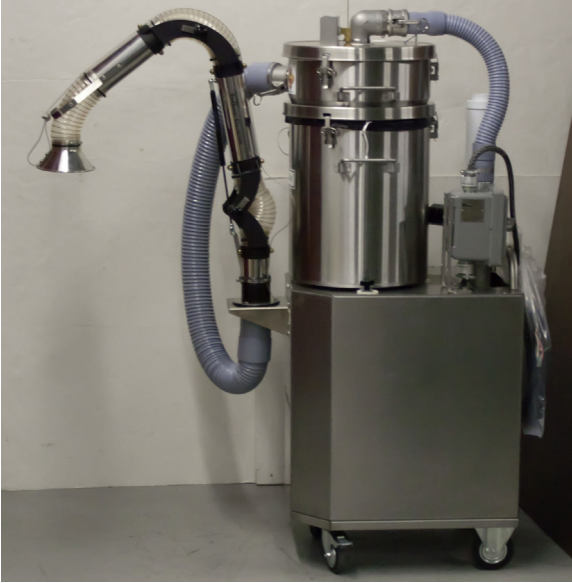
FIGURE 8.47 Vacuum cleaners should be applied to extract maintenance debris at the place where the maintenance takes place.
