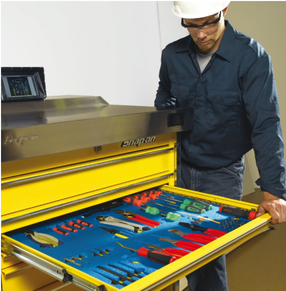
FIGURE 8.48 Tool containers with foam cutouts may support technicians in tool accountability. When tools are returned at the end of a project, any open space alerts the technician of a potentially missing tool. Courtesy of Snap-on Industrial.
