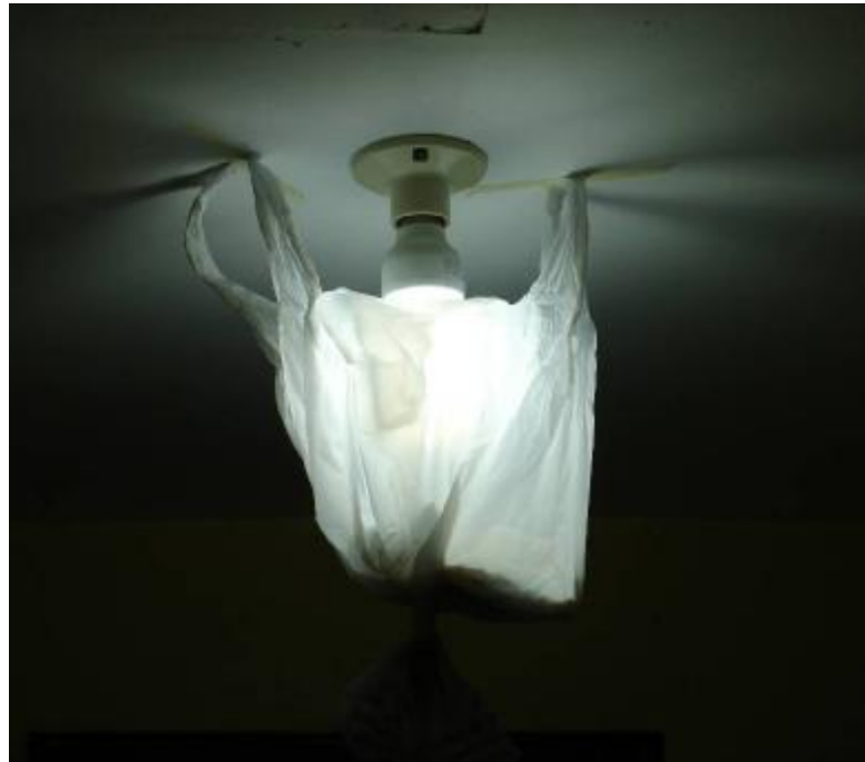
Figure 3 – Makeshift incubator for Petri Plates
