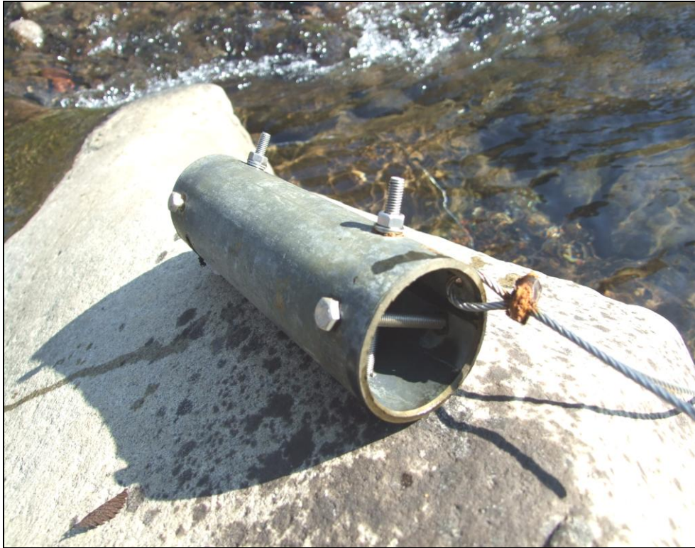
Figure 2.7 Dallas® Thermochron i-buttons protected by a 20cm section of water piping
