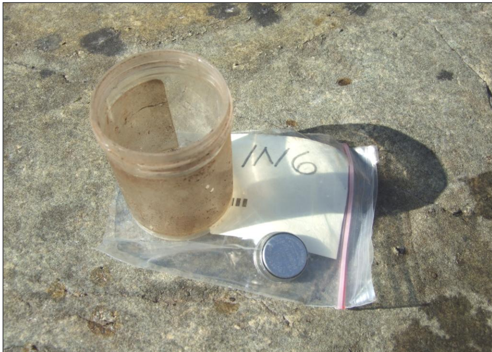
Figure 2.6 Dallas® ThermoChron i-button programmed to measure daily water temperature in 90 minute intervals
