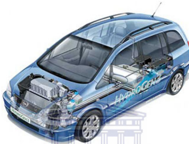
Figure 2.2 HydroGen3, a fuel cell car developed by Adam Opel AG, is propelled by a fuel cell stack consisting of 200 individual PEM fuel cells connected in series [6]
