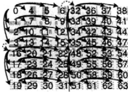
Figure 4.5: The ordering 2D 8 \times 8 WHT for fast KHT algorithm. Numbers denote the order. Solid arrows denote the computation dependence using the KHT algorithm while dashed arrows denote the computation dependence using the GCK algorithm. For example, projection values 4, 5 and 6 are computed from 0 by the KHT algorithm while 32 is computed from 6 by the GCK algorithm.
