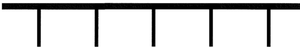
Figure 2-11: Slow-wave structure based upon capacitive loaded transmission line.
