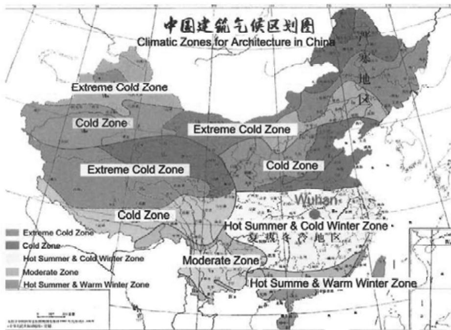
Figure3- 1: Five main climatic zones for building design in China and the location of Wuhan 20
