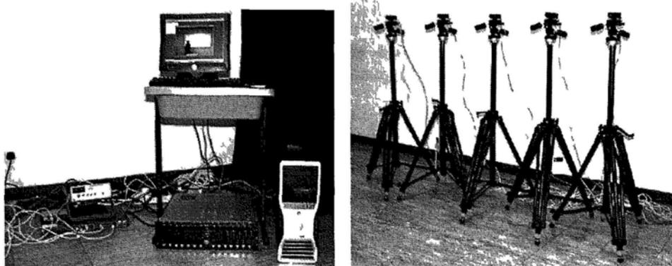
(a) The control units computer, switch, synchronizer and harddisk array (b) Five Prosilica GC650C cameras
