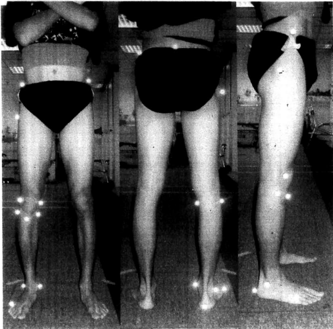
Figure 5.9 Marker set of motion analysis assessment (left to right: anterior view, posterior view and lateral view).
