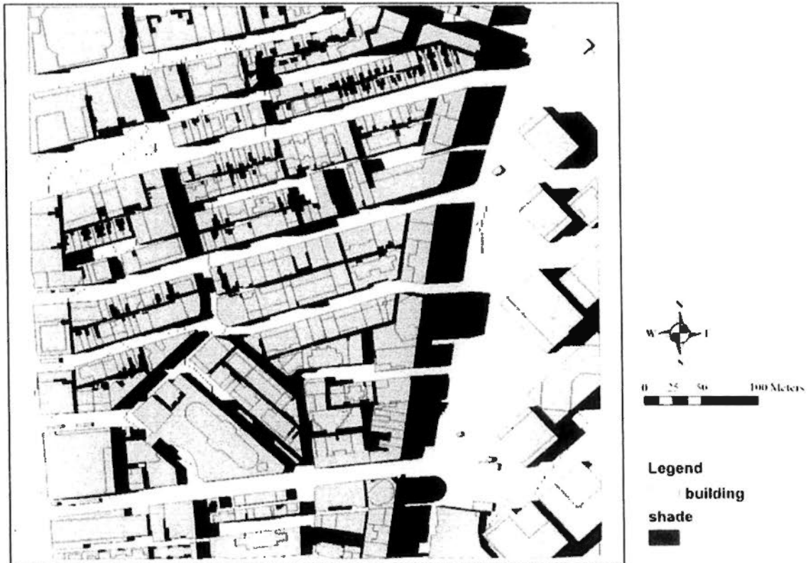
Figure 4.16 Shading map of the study site. The map represents the shade pattern at 14:30 because of the 1 hour time resolution used.
