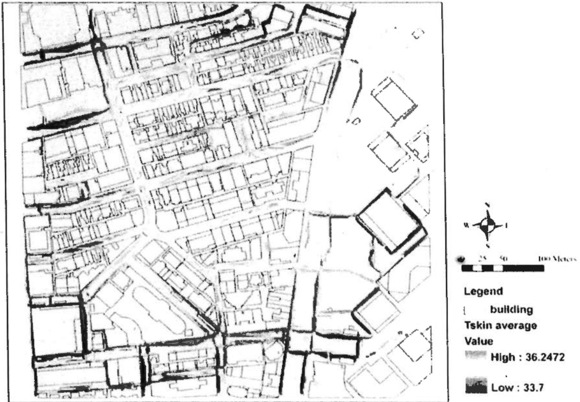
Figure 4.35 Map of the spatial distribution of pedestrians' average skin temperature during the simulation course. Grey color means no data, i.e. the space is not used by pedestrians, e.g. car road or unwalkable space.
