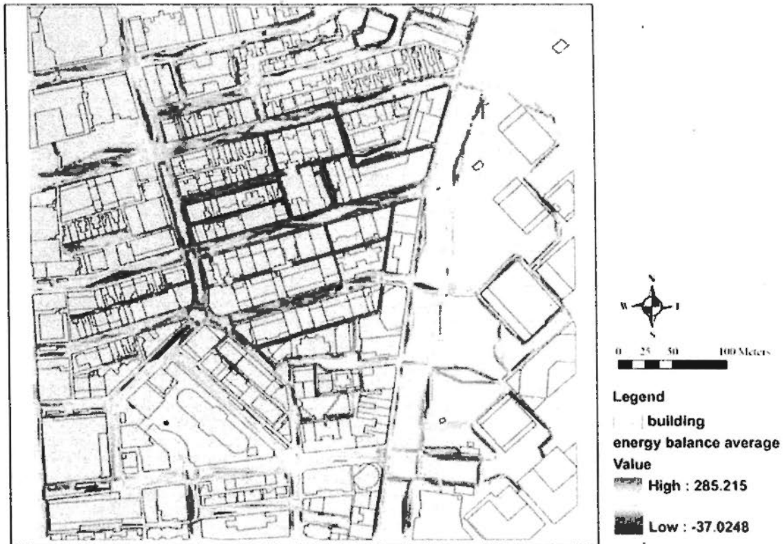
Figure 4.43 Map of the spatial distribution of pedestrians' average energy balance during the simulation course for the modified scenario. Grey color means no data, i.e. the space is not used by pedestrians, e.g. car road or unwalkable space.
