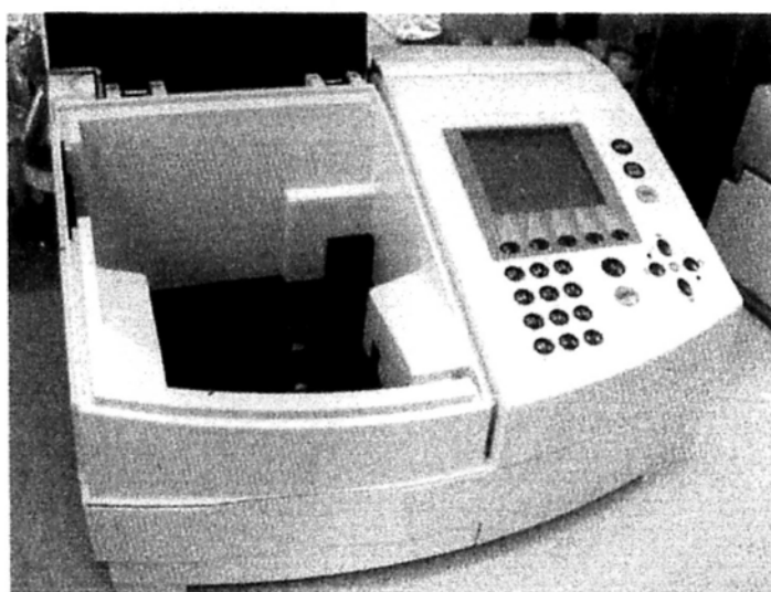
Plate 3.3 A Helios Gamma UV-vis spectrophotometer (Thermo Electron, England).
