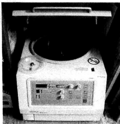
Plate 3.2 A Hermle Z323 centrifuge (Hermle Labortechnik, Germany).
