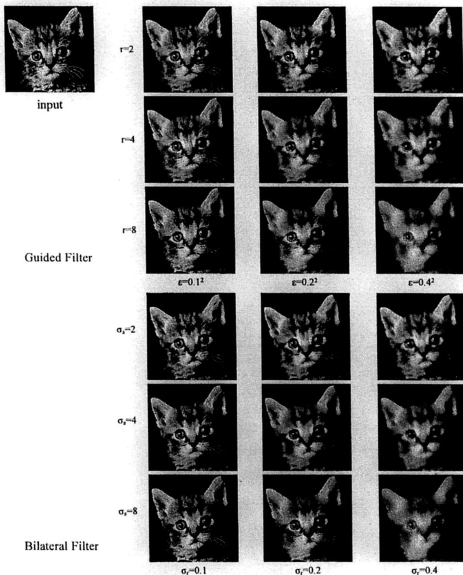
Figure 4.7: Filtered images of a gray-scale input. In this example the guidance  $I$  is identical to the input  $p$ . The input image has intensity in  $[0, 1]$ . The input image is from [80].
