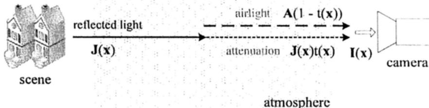
Figure 2.2: A macro physical picture of the haze imaging model.
