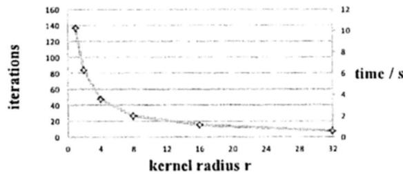
Figure 4.5: Iteration numbers and running time vs. kernel size. The iteration numbers correspond to the error  $1e^{-10}$  in Fig. 4.4.
