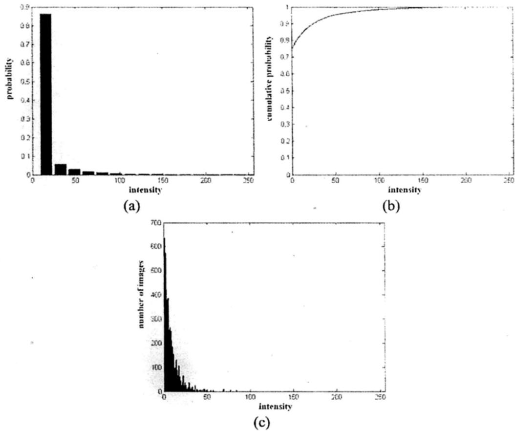
Figure 3.4: Statistics of the dark channels. (a) Distribution of the pixel intensity of all of the 5,000 dark channels (each bin represents 16 intensity levels). (b) Cumulative distribution. (c) Distribution of the average intensity of each dark channel.
