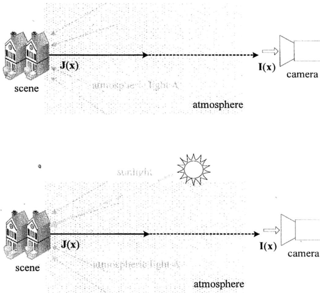
Figure 3.8: Illumination sources in hazy days. Top: The atmospheric light is the sole illumination source. Bottom: the sunlight is another illumination source.
