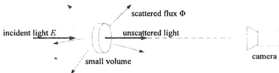
Figure A.2: Scattering model in a small volume of atmosphere.
