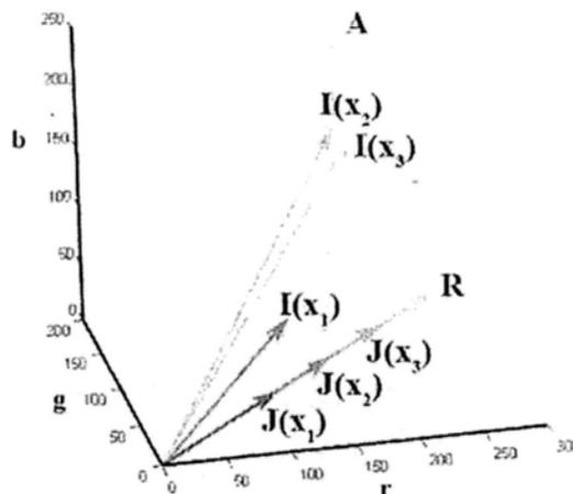
Figure 2.11: The color vectors in the RGB space. Three pixels at  $x_1$ ,  $x_2$ , and  $x_3$  have the same reflectance  $R$ , but different luminance and transmission.
