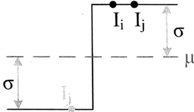
Figure 4.8: 1-D example of an ideal step edge. For a window that exactly center on the edge, the variables  $\mu$  and  $\sigma$  are as indicated.
