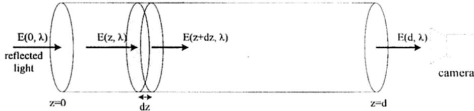
Figure A.3: Light traveling in the atmosphere is attenuated.
