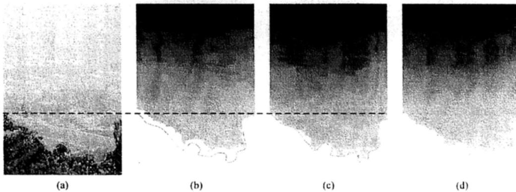
Figure 4.12: Dilation and erosion. (a) Input hazy image. The red curve approximately outlines the profile of the trees. (b) Estimated transmission by (3.14). The trees appear “dilated”. (c) Estimated transmission after erosion (4.53). The profile is more consistent. (d) Guided-filtered result of (c).
