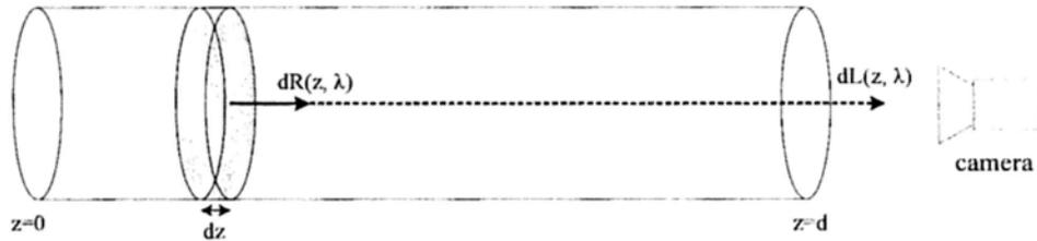
Figure A.5: The radiated light by a volume has to pass through the haze before reaching the observer.
