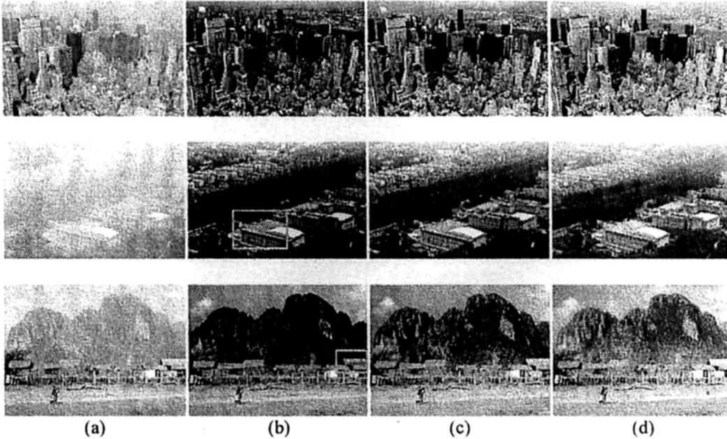
Figure 3.15: Recovering images using different patch sizes (after soft matting). (a): Input hazy images. (b): Using  $3 \times 3$  patches. (c): Using  $15 \times 15$  patches. (d): Using  $30 \times 30$  patches.
