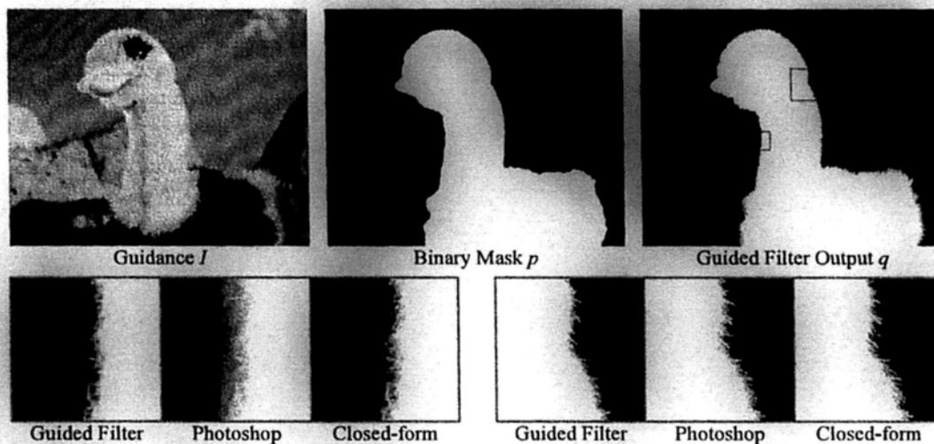
Figure 4.19: Alpha Matting/ Guided Feathering. A binary mask  $p$  is filtered under the guidance of  $I$ . In the zoom-in patches, we compare with the Photoshop Refine Edge function and the closed-form matting. For closed-form matting, we erode and dilate the mask to obtain a trimap. The parameters for the guided filter are  $r = 60$ ,  $\epsilon = 10^{-6}$ .
