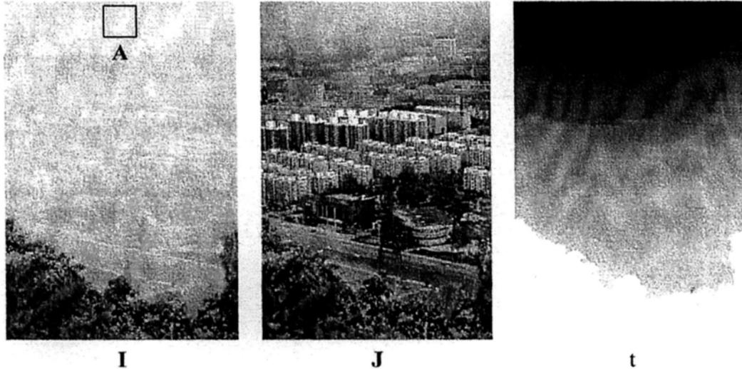
Figure 2.1: Variables in the haze imaging equation. The transmission map  $t$  is shown as white when  $t=1$ , and black when  $t=0$ .
