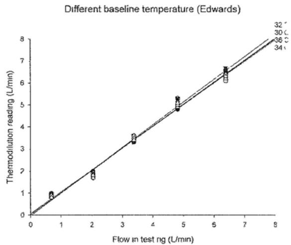
Figure 2.27b. Regression lines showing four different water temperatures using an Edwards catheter. Note that only slight differences in the slopes occurred between the four lines. The gradient of the slopes ranged from 0.99 to 1.03. When X=5L/min, Y ranged from 5.0 to 5.1L/min.
