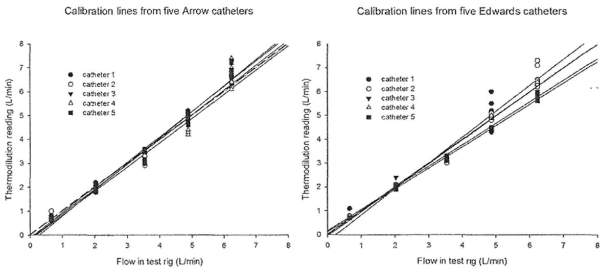
Figure 2.36. Plots comparing the calibration lines for 5 different Arrow catheters (left), and 5 different Edwards catheters (right). Lines constructed from sets of 5 readings taken at
