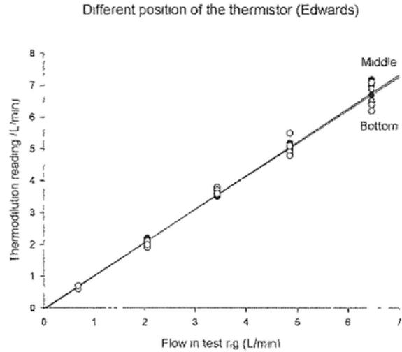
Figure 2.29b. Calibration lines showing different positions of the catheter tip within the lumen of the Edwards catheter. There is only a slight difference between the two lines. The slope ranges were 1.04 and 1.05. When  $X=5\text{L}/\text{min}$ ,  $Y$  ranges from 5.1 to 5.2L/min.
