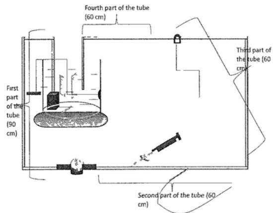
Figure 2.5b. Schematic diagram showing the different sections of the tubing.
