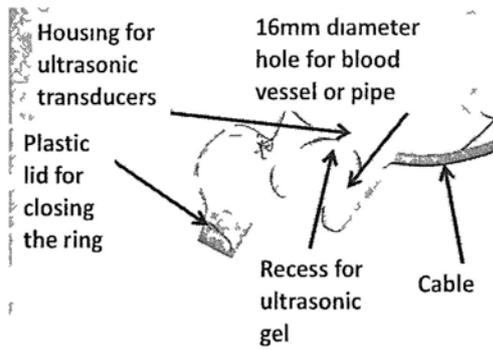
Figure 2.9 Transonic 16A flow probe
