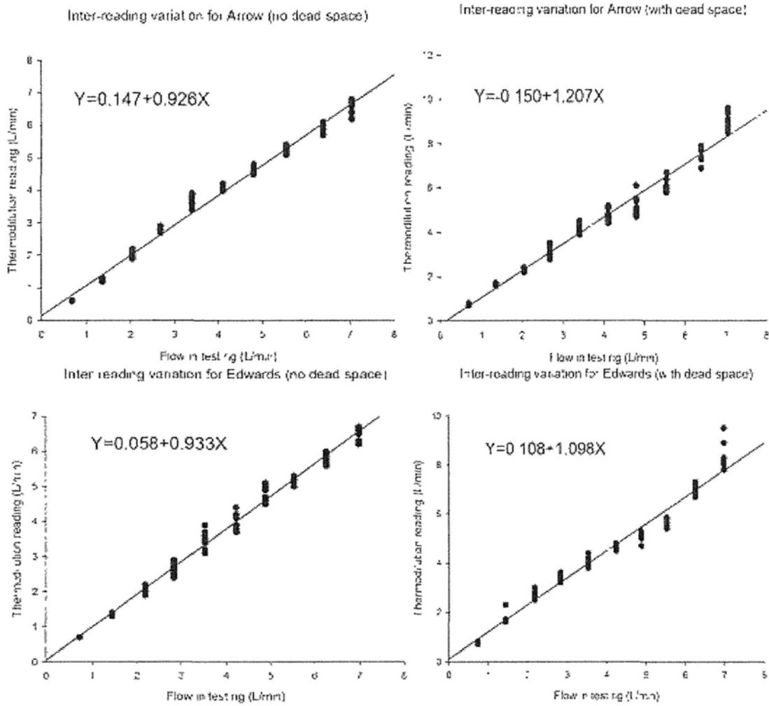
Figure 2.35. Plots showing the inter-reading variability when performing single-bolus thermolution measurements with the Siemens SC9000 cardiac output monitor. Data for Arrow (upper) and Edwards (lower) catheters, without (left) and with (right) catheter dead space. Sets of 10 readings were collected at each flow rate. Note the slightly nonlinear relationship of data to the regression line.
