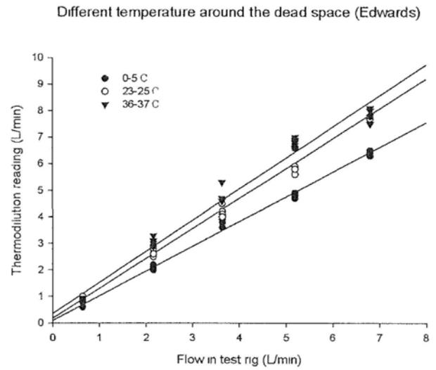
Figure 2.30b. Calibration plot showing the effect of 3 different ambient temperatures applied to the dead space of the Edwards catheter. The slopes ranged from 0.93 to 1.17. When  $X=5L/min$ ,  $Y$  was 4.8, 5.8, and 6.2 for 0-5, 23-25, and 36-37°C respectively.
