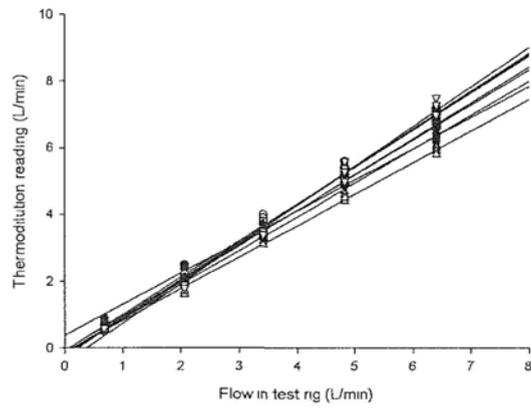
Figure 2.28b. Plot showing the influence of mixing distance when using an Edwards catheter. Slopes ranged from 0.931 to 1.180. When  $X=5\text{L/min}$ ,  $Y$  ranged from 4.6 to 5.5L/min.
