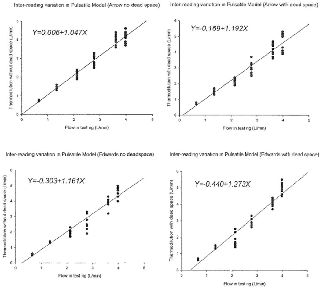
Figure 2.39. Plots showing the inter-reading variability for pulsatile flow when performing single-bolus thermodilution measurements using the Siemens SC9000 cardiac output monitor. Data for Arrow (upper) and Edwards (lower) catheters, without (left) and with (right) catheter dead space. Sets of 10 readings were collected at each flow rate. Note the slightly nonlinear relationship of data to the regression line, most noticeable when using the Edwards catheters.
