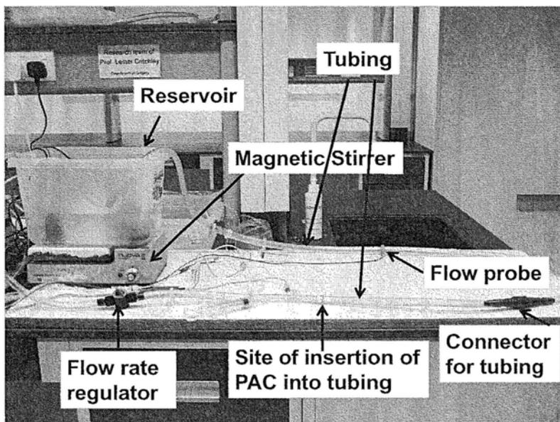
Figure 2.2a. The test rig assembled on a white wooden board and placed on the laboratory bench with sink in the background.
