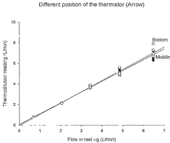
Figure 2.29a. Calibration lines showing different positions of the catheter tip within the lumen of the Arrow catheter. There is only a slight difference between the two lines. The slopes were 1.05 and 1.09. When  $X=5\text{L}/\text{min}$ ,  $Y$  ranges from 5.3 to 5.4L/min.
