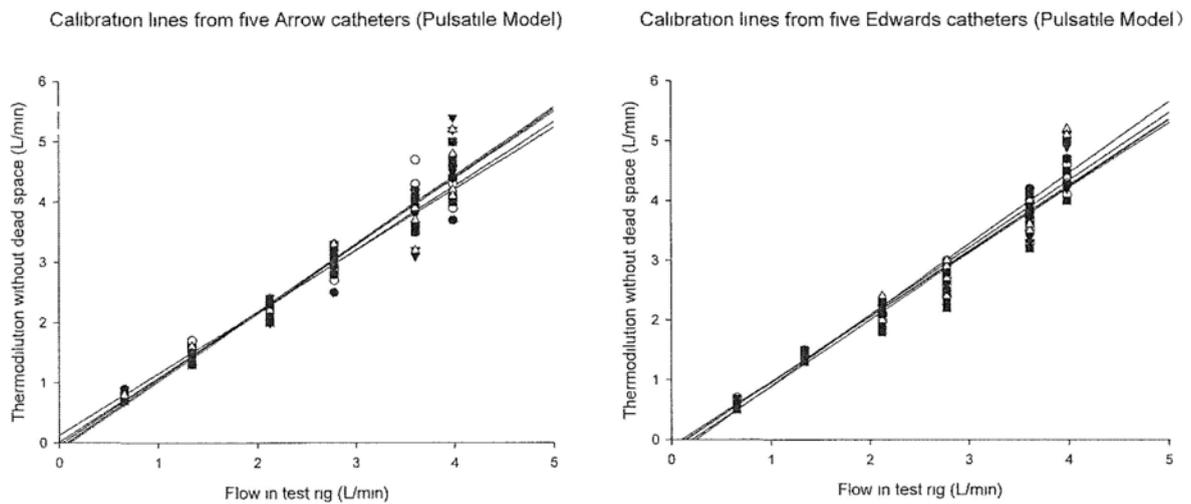
Figure 2.40. Plots comparing the calibration lines for 5 different Arrow catheters (left), and 5 different Edwards catheters (right) using pulsatile flow conditions. Lines constructed from sets of 5 readings taken at different flow rates between 0 and 5 L/min (corrected).
