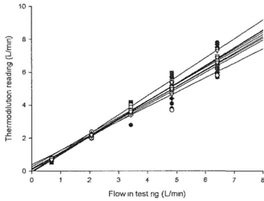
Figure 2.28a. Plot showing the influence of mixing distance when using an Arrow catheter. Slopes ranged from 0.880 to 1.151. When  $X=5\text{L/min}$ ,  $Y$  ranged from 4.8 to 5.7L/min.
