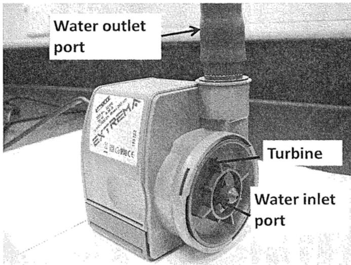
Figure 2.3. Heavy duty electrical water pump. The water in the reservoir is sucked into the inlet port and pumped out of the outlet port and circulated around the tubing system before being returned to the water tank.
