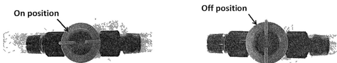
Figure 2.4a and 2.4b. Variable orifice flow regulator placed downstream to the pump. Flow rate was adjusted by turning the tap. The tap position was set against the reading from the flow meter.
