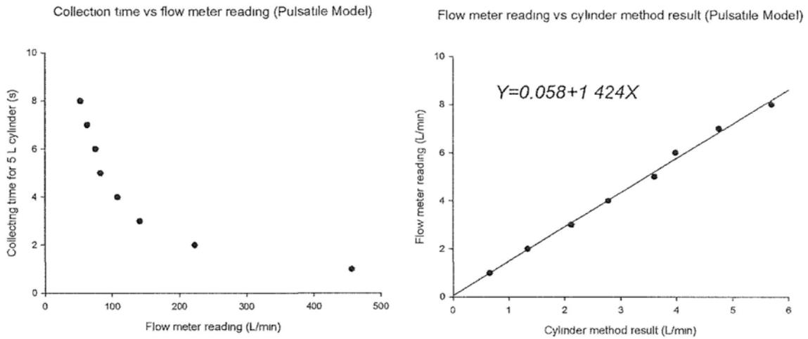
Figure 2.38. Regression plot showing the linear relation between the flow meter and cylinder methods with readings taken over the range of test rig flow rates under pulsatile flow conditions.
