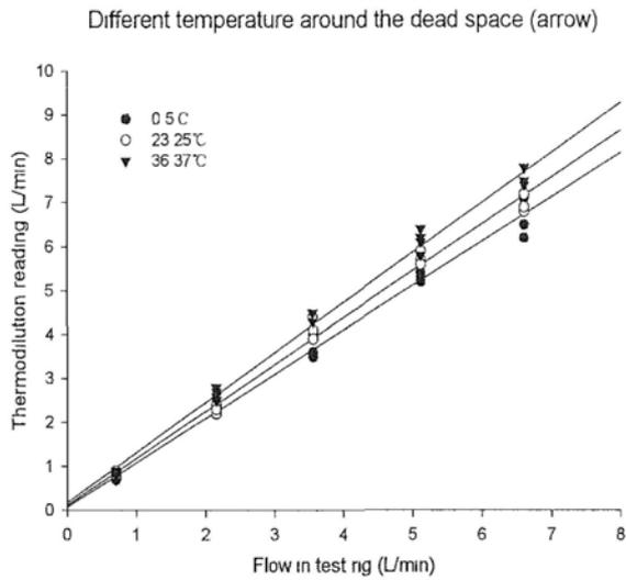
Figure 2.30a. Calibration plot showing the effect of 3 different ambient temperatures applied to the dead space of the Arrow catheter. The slopes ranged from 1.01 to 1.14. When  $X=5L/min$ ,  $Y$  was 5.1, 5.4 and 5.9 L/min for 0-5, 23-25, 36-37°C respectively.
