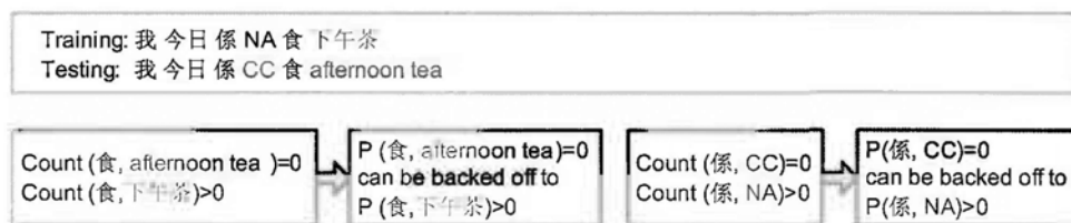
Figure 5.5: An example of a reasonable estimation of code-mixing unseen n-grams with seen n-grams
