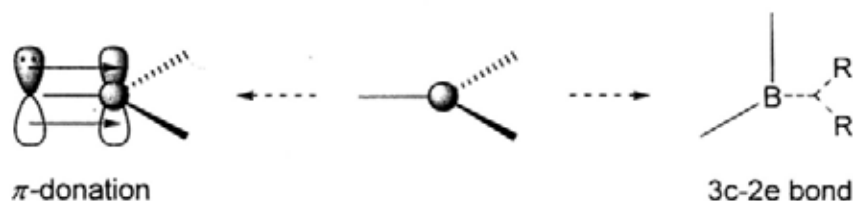
Figure 4.21. Compensation of electron-deficiency in classic boranes.
