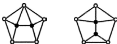
Figure 1.4. Trapezoidal open faces in the CAD 13-vertex carboranes.
