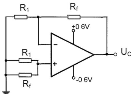
Fig. 65 schematic of testing circuit for  $V_{off}$
