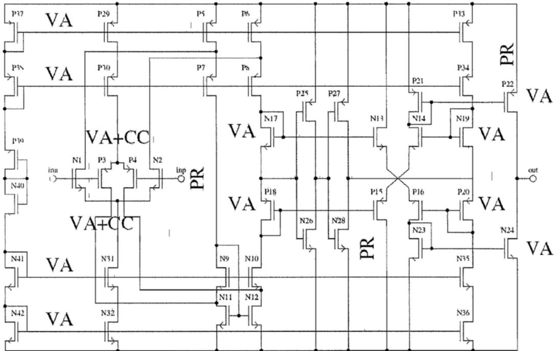
Fig. 31 Schematic of a buffer amplifier
