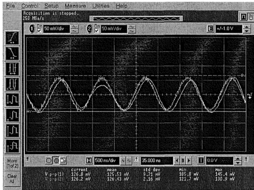
Fig. 68 waveforms for UGF measurement
