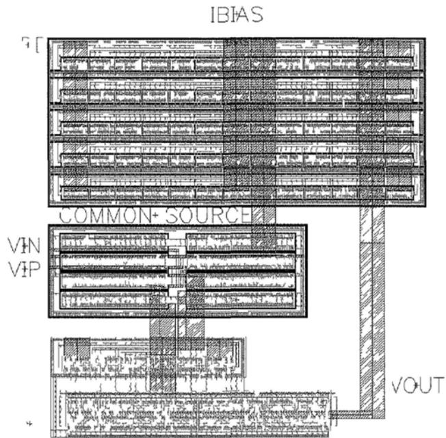
Fig 57 Layout for 2-stage op amp except Miller Capacitor
