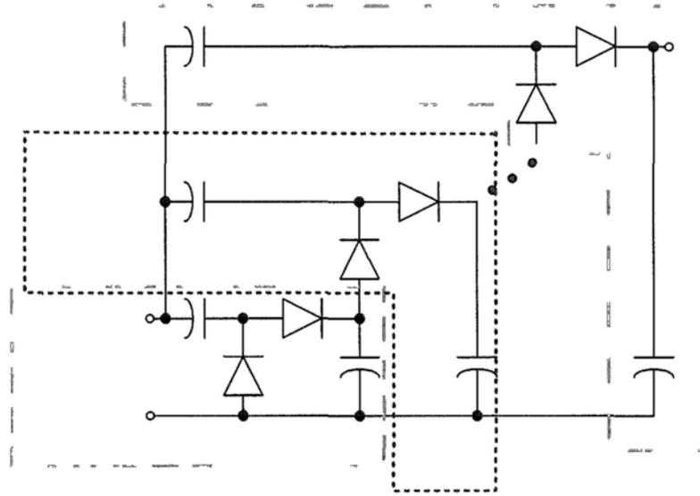
Fig. 6 Circuit structure of a VM
