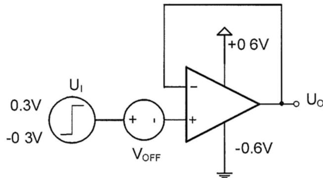
Fig. 72 schematic for SR test
