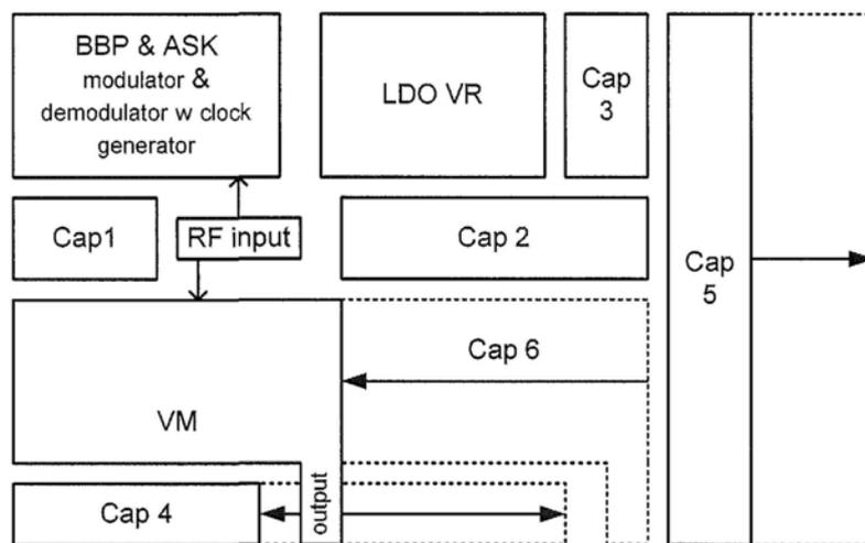
Fig. 8 Template floorplan with critical routings for reconfigurable RFID tag
