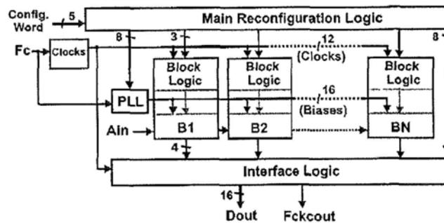
Fig. 2 A reconfigurable ADC structure
