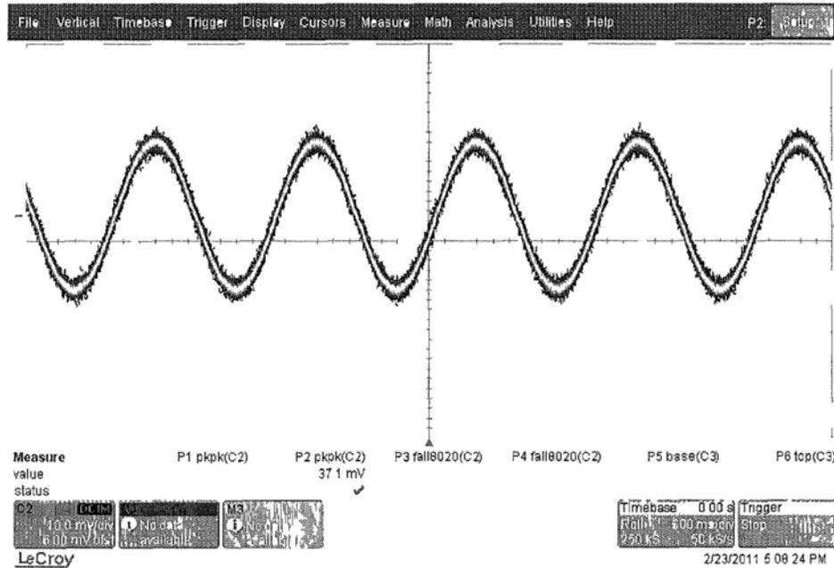
Fig. 73 Common mode gain test waveform
