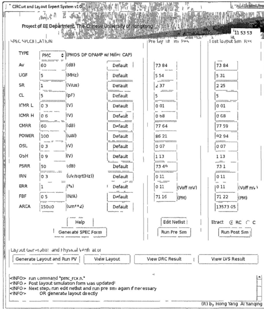
Fig. 64 Comparison of results after Post-layout Simulation
