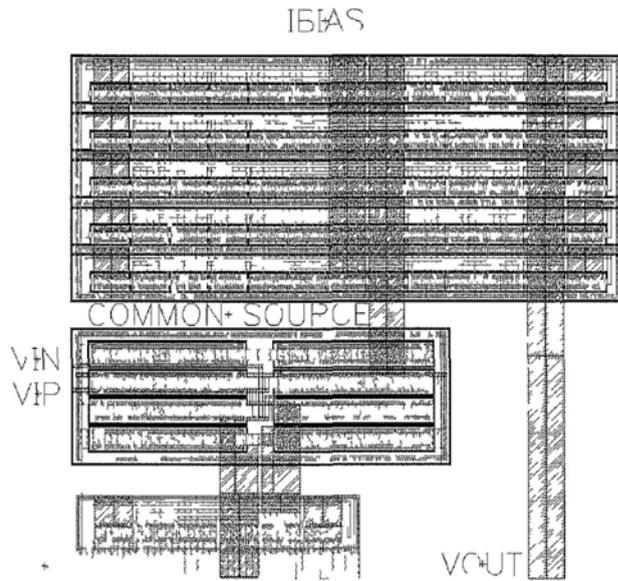
Fig 56 CA layout for 2-stage op amp with routings
