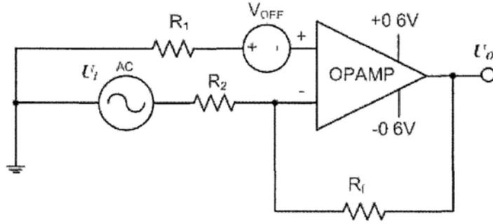
Fig. 66 testing schematic for open loop gain  $A_V$
