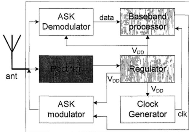
Fig. 4 diagram of a passive UHF RFID tag
