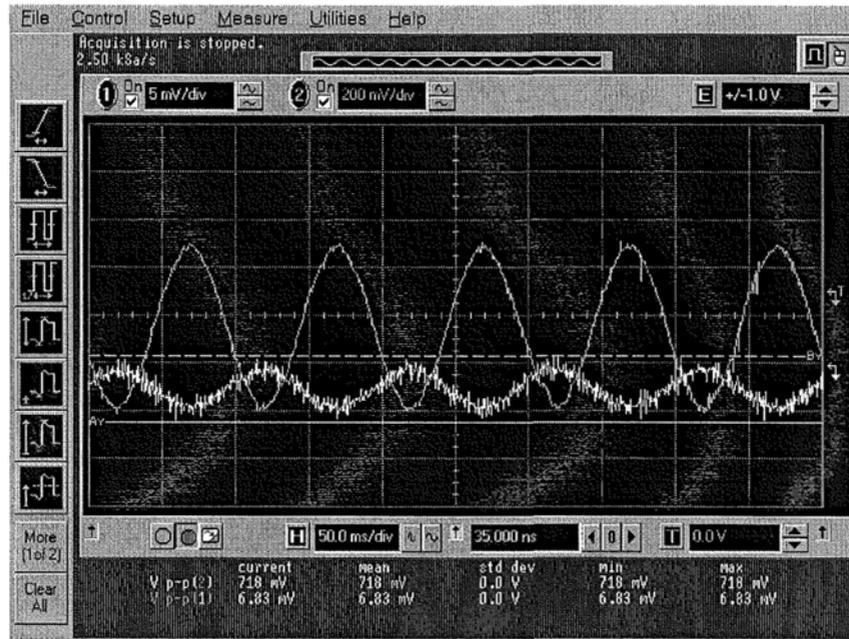
Fig. 67 waveforms of input & output ac signals for  $A_V$  measurement
