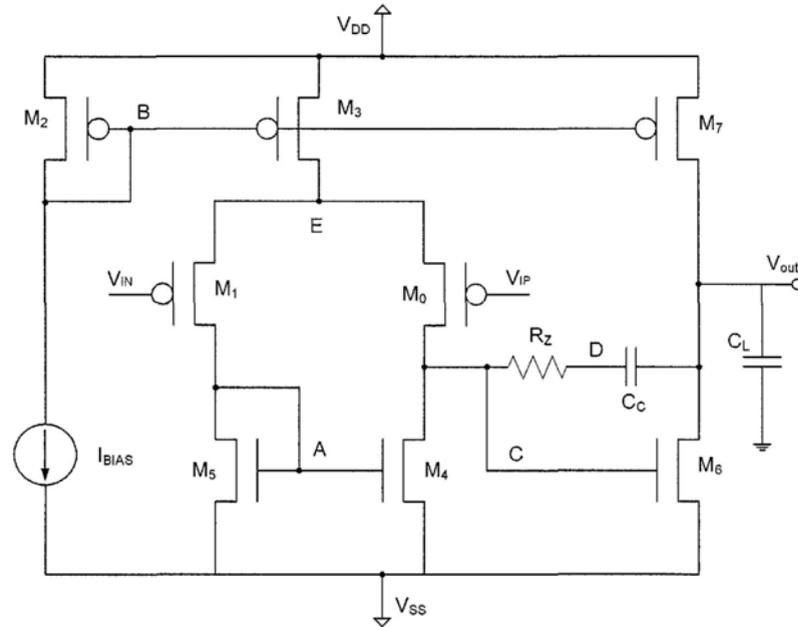
Fig. 38 Schematic of 2-stage op amp with Miller cap and PMOS input
