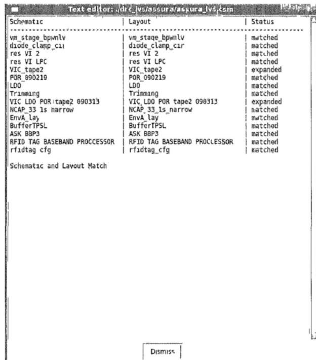
Fig.16 LVS results for generated RFID tag layout
