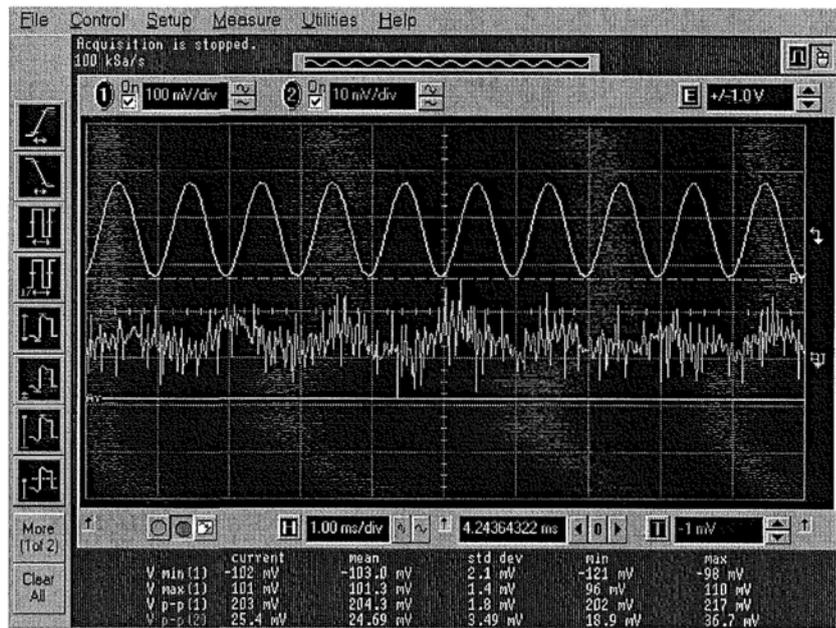
Fig. 75 waveforms for PSRR- @ 1KHz
