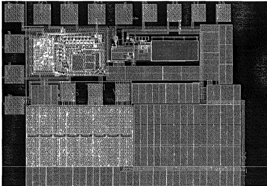
Fig. 12 Layout of RFID tag with 8 stages of VM
