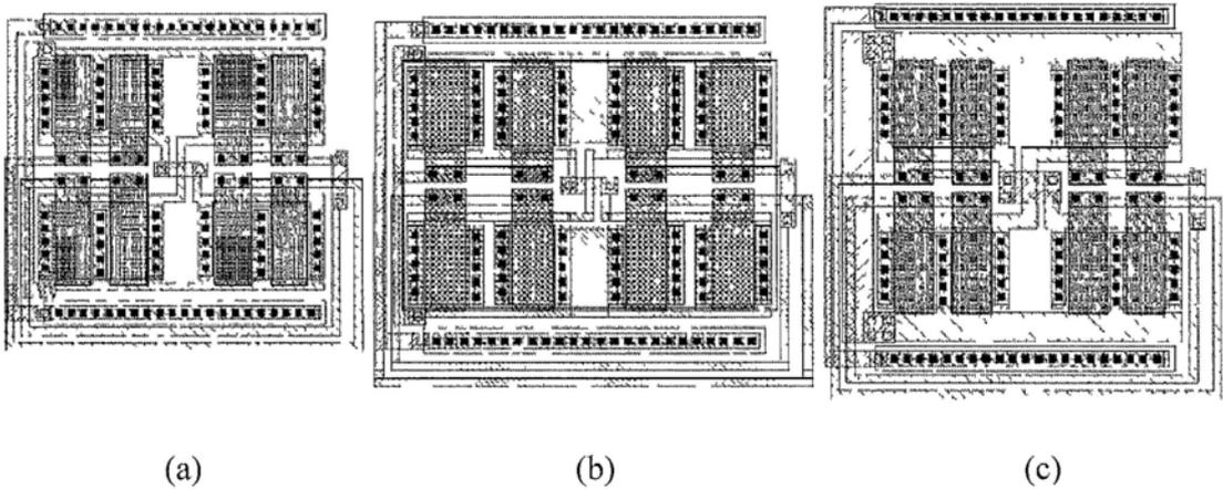
Fig. 29 Different layout implementation of a differential pair
