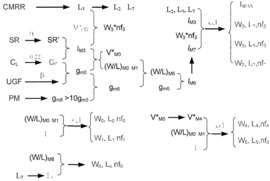
Fig. 39 Deduction flow for initialization of parameters (2-stage case)
