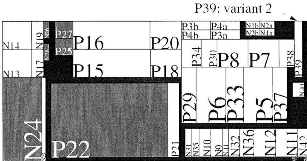
Fig. 32 one placement of an aspect ratio for the circuit of Fig.28
