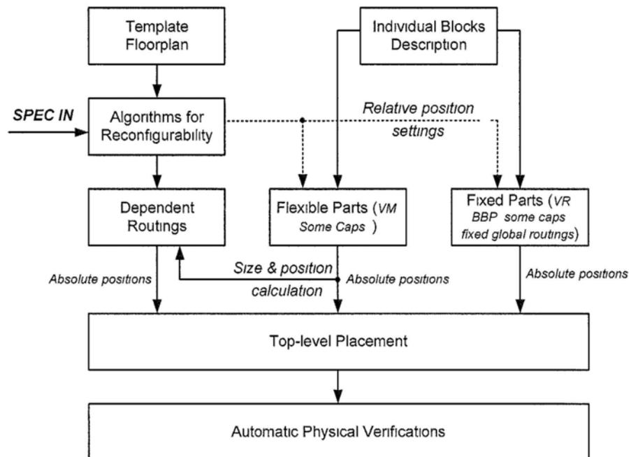
Fig. 9 Design Flow for the proposed reconfigurable RFID design
