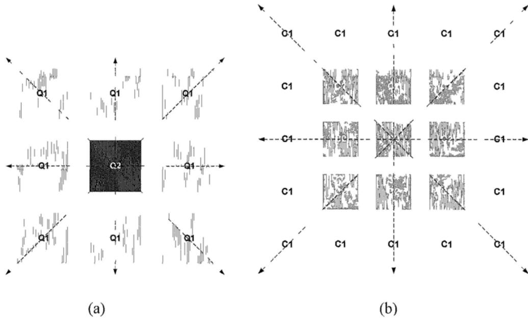
Fig. 27 (a) Common-centroid layout (bipolar) (b) Common-centroid layout (capacitor)
