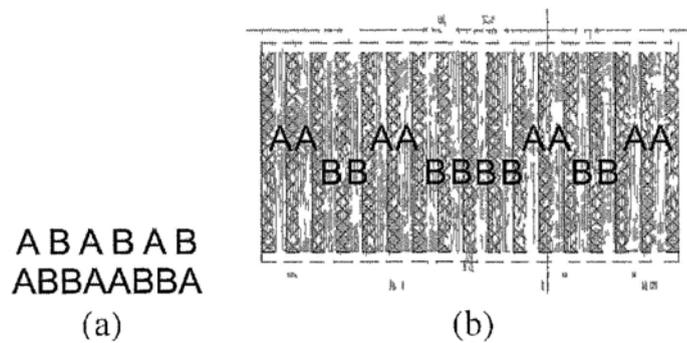
Fig. 26 Interdigitized transistor layout
