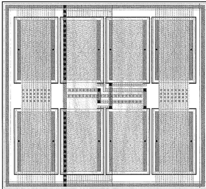
(b) Layout of the PMOS differential pair with S/B connected
