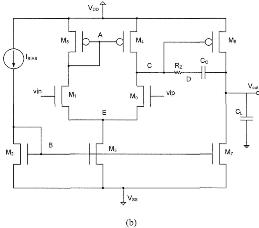
Fig. 59 (a) total layout of 2-stage op amp with Miller Compensation (NMOS-input) (b) the corresponding schematic
