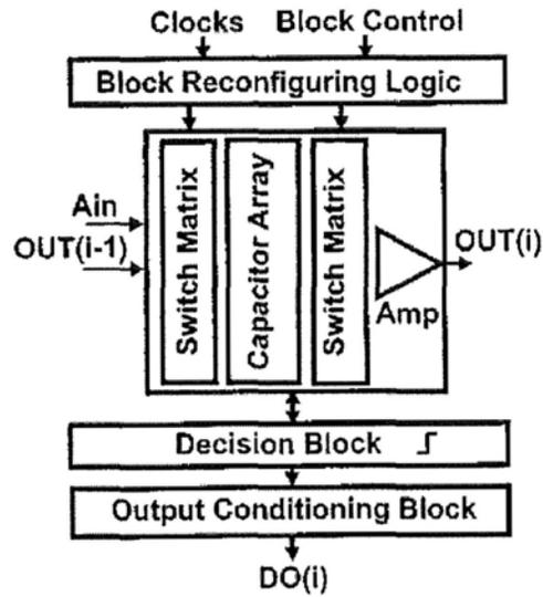
Fig. 3 Structure of a basic building block
