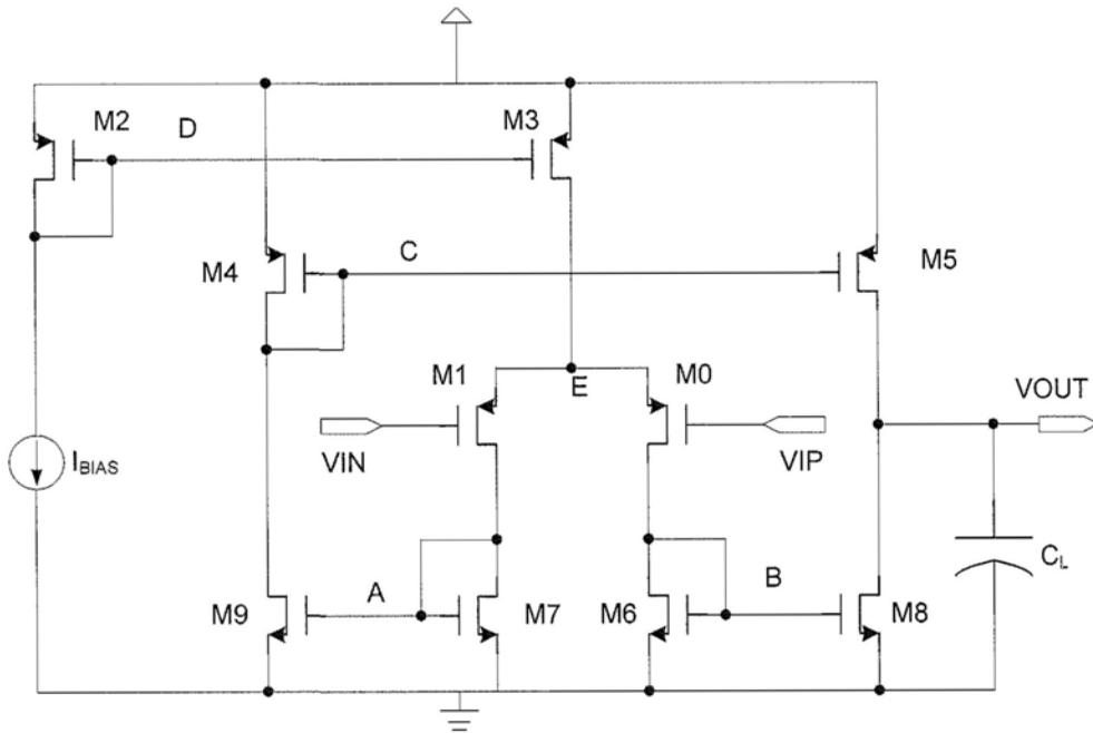
Fig. 40 Schematic of single-stage current mirror op amp
