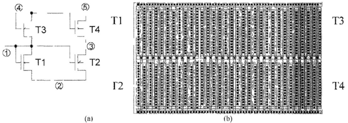
Fig. 28 (a) Schematic (b) the corresponding module layout of a cascode current mirror
