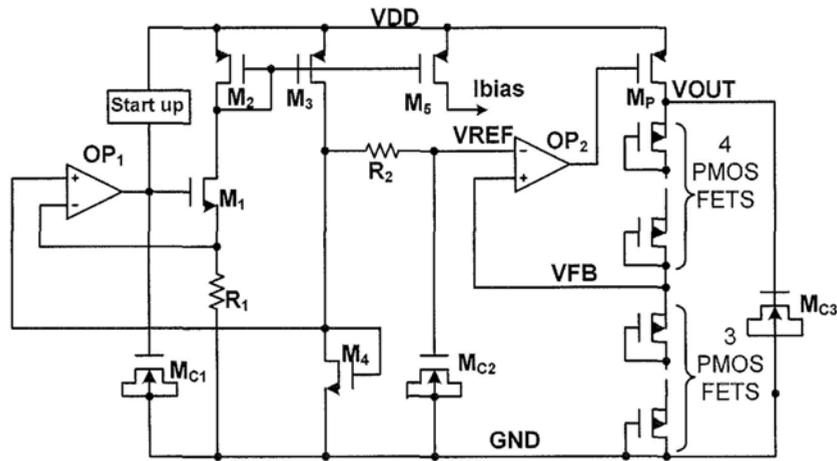
Fig. 10 Proposed LDO voltage regulator
