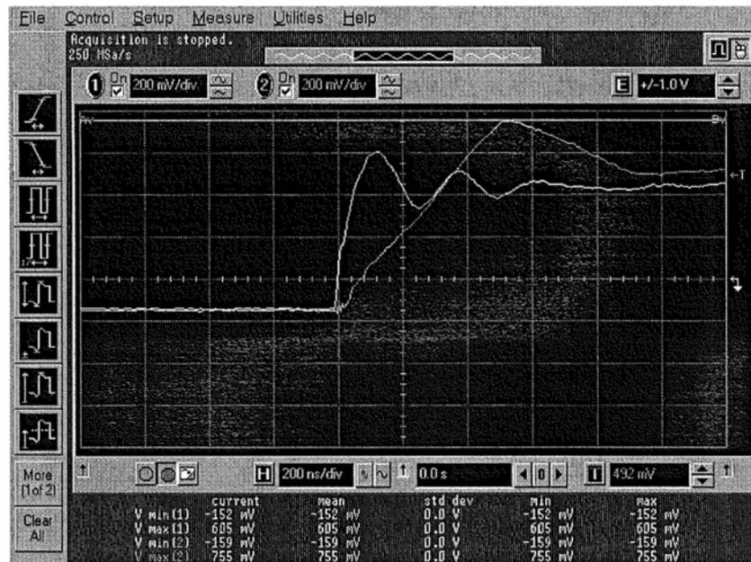
Fig. 70 Rising edge SR test waveform
