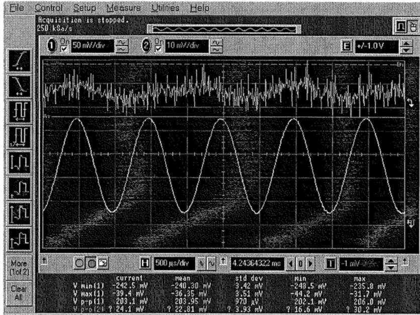
Fig. 74 waveforms for PSRR+ @ 1KHz
