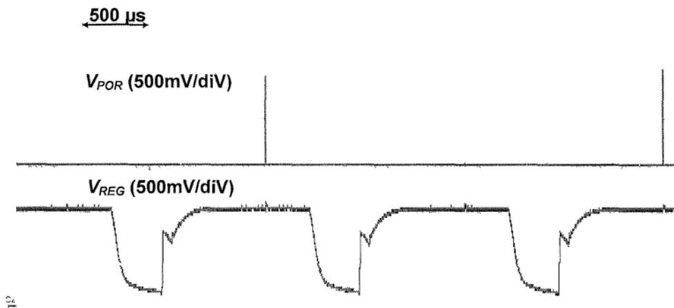
Fig. 2.21 Measured power-on and power-off responses of the POR circuit with the proposed power-off auto-discharging path
