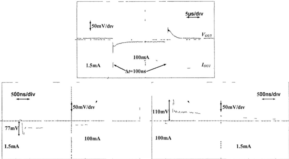
Fig. 3.15 Measured load transient response when  $V_{IN} = 0.75$  V,  $V_{OUT} = 0.5$  V,  $C_{OUT} = 50$  pF and 100-ns edge time
