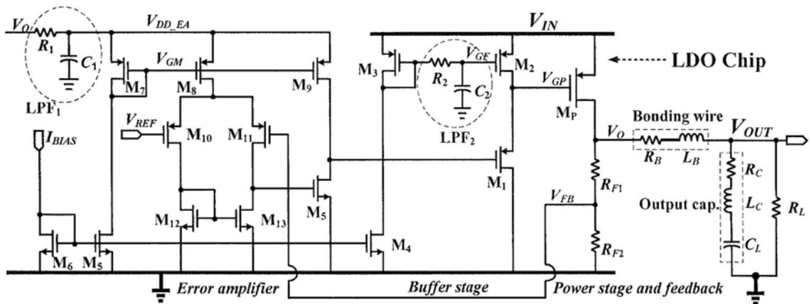
Fig. 4.13 Schematic of proposed EFPF-LDO
