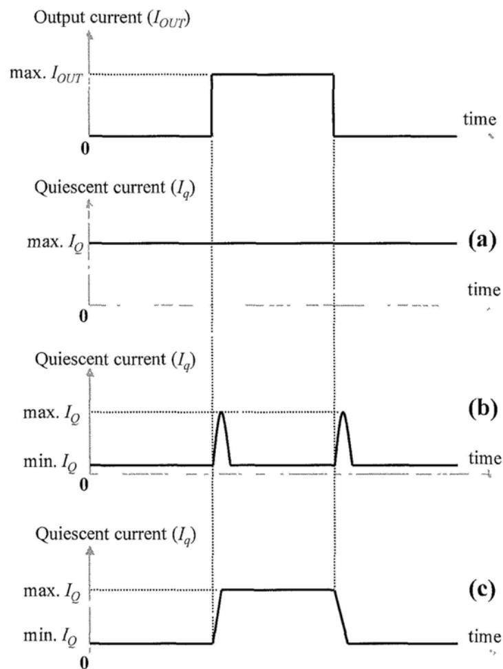
Fig. 3.2 Different methods to improve load transient response
