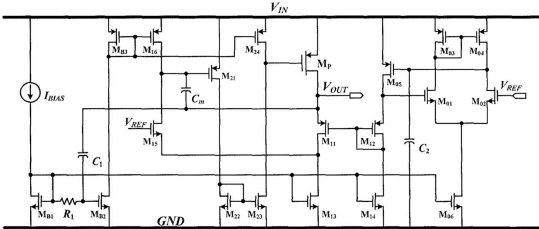
Fig. 3.8 Full schematic of the proposed LDO (with slew-rate enhancement)
