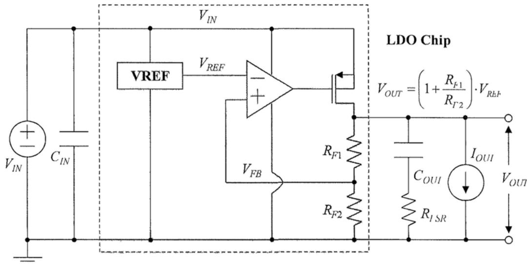
Fig. 1.3 Typical LDO topology with PMOS as pass element
