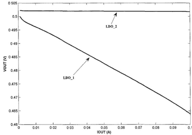
Fig. 3.5 Simulated load regulations of the LDOs shown in Fig. 3.3 (LDO\_1) and Fig. 3.4 (LDO\_2)
