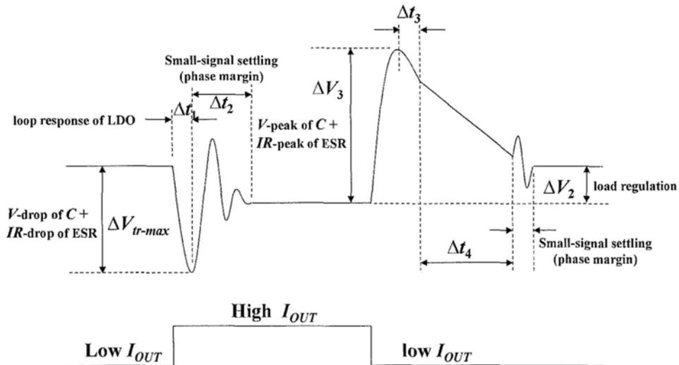
Fig. 3.1 Typical load transient response of LDO
