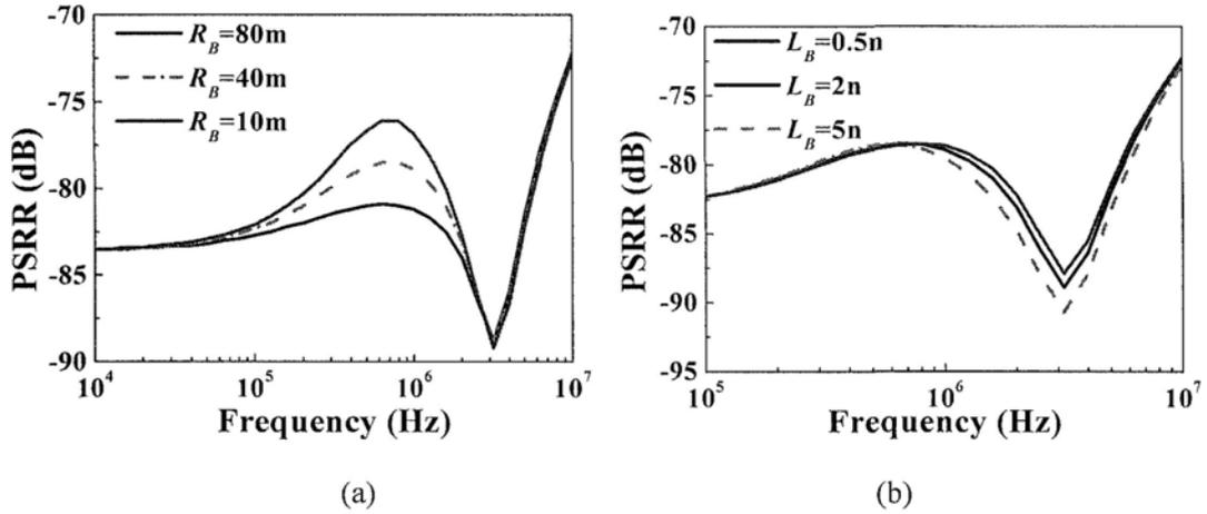
Fig. 4.17 PSRR simulation results with different bonding wire (a) resistance and (b) inductance
