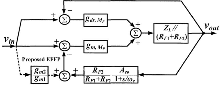
Fig. 4.11 Signal flow chain of proposed EFPF-LDO
