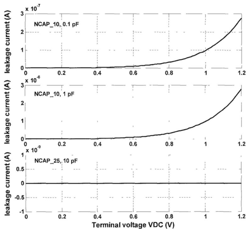
Fig. 2.18 Simulation results of gate leakage current
