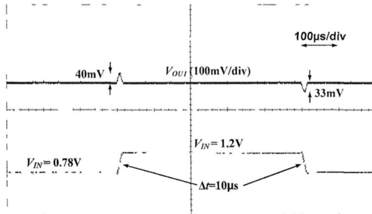
Fig. 3.16 Measured line transient waveform when  $V_{OUT} = 0.5$  V,  $I_{OUT} = 1$  mA and  $C_{OUT} = 10$  pF
