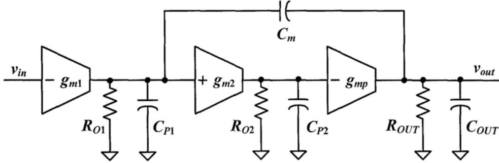
Fig. 3.6 Small-signal modelling of the proposed LDO
