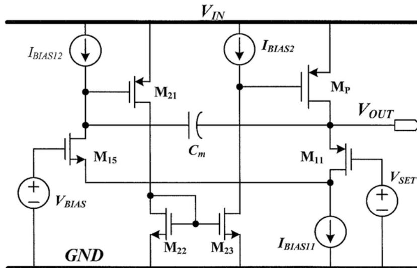
Fig. 3.4 Proposed OCL-LDO structure (core part, without slew-rate enhancement)
