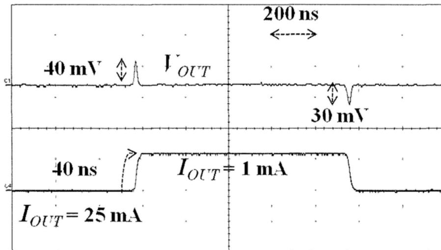
Fig. 4.22 Measured load transient response
