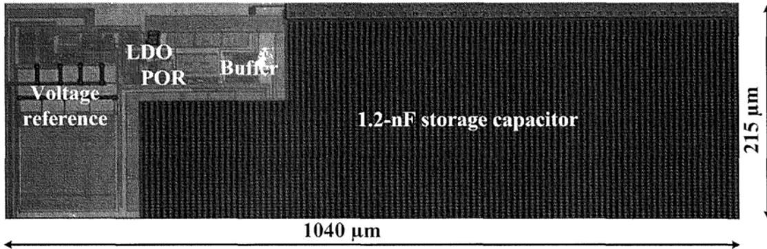
Fig. 2.9 Chip micrograph
