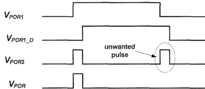
Fig. 2.8 Ideal time sequence of POR circuit
