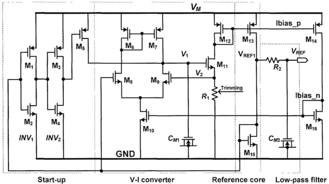
Fig. 2.3 Schematic of the voltage reference
