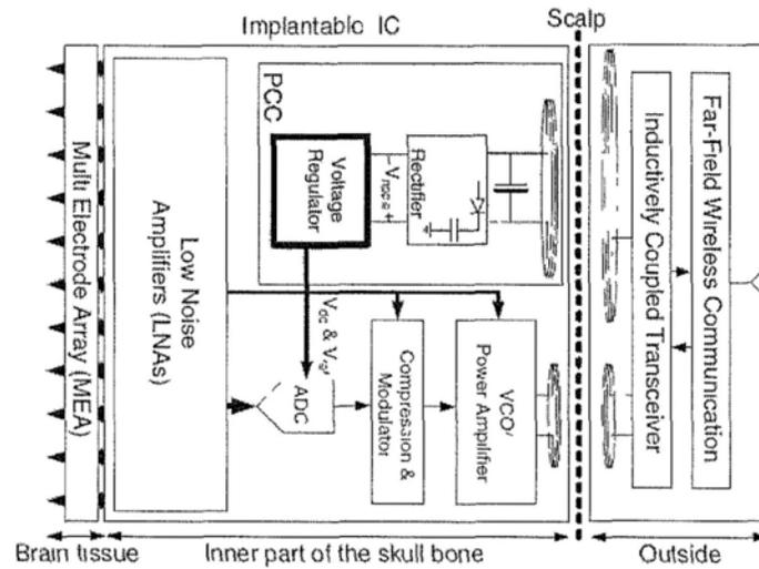
Fig. 1.1 A wireless-powered energy-autonomous system for brain implant application [13]
