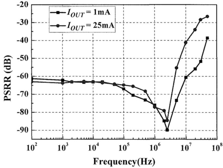
Fig. 4.21 Measured PSRR performance under different load conditions
