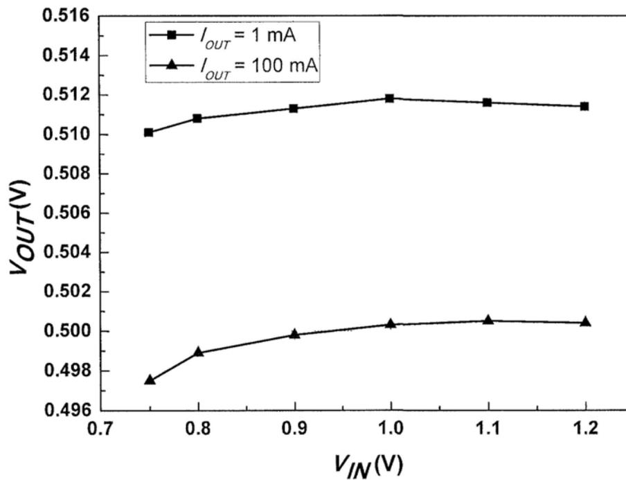
Fig. 3.17 Measured line regulation for  $I_{OUT} = 1$  mA and  $I_{OUT} = 100$  mA when  $V_{REF} = 0.5$  V (no external  $C_{OUT}$  is added)
