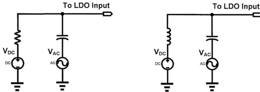
Fig. 4.2 AC signal injection through capacitor coupling
