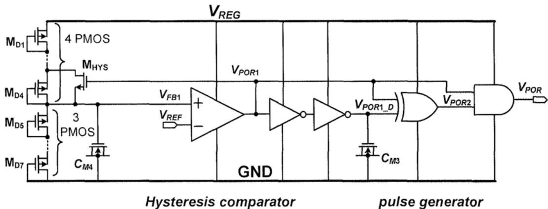
Fig. 2.7 Schematic of the proposed POR circuit
