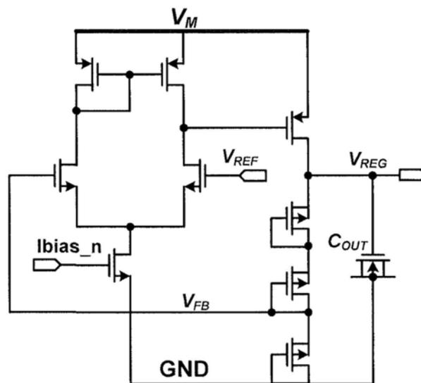
Fig. 2.5 Schematic of the low-dropout voltage regulation circuit
