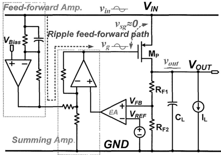
Fig. 4.9 A high-PSRR LDO with ripple cancellation by feed-forward and summing amplification
