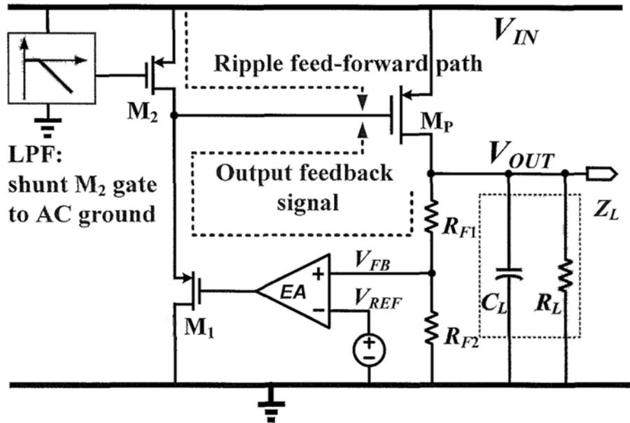
Fig. 4.10 Block diagram of proposed LDO
