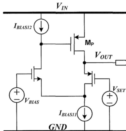
Fig. 3.3 Prior work: LDO structure based on FVF
