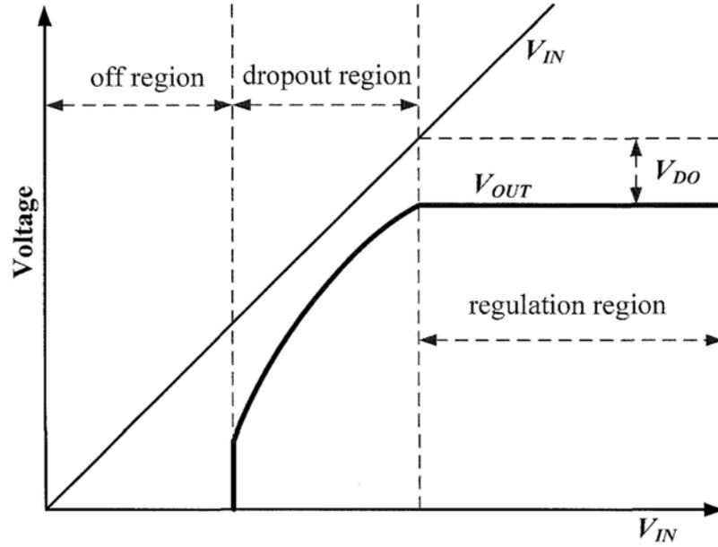
Fig. 1.4 Typical input/output voltage characteristics of a LDO
