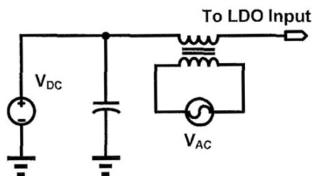
Fig. 4.4 AC signal injection through a transformer
