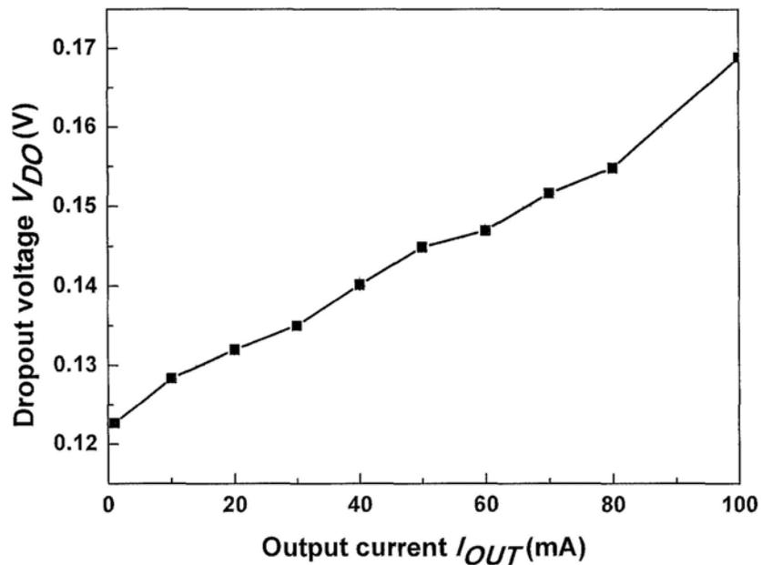
Fig. 3.19 Measured dropout voltage vs.  $I_{OUT}$  when  $V_{REF} = 1$  V (no external  $C_{OUT}$  is added)
