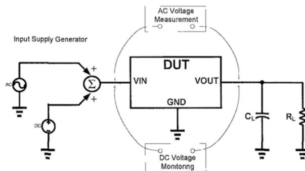
Fig. 4.1 LDO PSRR measurement setup
