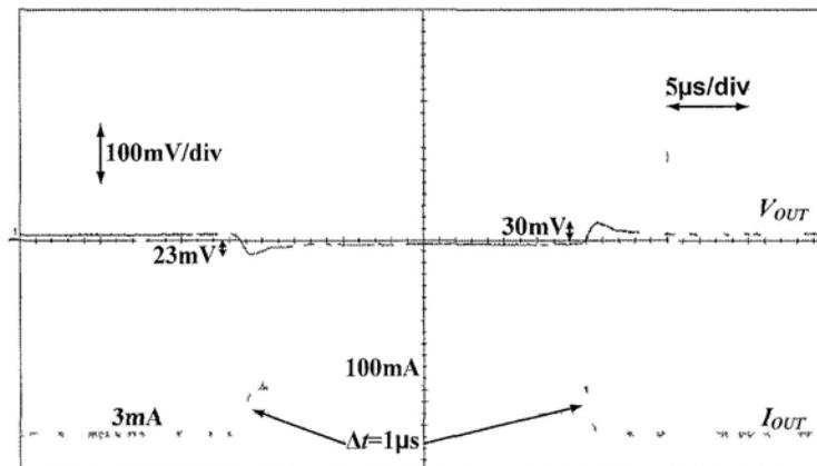
Fig. 3.13 Measured load transient response at  $V_{IN} = 1.2\text{ V}$ ,  $V_{OUT} = 0.5\text{ V}$ ,  $C_{OUT} = 50\text{ pF}$  and 1- $\mu\text{s}$  edge
