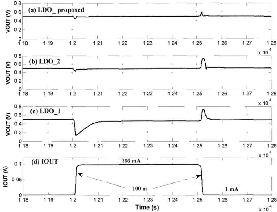
Fig. 3.9 Simulated load transient responses of different LDO topologies
