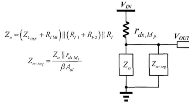
Fig. 4.7 A simple modeling to investigate the PSRR of LDO
