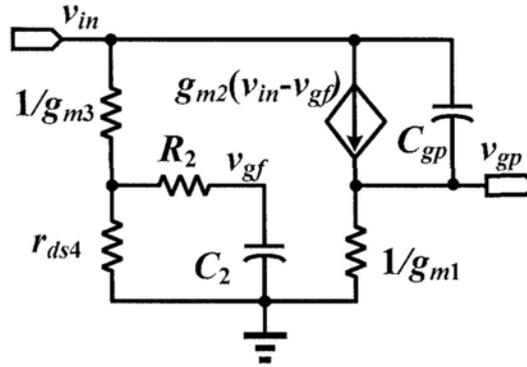
Fig. 4.15 Small signal modeling of embedded feed-forward amplifier
