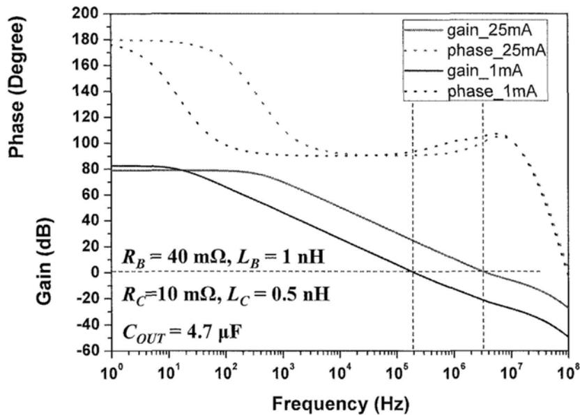
Fig. 4.16 AC simulation results of loop gain under different load conditions
