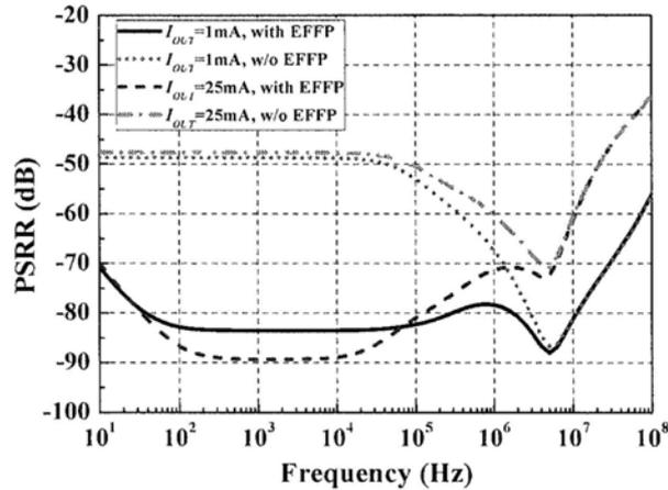
Fig. 4.12 PSRR simulation results with and without EFPF
