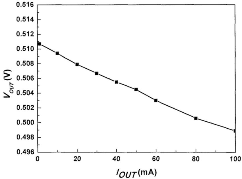
Fig. 3.18 Measured load regulation when  $V_{IN} = 0.8$  V,  $V_{REF} = 0.5$  V (no external  $C_{OUT}$  is added)
