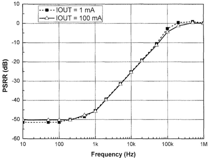
Fig. 3.21 Measured PSRR vs. frequency for  $I_{OUT} = 1$  mA and  $I_{OUT} = 100$  mA when  $V_{OUT} = V_{REF} =$
