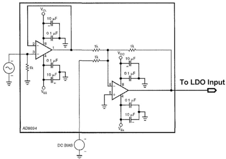
Fig. 4.5 A input supply solution for signal generator without DC bias ability by using AD8034 [12]
