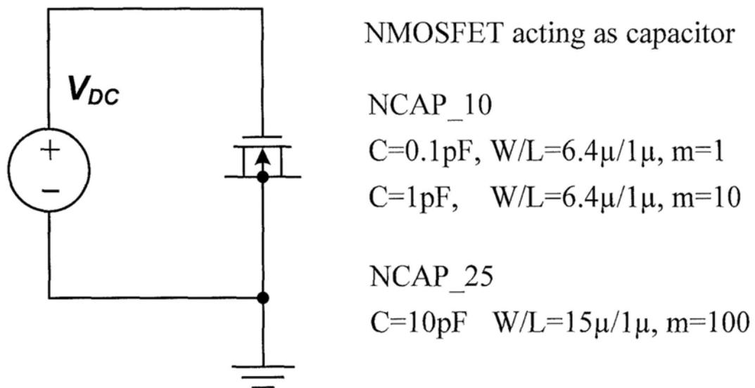
Fig. 2.17 Test setup for the gate leakage simulation
