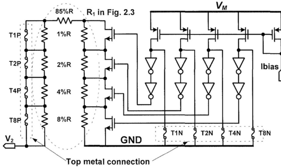
Fig. 2.4 Schematic of the trimming circuit
