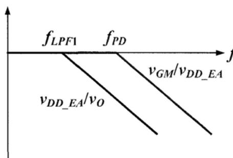
Fig. 4.14 Frequency response of  $LPF_2$  and voltage divider.
