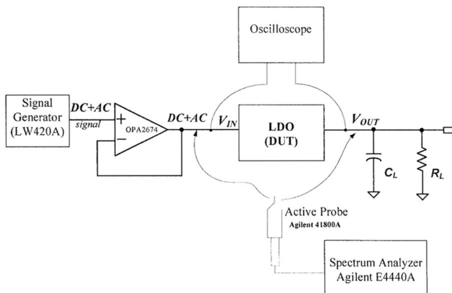
Fig. 4.20 PSRR measurement setup
