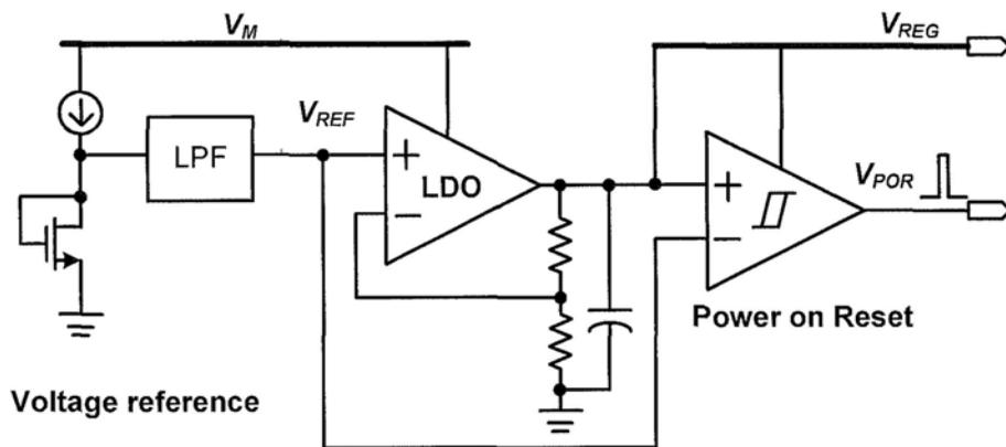
Fig 2 2 Structure of the proposed voltage regulator
