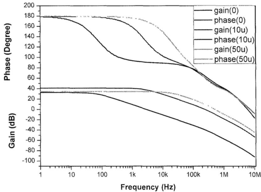
Fig. 2.6 Bode plots of LDO circuit under 0-, 10- and 50- $\mu$ A load current
