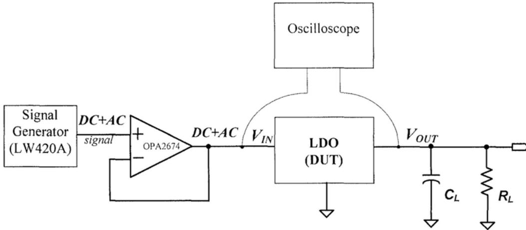
Fig. 3.20 PSRR setup through voltage buffer and oscilloscope
