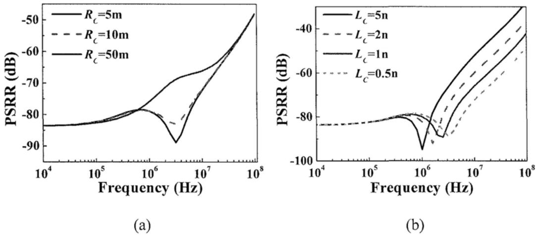
Fig. 4.18 PSRR simulation results with different (a) ESR and (b) ESL of  $C_L$
