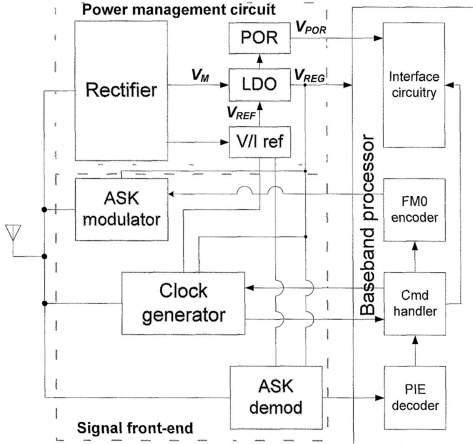
Fig. 2.1 Diagram of a typical passive RFID tag
