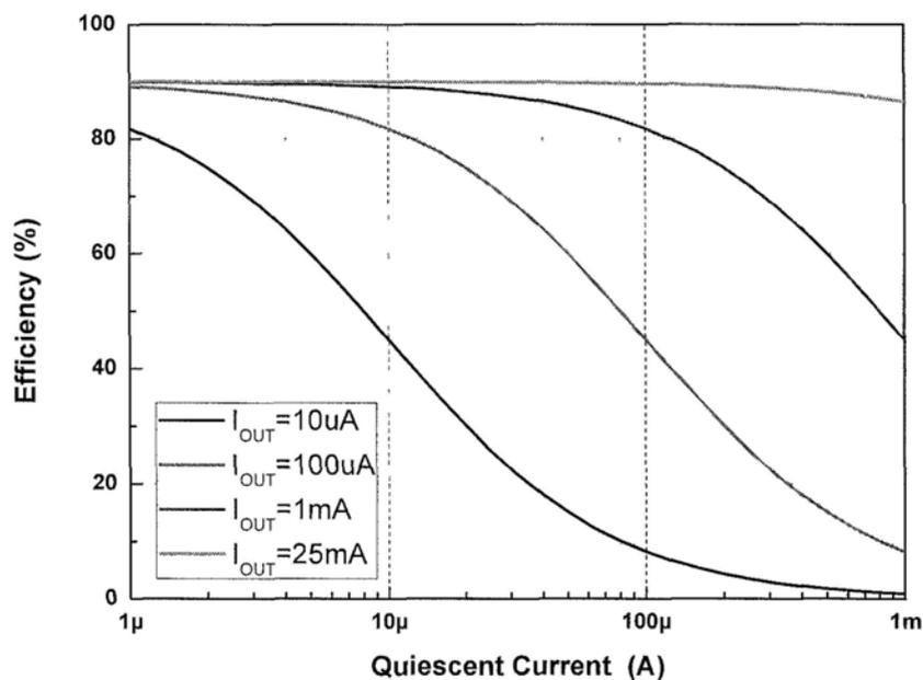
Fig. 1.5 LDO power efficiency changing with  $I_q$  in different load conditions
