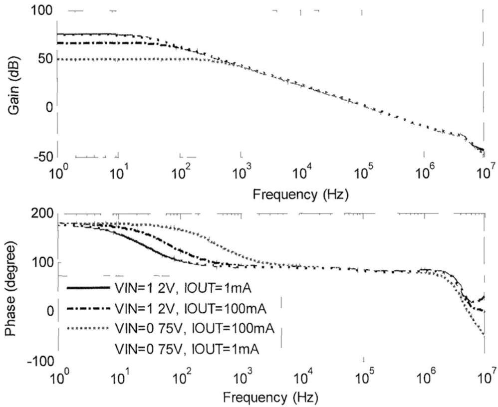
Fig. 3.7 Simulated bode plots of proposed LDO with different  $V_{IN}$  and  $V_{OUI}$  ( $C_{OUT} = 10$  pF).
