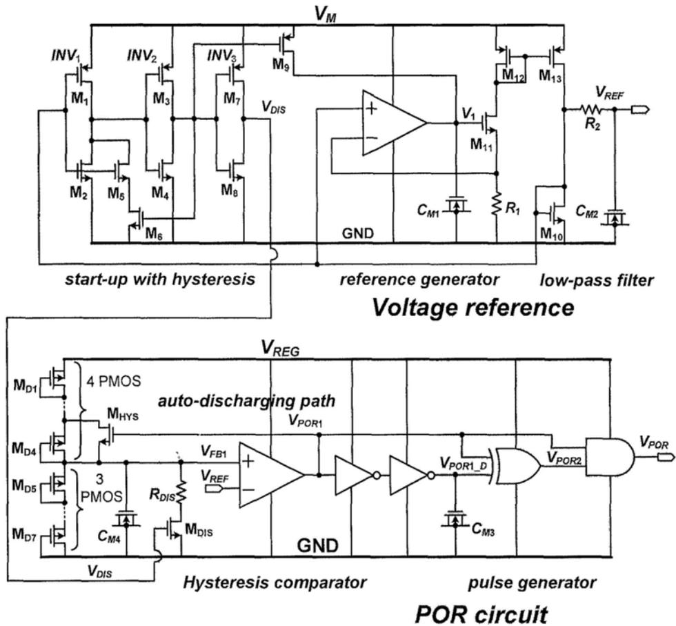
Fig. 2.15 Proposed voltage reference and POR circuit in 90-nm CMOS technology
