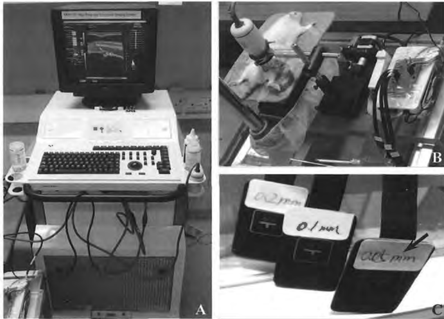
Figure 2.6-1 The procedure of 3D-HF-PDU scanning. A: Vevo-770 high frequency In-Vivo Micro-Imaging System. B: The rat was prone positioned on a flat with the extremities secured. Coupling gel was loaded to cover the exposed callus region for linear scanning. C: The step size of scanning was set at 0.05 mm (black arrow).
