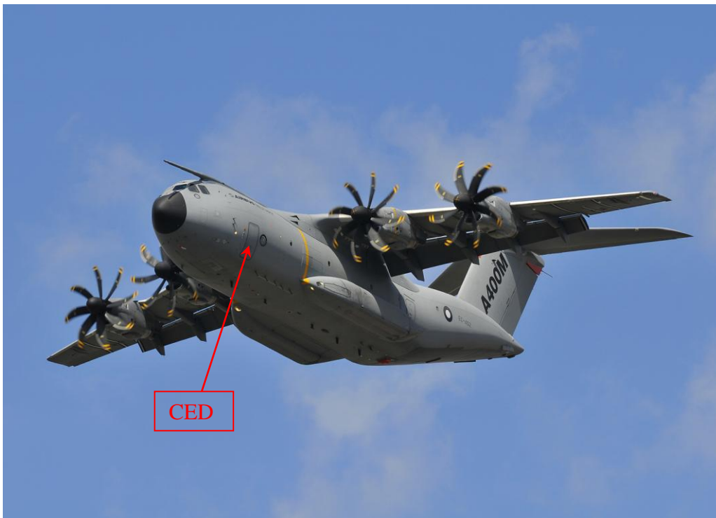
Figure 1. Airbus A400M with the Crew Entrance Door pointed out. Picture copied from Airbus Military [1]
