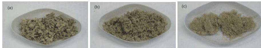
Fig. 24. Wheat straw pulp fractions: (a) > 16 mesh, (b) 16–32 mesh, (c) < 35 mesh.
