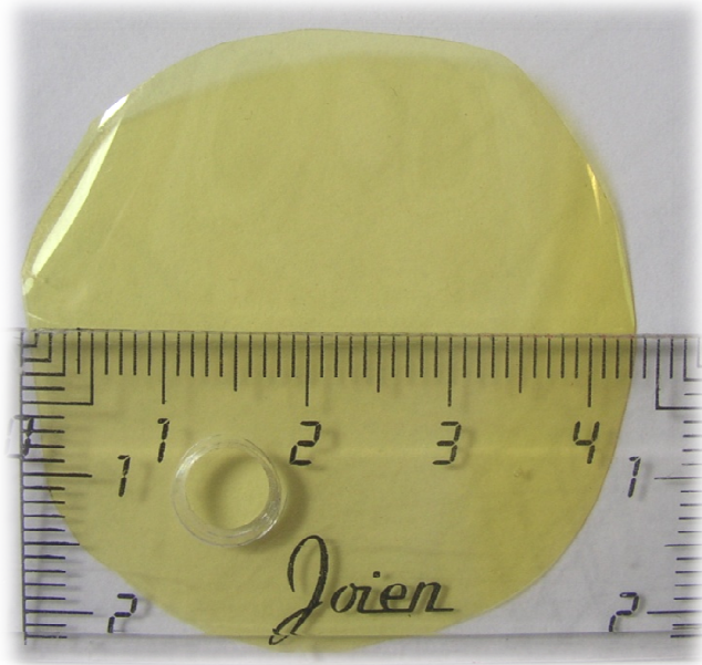
Figure II – 2. Image of a typical Matrimid dense film prepared in this work
