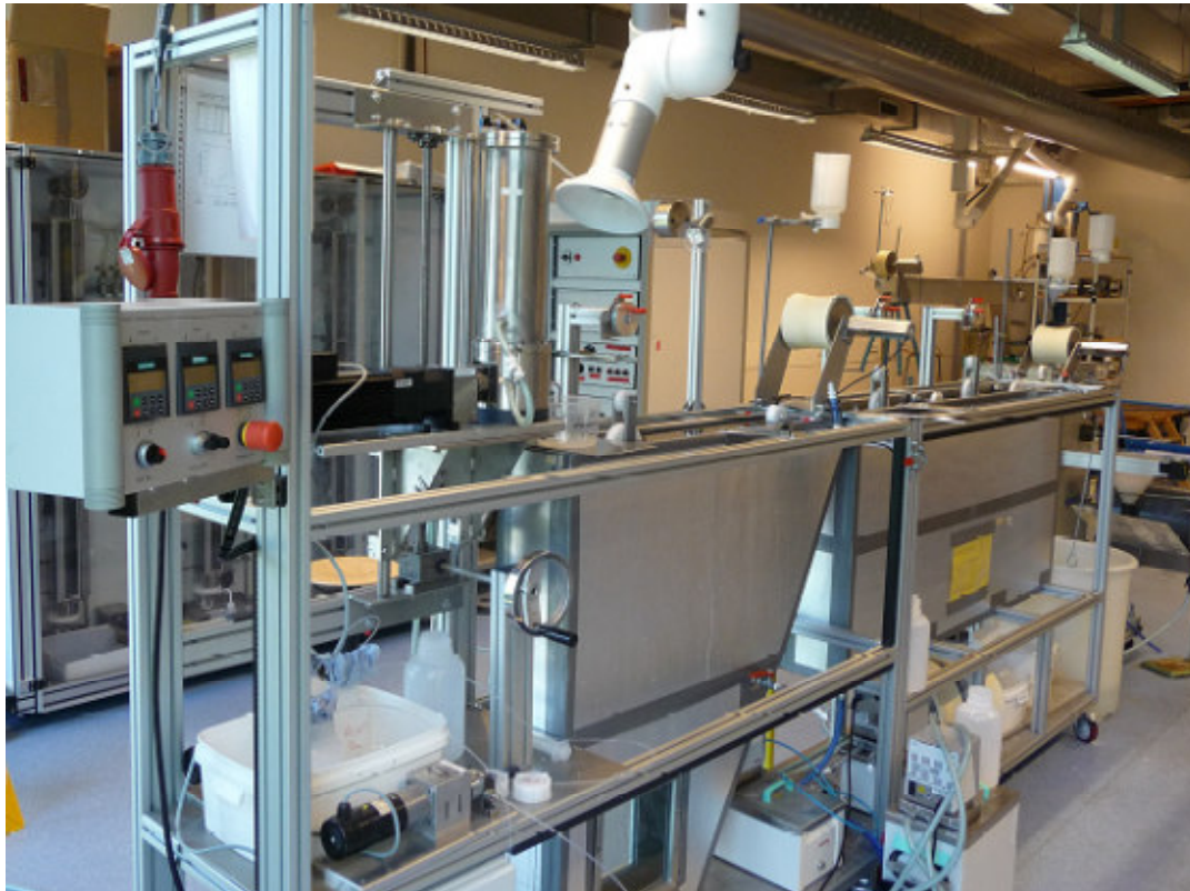
Figure III - 7. Image of the spinning line used for the fabrication of the asymmetric hollow fiber membranes (University of Twente).
