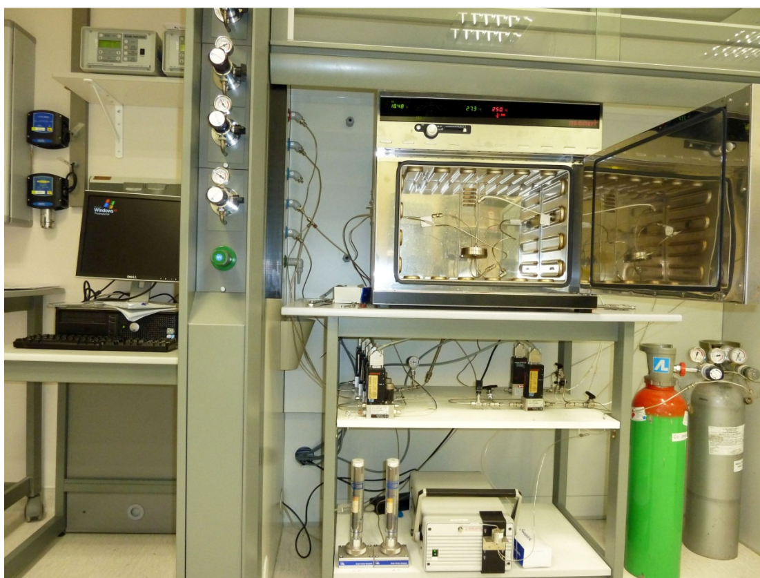
Figure II – 8. The photographic image of the experimental permeation set – up with the heating oven open for a better viewing of the testing cell.
