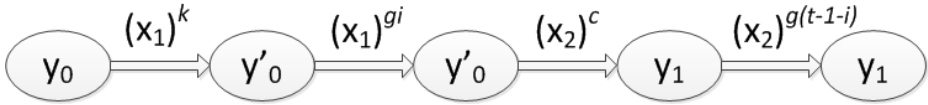
Fig 2. Our multicollision method with computational complexity in O(2^{\frac{n}{2}}) and message length in O(2^n) .
