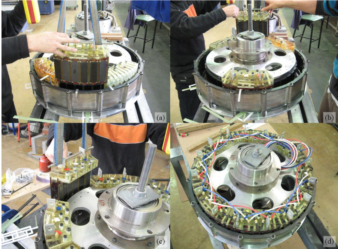
Figure 52: Inserting stator segments into the double-sided rotor PMSG.
