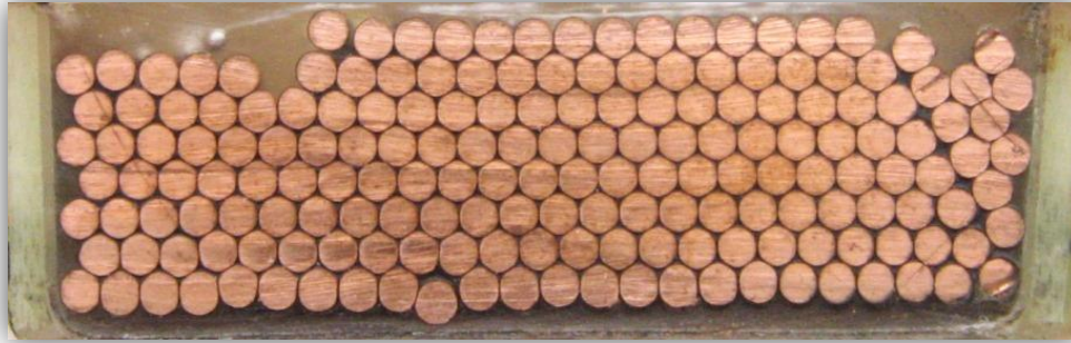
Figure 28: Cross sectional view of copper conductors in stator slot
