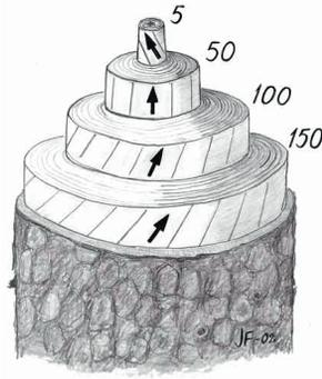
**Figure 3.1:** Spiral grain orientation in a log at different annual rings (5, 50, 100, 150) in an old spruce tree. The grain angle is the angle between the direction of growth and the wood fibres. (Illustration from Harald Säll, Forestry and Wood Technology, Linnaeus University, Växjö.)
