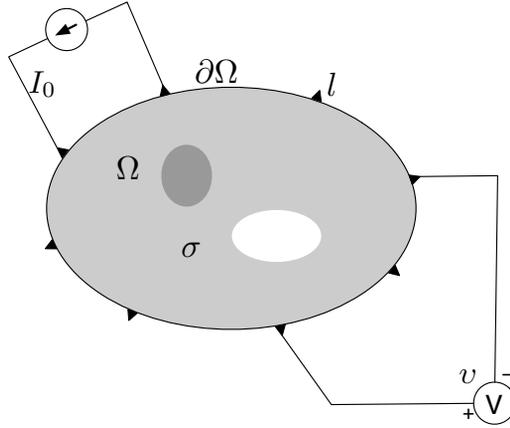
**Figure 5.1:** EIT measurement set-up. The domain is  $\Omega$ ,  $\partial\Omega$  the boundary,  $l$  sensor label,  $I_0$  the exciting current and  $v$  measured potential differences. Varying conductivity  $\sigma$  is indicated with colour changes.
