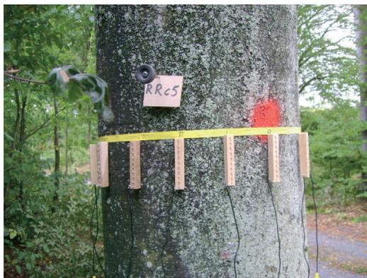
**Figure 3.3:** Measurement of the interior of a beech tree, searching for red coloured heartwood with EIT. (Photo and experimental measurement equipment, Bengt Bengtsson, Romele Elektronik AB.)
