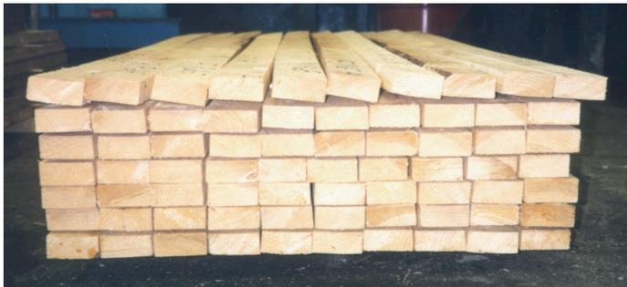
**Figure 3.2:** Picture of sawn boards from four trees with normal grain angle (six bottom layers) and a tree with large grain angle (top row). (Photo, Harald Säll, Forestry and Wood Technology, Linnaeus University, Växjö.)
