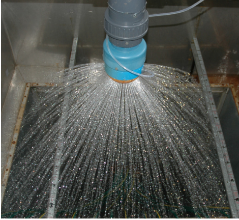
Figure 5.18: Sphere spray nozzle in operation
