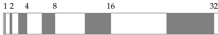
Figure 1.1: The range table for six LOD ranges with relative sizes at the top. The morph area of each range is shown in gray.
