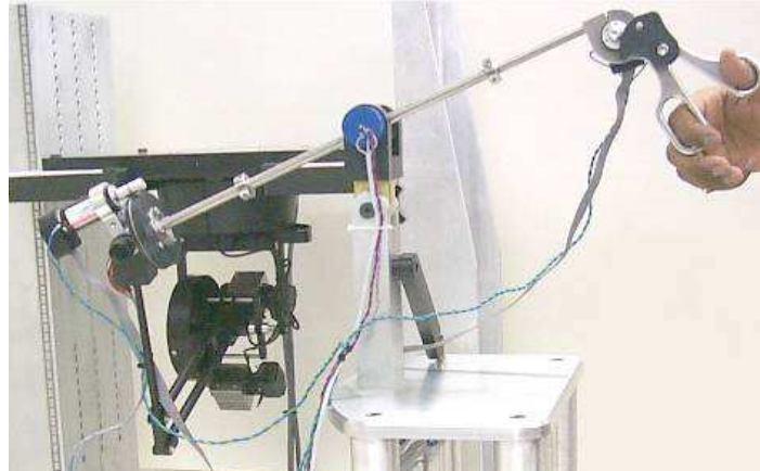
Figure 4: The force reflective master-slave system of Tavakoli et al. (2003)
