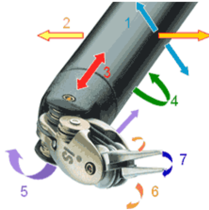
Figure 2: The EndoWrist design with its 7 DOF indicated ( EndoWrist design , [S.a.])
