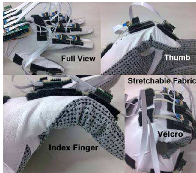
Figure 12: The finger motion capturing device of Li et al. (2011)
