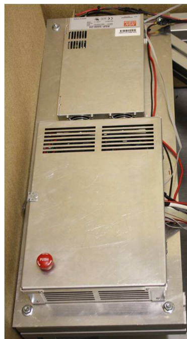
Figure 25: The SSM electronics box and power supply assembly
