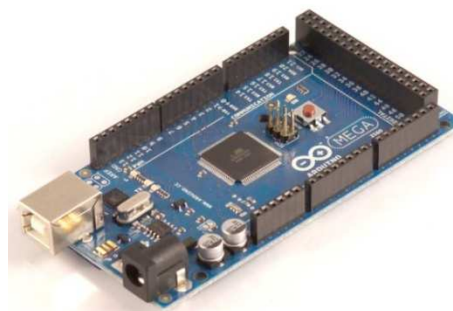
Figure 20: The Arduino Mega 2560 ( Arduino Mega 2560 , [S.a.]
