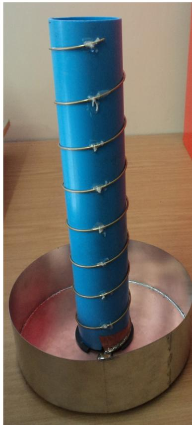
**Figure E.1:** Photo of the helical beam antenna.
