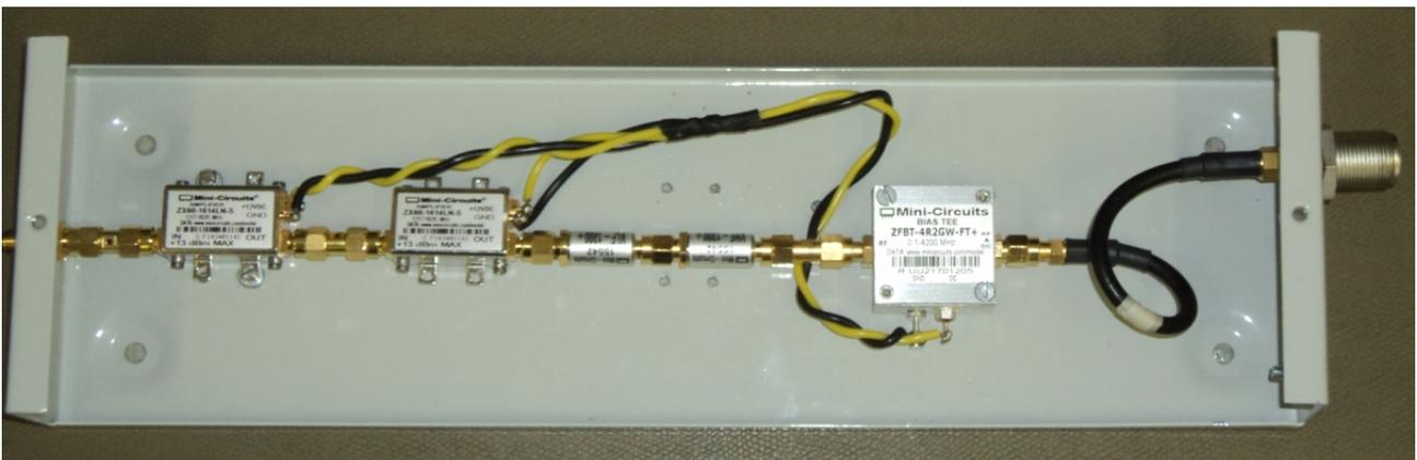
Figure E.3: Photo of the low-noise front-end units.
