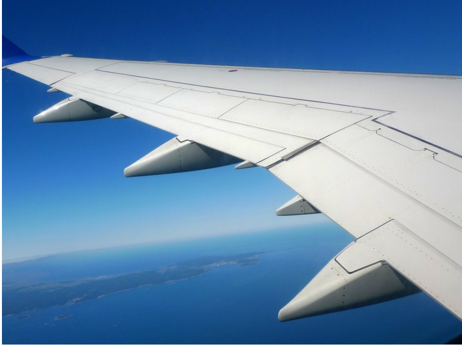
Figure 1.1 – Typical fairing protrusions on a wing of a conventional aircraft
