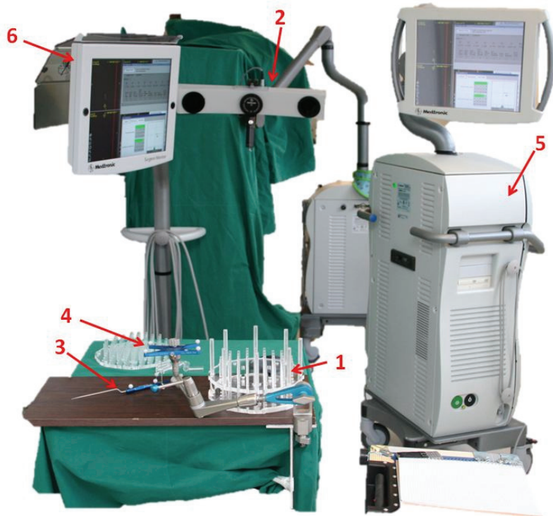
Fig. 17. The StealthStation Treon plus –navigator and the accuracy assessment setup with systems in place. (1) Accuracy assessment phantom, (2) Navigator’s optical camera, (3) Tracking instrument, (4) Patient tracker, (5) StealthStation Treon plus –navigator’s CPU, (6) Surgeon’s monitor.
