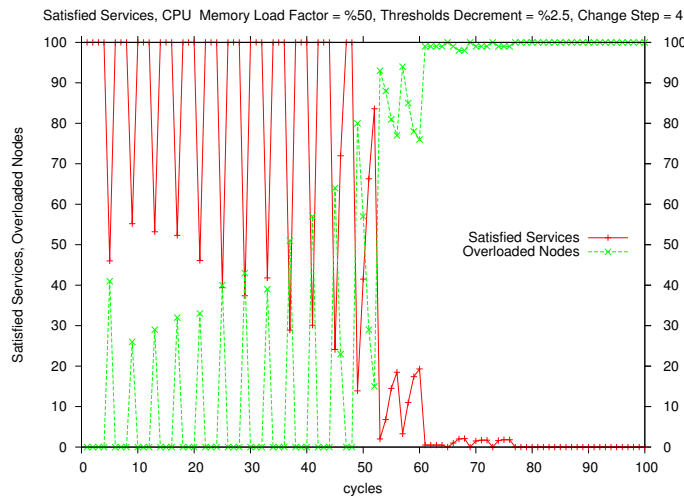
Figure 6.17. Satisfied services and overloaded nodes in case of decreasing node capacities. CPU and memory load factors are %50. Capacities are decremented by %2.5 every 4 cycles. Maximum number of replicas per service is R = 2 . We want to meet CPU and memory demands of services.
