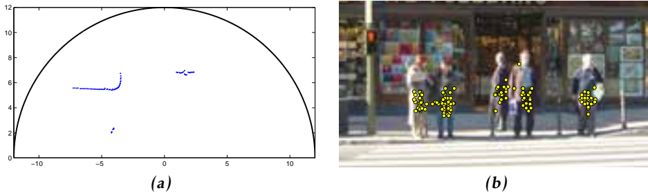
Figure 7.1: (a) Laser data with car, bicycle and pedestrian. (b) Camera image with pedestrian detections. Detections obtained using the classifier by Maji et al. (2008).
